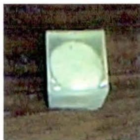
Figure 4.12 – Photograph showing a cake having been embedded in epoxy resin and squared off prior to sectioning
