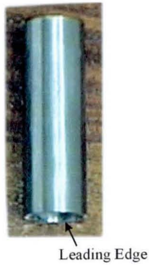
Figure 4.6 – Detail of the second sample tube, designed to be held in the apparatus used to temporarily set the cake prior to embedding in epoxy resin
