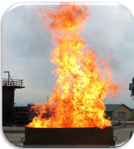
Figure 2.49: Clear flame of the ethanol pool fire. The unobscuration ratio for the ethanol fires was assumed to be 1
