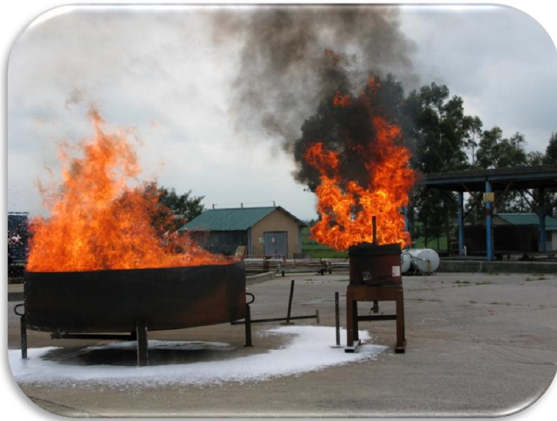
Figure 4.47: The gasoline ignited in the adjacent tank as a result of radiant heat flux. The adjacent small tank was uncovered and the liquid was evaporating
