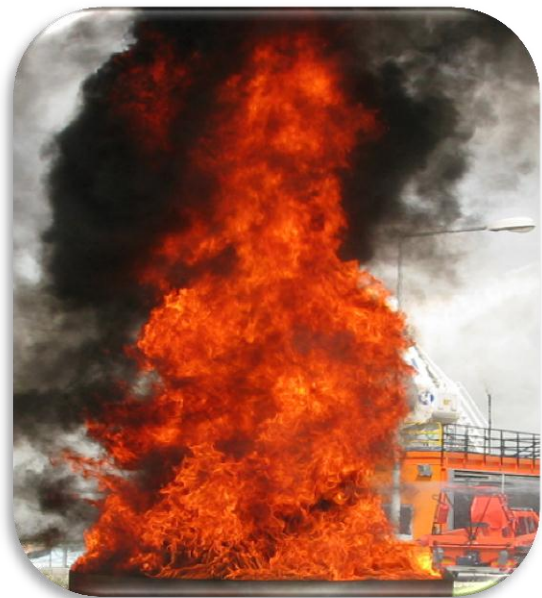
Figure 2.50 Smoky flame of the gasoline pool fire. The unobscuration ratio for the gasoline fires was assumed to be 0.9
