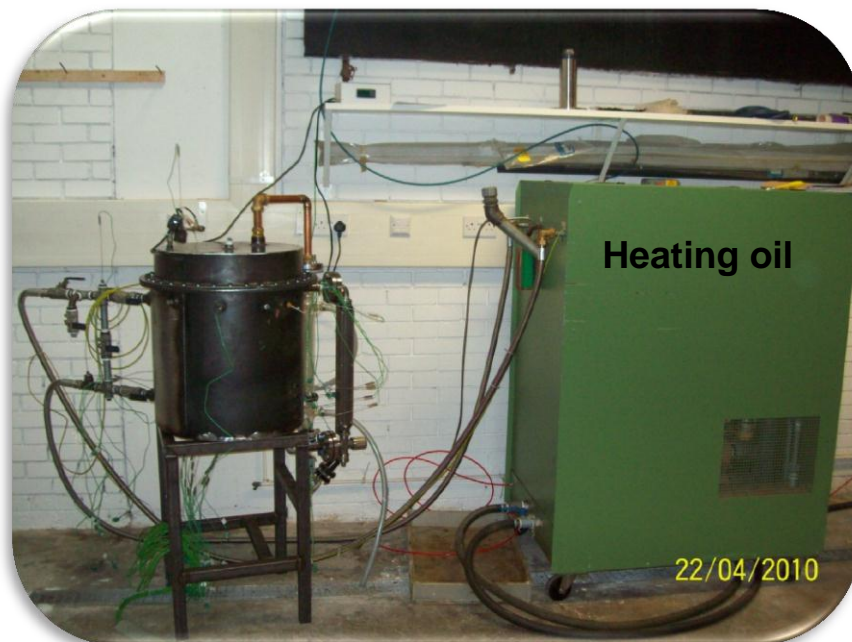
Figure 4.20: The heater heats the oil to the desired temperature and then pumps it to the vessel jacket. The vessel then receives cold oil, in a circulation heating process
