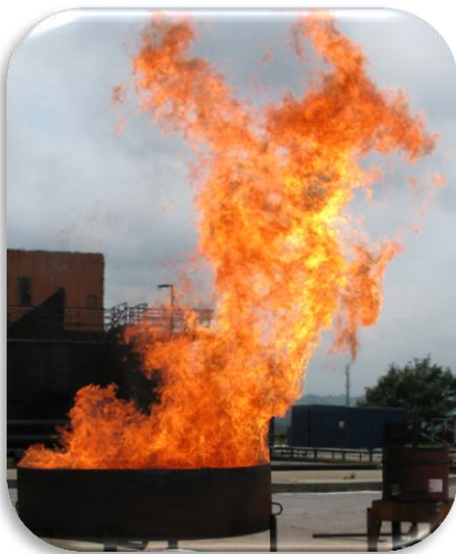
Flames from an experimental gasoline pool fire in Spain in 2010 – the wind-speed is 2 \text{ m. s}^{-1}
