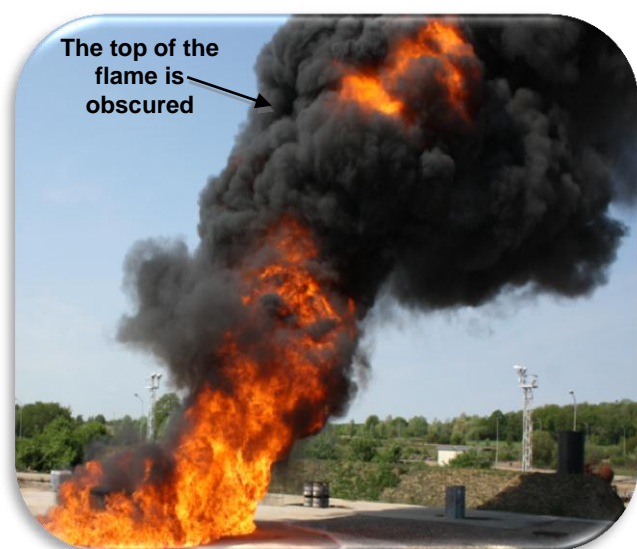
Figure 2.25: (10m) diameter gasoline pool fire showing that the flame is more obscured than in pools of a smaller diameter (LASTFIRE, 2011)
