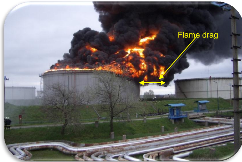
Figure 2.19: Flame drag, as observed in the LASTFIRE atmospheric gasoline storage tank fire test in Hungary
