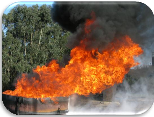
Flames from an experimental gasoline pool fire in Spain in 2010 – the wind-speed is 2 \text{ m. s}^{-1}
