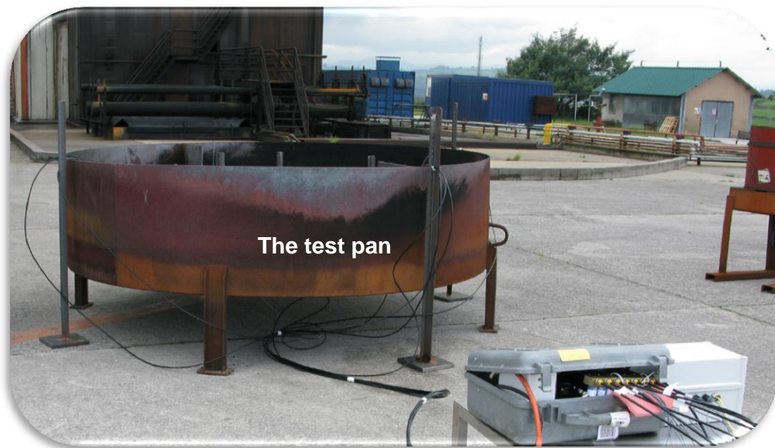
Figure 2.40: The pool fire test pan, with a diameter of 2.4 m. The rim of the pan stood approximately 1m above the ground
