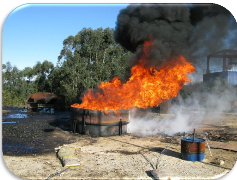
Figure 4.56: Shows the fire in the 2.4m test pan and the small tank, with regards to the pool fire. The flame is tilted, due to the effects of the wind, and the radiometer is positioned near the top of the small adjacent tank
