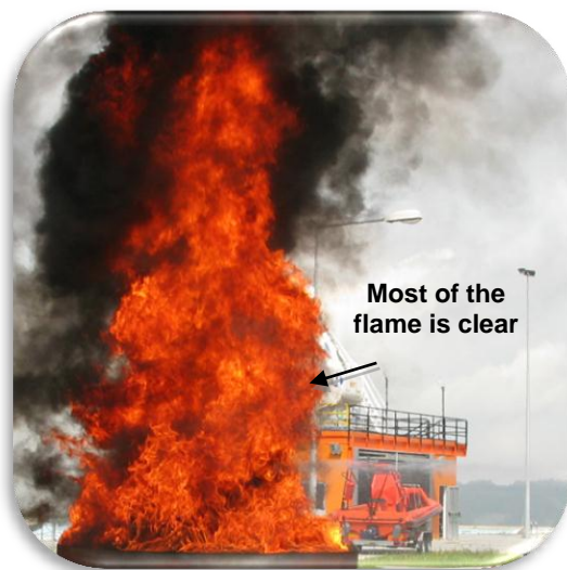
Figure 2.24: (2.4m) diameter gasoline pool fire showing that the flame is less obscured than in pools of a larger diameter (LASTFIRE, 2009)
