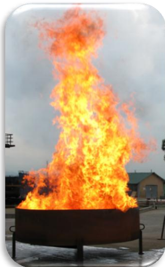
Flames from an experimental gasoline pool fire in Spain in 2009 – the wind-speed is 1 \text{ m. s}^{-1}
