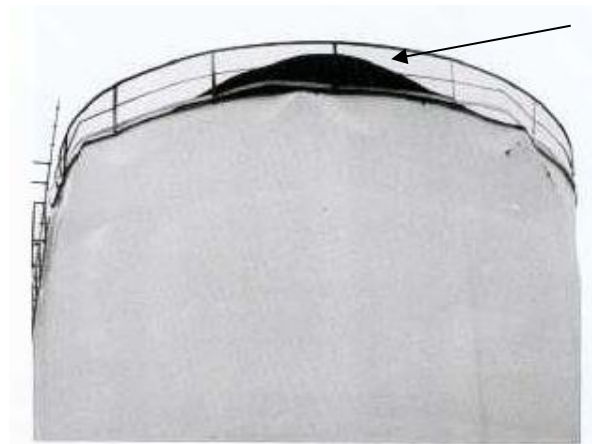
Figure 1.9: Fixed-roof tank with 'cod's mouth' failure, as it was subjected to internal pressure (www.mc-integ.co.uk, accessed March 2012)
