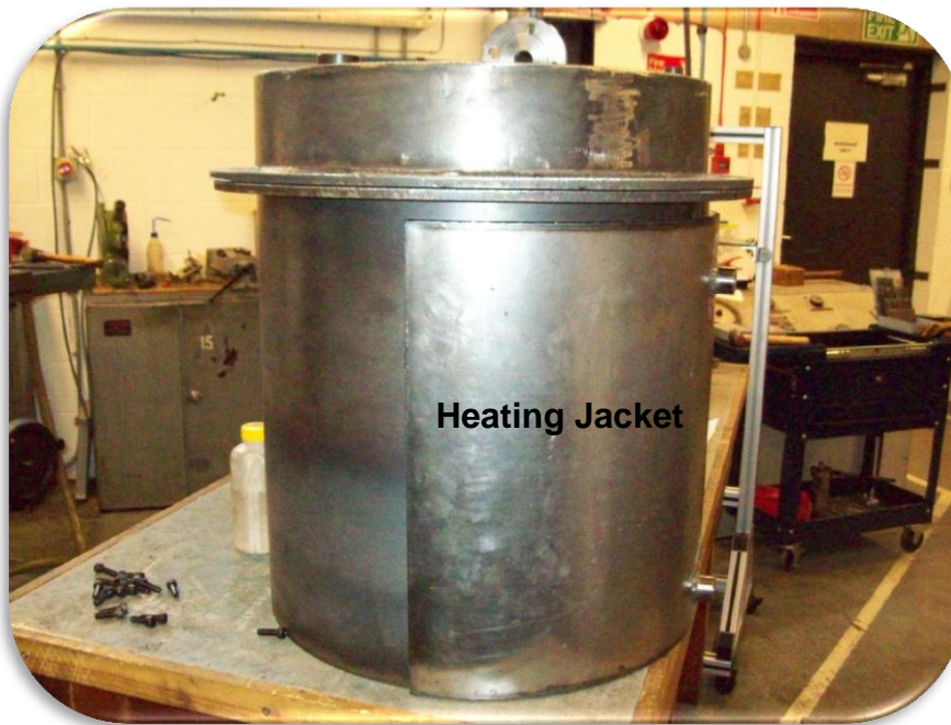
Figure 4.19: The heating oil jacket allows the heating oil to flow over and cover half the wall of the vessel
