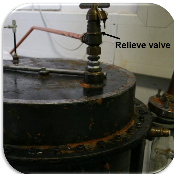
Figure 4.22: The experimental vessel was equipped with a pressure relief valve, in order to release the vapour at a certain set pressure
