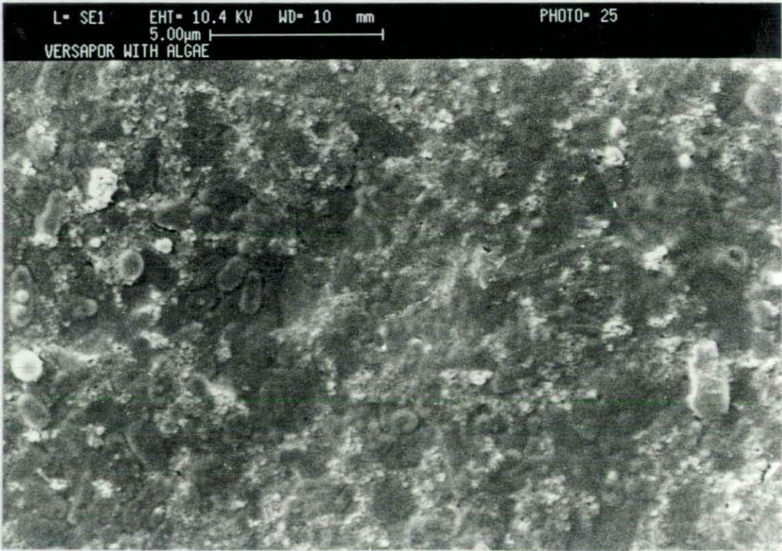
b) Clogged with algae and solids Fig 30 Polymer membrane
