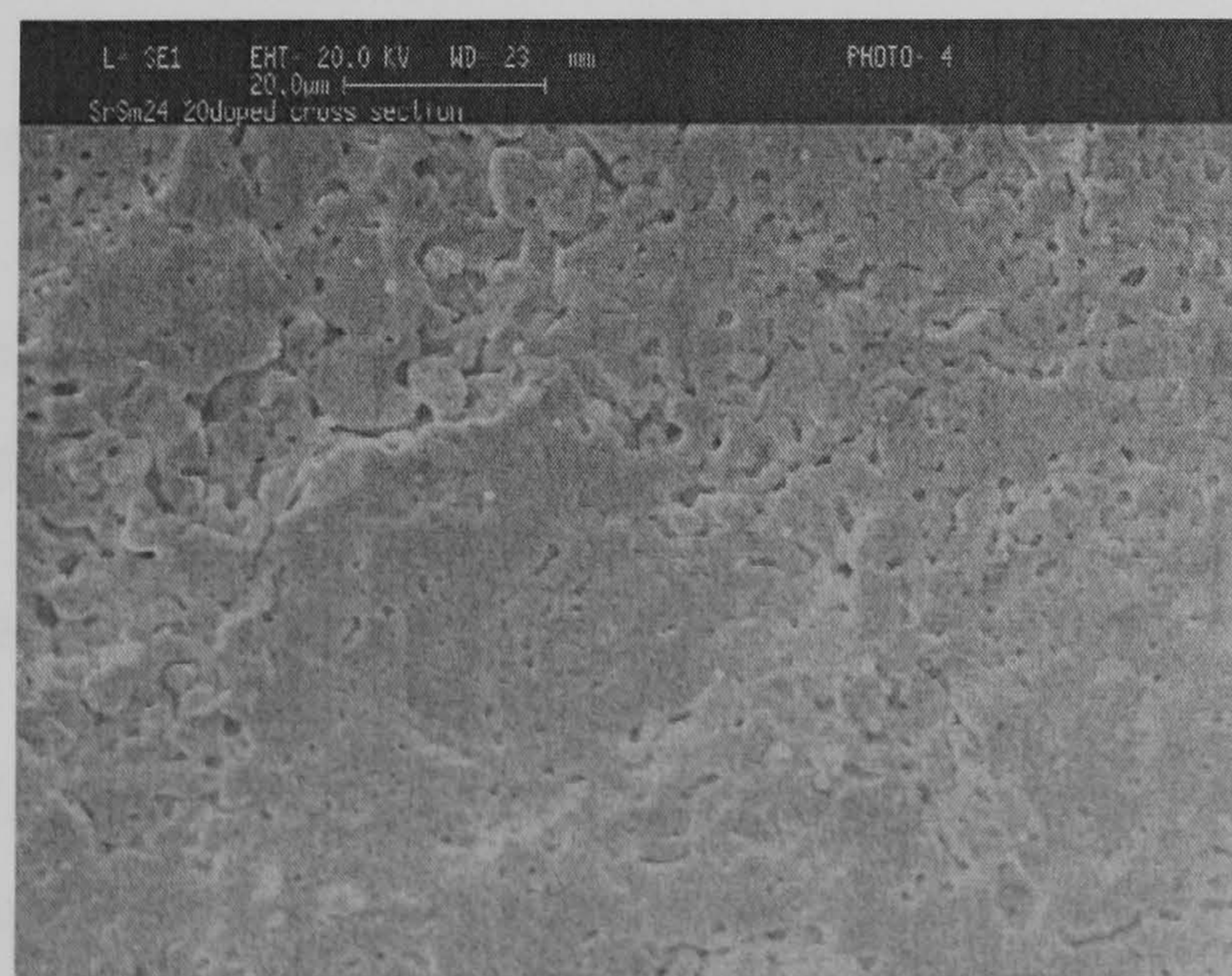
Figure 3-28. SEM image of cross section of samarium sulphide based pellet after EIS measurements
