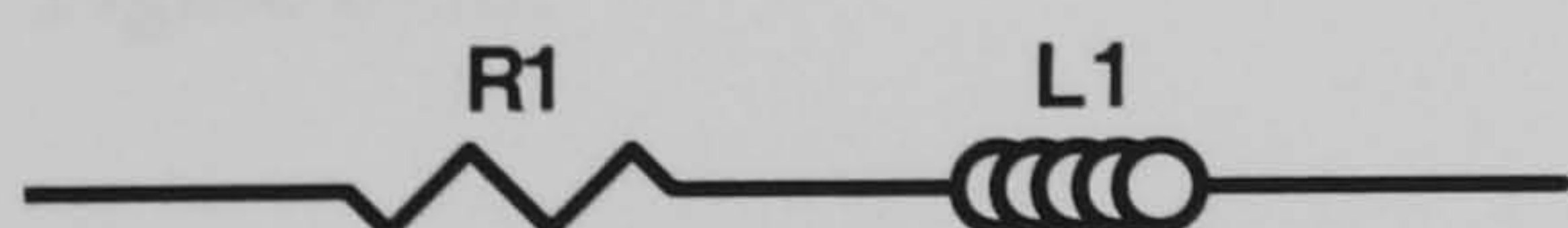
Figure 6-33. Proposed 'R-L' equivalent circuit for \text{BaBi}_2\text{S}_4
