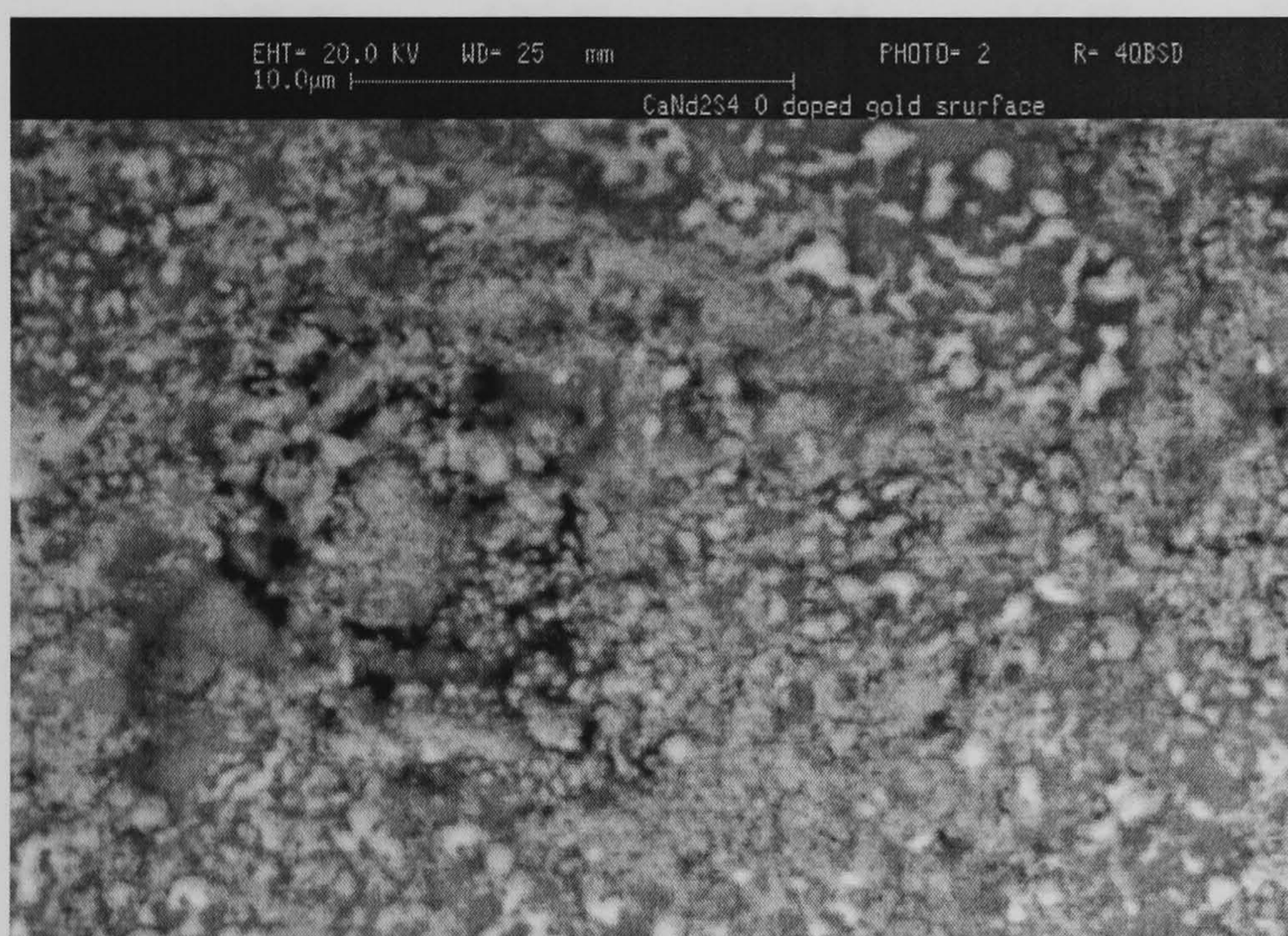
Figure 3-30. SEM image of gold electrode on undoped \text{CaNd}_2\text{S}_4 after EIS at 400°C in argon
