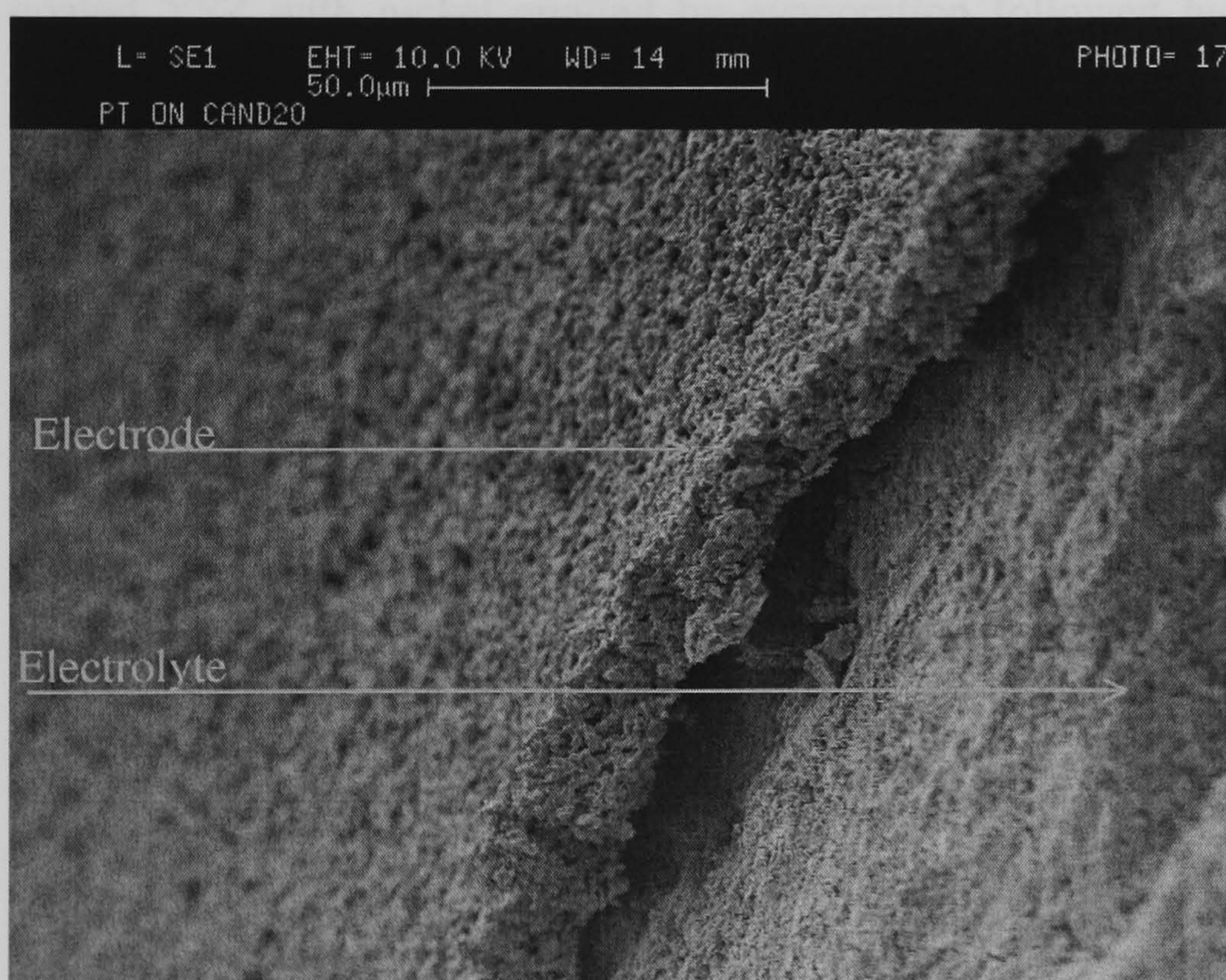
Figure 3-26. Pt electrode painted on \text{CaNd}_2\text{S}_4 , which has a porous structure similar to base material.
