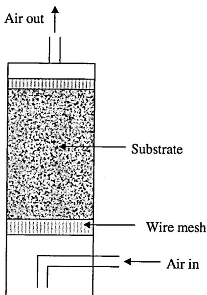
Figure 2.22 A Packed Bed Bioreactor (adapted from Robinson and Nigam, 2003).
