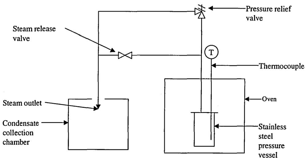
Figure 3.6. Steam Explosion Experimental Equipment.
