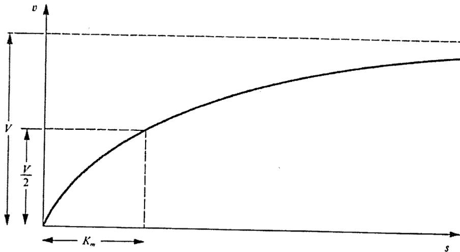
Figure 2.15 The Hyperbolic Relationship Between Initial Reaction Rate and Substrate Concentration of a Simple Catalysed Reaction (Yudkin and Offord, 1973).
