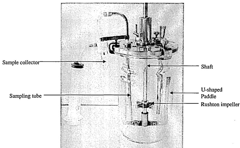
Figure 3.14. Glass Bioreactor.
