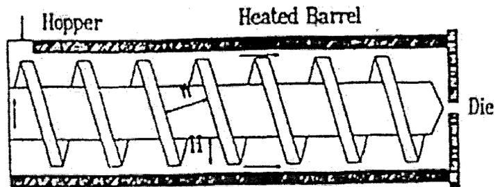
Figure 2.17 Diagram of a Single Screw Extruder (Jaluria and Wang, 1999).
