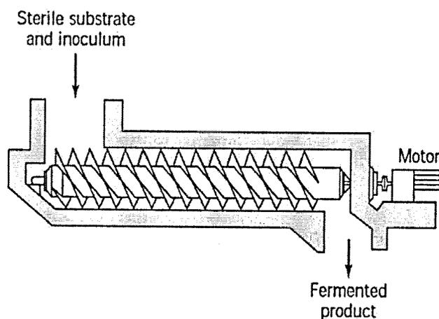
Figure 2.24 Continuous Screw Bioreactor (Chisti, 1999)
