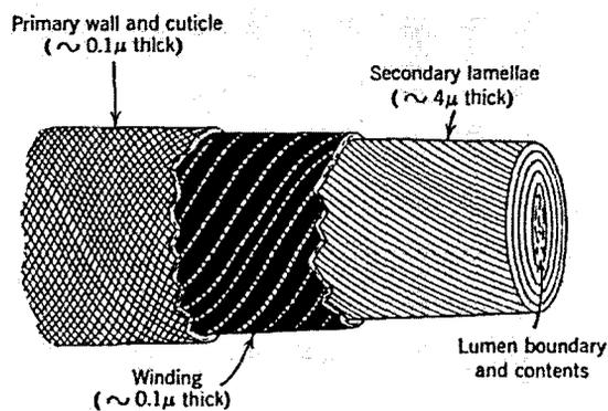
Figure 2.4 The Structure of Cotton Fibre (Immergut, 1963).
