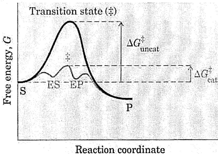
Figure 2.14 Reaction Coordinate Diagram Comparing Enzyme Catalysed and Uncatalysed Reactions (Lehninger, 1975).
