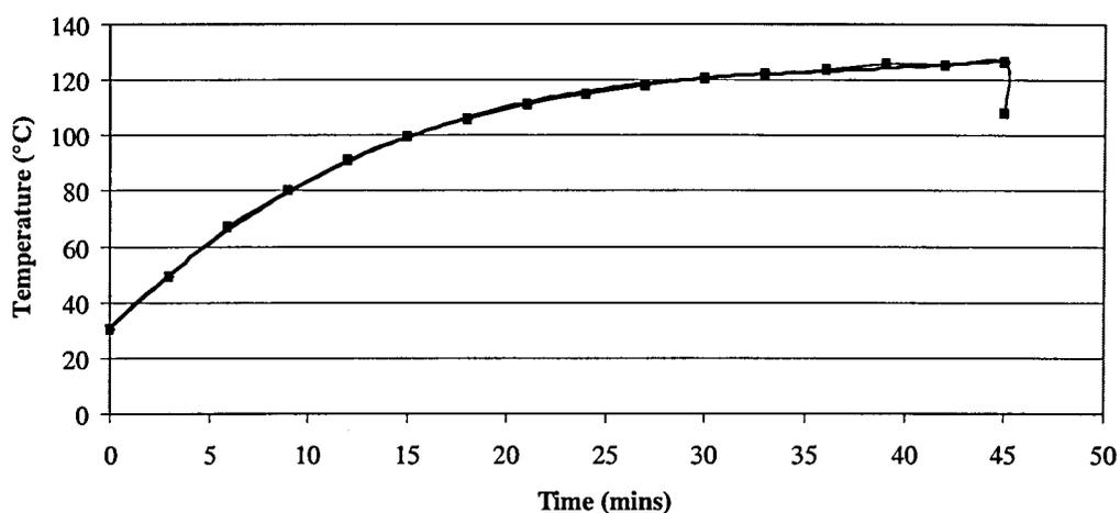
Steam Explosion Temperature Profile at an Oven Temperature of 130°C.
