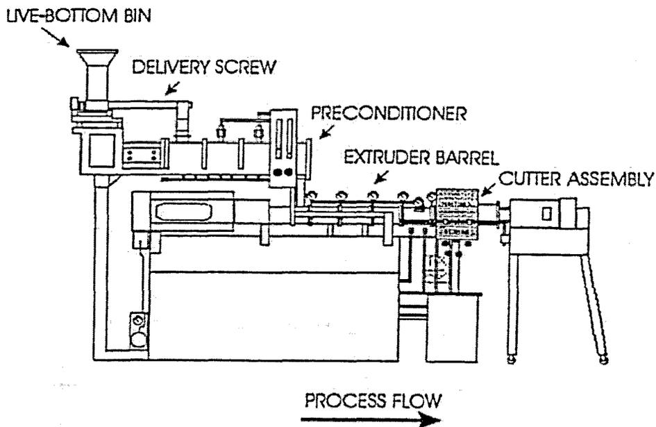
Figure 2.18 Flow Diagram of an Extruder (Brent, 1999).
