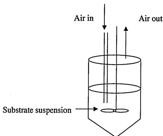
Figure 2.23 Agitated Batch Reactor.
