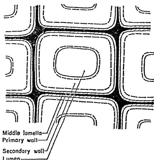
Figure 2.5 Cross Section of a Group of Wood Cells (Farmer, 1967).
