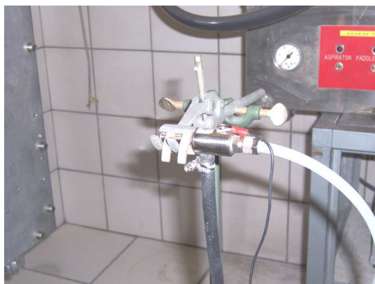
Figure 3.8: The feeding nozzle of Palas BEG-100 dust feeder.
