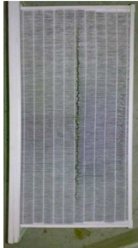
Figure 4.23: A fractured pleated media panel of minipleat filter used in an HVAC application in Kuwait.
