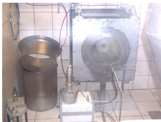
Figure 3.9: The feeding nozzle direction of the Palas BEG-100 dust feeder relative to the testing facility.
