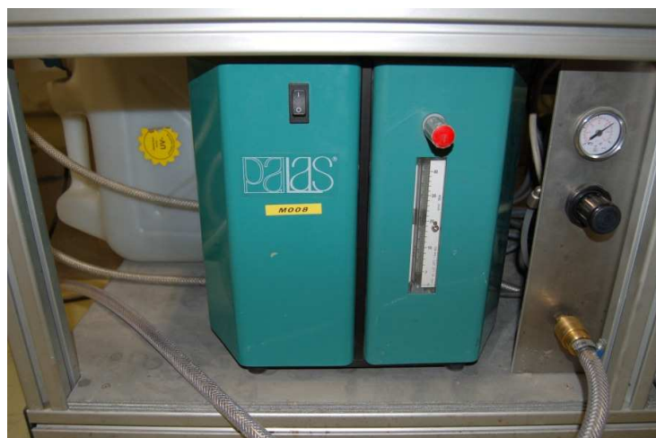
Figure 3.10: The PALAS aerosol generator used in the generation of DEHS.
