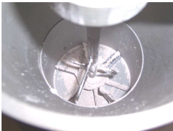
Figure 3.7: The powder reservoir towards the end of dust feeding.
