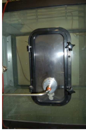
Figure 3.5: Access door and nozzles for efficiency measurement.
