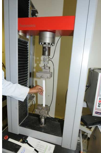
Figure 3.13: The universal testing machine used to measure the filter medium Young's modulus of elasticity (Testometric FS 150) at K.I.S.R. in Kuwait.
