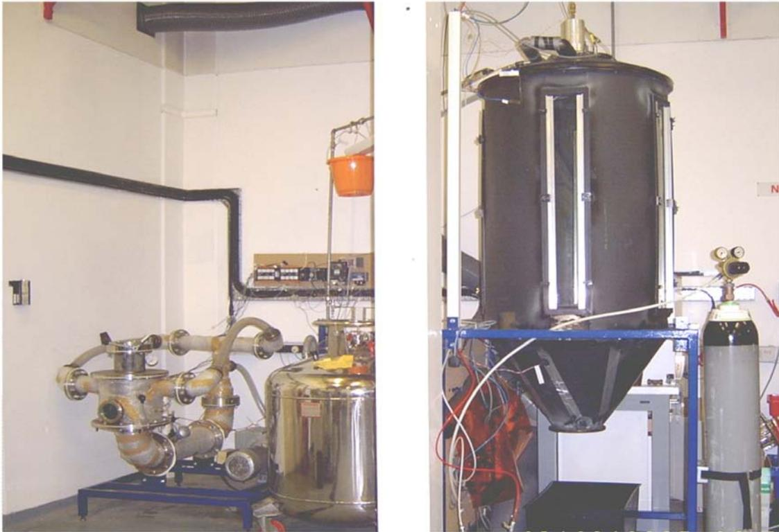
Figure 2. The spray-freeze-drying apparatus used at Loughborough. Spray-freezing initially occurs in the large (black) chamber located on the right of the photo. The spray frozen particles are collected from the base of this chamber and transferred to the sub-atmospheric fluidized bed freeze-drying apparatus on the left of the photo.
