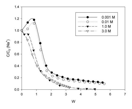
Figure 5: Variations of  $C/C_0$  (Na<sup>+</sup>) in the wash liquor with wash ratio (*W*) and ionic strength (10 mm cake, pH 7.4, 20 V,  $\Delta p_w = \Delta p_f = 100$  kPa).
