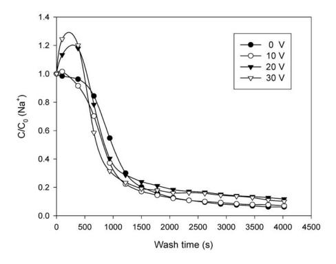
Figure 3: Variations of  $C/C_0$  (Na<sup>+</sup>) and in the wash liquor with time (t) and applied voltage (pH 7.8,  $10^{-3}$  M NaNO<sub>3</sub>,  $\Delta p_w = \Delta p_f = 400$  kPa). The area under the curve, which corresponds to the quantity of ions removed, is the time for each experiment. However, this can only be seen when a longer period if time is considered.
