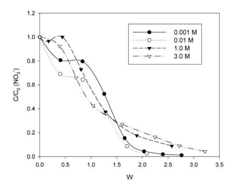
Figure 6: Variations of  $C/C_0$  (NO<sub>3</sub><sup>-</sup>) in the wash liquor with wash ratio (*W*) and ionic strength (10 mm cake, pH 7.4, 20 V,  $\Delta p_w = \Delta p_f = 100$  kPa).
