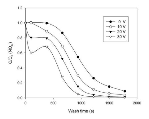
Figure 4: Variations of  $C/C_0$  (NO<sub>3</sub><sup>-</sup>) in the wash liquor with time (t) and applied voltage (pH 7.8,  $10^{-3}$  M NaNO<sub>3</sub>,  $\Delta p_w = \Delta p_f = 400$  kPa). The area under the curve, which corresponds to the quantity of ions removed, is the time for each experiment. However, this can only be seen when a longer period if time is considered.
