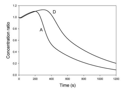
Figure 10: Concentration gradient as calculated by a numerical simulation for two sets of values for the velocity, ionic velocity for A is  $3x10^{-5}$  m s<sup>-1</sup> and  $2x10^{-5}$  for D.  $P^{(11)}$  and  $F^{(11)}$  are similar for both curves  $P^{(11)}/a = -0.003$  s<sup>-1</sup>,  $F^{(11)}/a = 0.002$  s<sup>-1</sup>.
