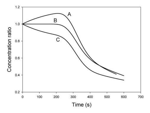
Figure 9: Concentration gradient as calculated by a numerical simulation for three sets of values for  $P^{(11)}$  and  $F^{(11)}$ ; A:  $P^{(11)}/a = -0.003 \, \text{s}^{-1}$ ,  $F^{(11)}/a = 0.002 \, \text{s}^{-1}$ ; B:  $P^{(11)}/a = -0.003 \, \text{s}^{-1}$ ,  $F^{(11)}/a = 0.003 \, \text{s}^{-1}$ .
