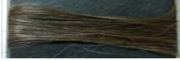
Fig. 31: Example of hair tress – support for contact angle measurements.
