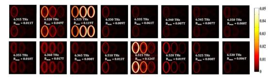
**Figure 3.** Switching over a range of 6.315 to 6.530 *THz* in a transverse electric field. The colour bar indicates the strength of the resulting magnetic flux density (limited to 0.05 T for greater visual clarity), which is much higher around the edges of the disks than at the locations of the  $\pi$ -rings. Whispering gallery modes of varying intensities appear around the elliptical disks as a function of frequency. The maximum field,  $B_{max}$  is indicated for each frequency.
