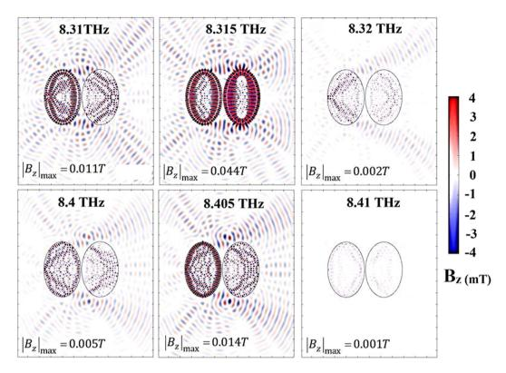
Figure 2. The electromagnetic field is focused at the centre of the left hand edge of the left elliptical disk, which contains a subwavelength sized notch. The propagation of the electric field can create a frequency dependent pumping of the system between whispering galleries. The maximum magnetic flux density in the *z*-direction is shown below the disks in each plot for the corresponding frequencies (shown above).
