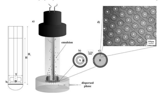
Figure 1. a) Schematic diagram showing a Micropore dispersion cell. b) Schematic view of the ring membrane. c) Schematic view of the whole membrane (region A indicates pores closed off, region B indicates open pores, and region C indicates the position where the gasket surrounding the membrane inside the stirred cell sits). d) Micrograph of a portion of membrane surface.
