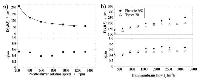
Figure 2. a) Effect of the stirrer rotational speed on the median droplet diameter and the span of the particle size distribution (whole 20- $\mu$ m membrane, continuous phase: 2% Tween 20,  $J_d=320$  lm<sup>-2</sup>h<sup>-1</sup>. b) Effect of the transmembrane flux on the mean particle diameter and the span of the particle size distribution (ring 20- $\mu$ m membrane at 596 rpm).
