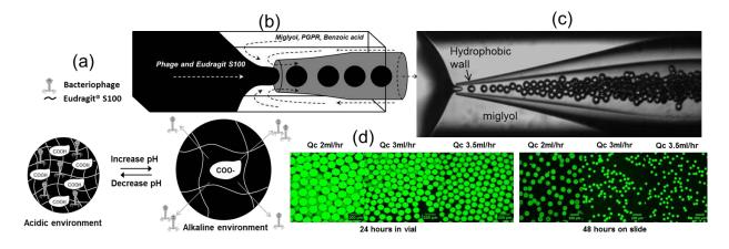
**Figure 1.** a) Schematic to show the polymer release mechanism; b) schematic of the glass capillary microfluidic device for particle generation; c) screen shot of droplet formation; d) SEM of phage encapsulated particles.
