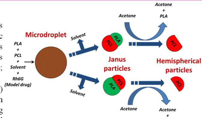
Figure 1. Bi-polymer Janus particles and hemispherical particle production.
