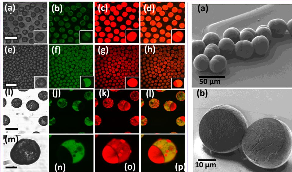
Figure 4. Confocal microscopic images of dyed polymer microspheres showing different PLA (Green) to PCL (Ratio) after phase. Scale bars: (a-d): 50  $\mu\text{m}$ ; (e-h): 50  $\mu\text{m}$ ; (i-l): 100  $\mu\text{m}$  and (m-p): 50  $\mu\text{m}$
