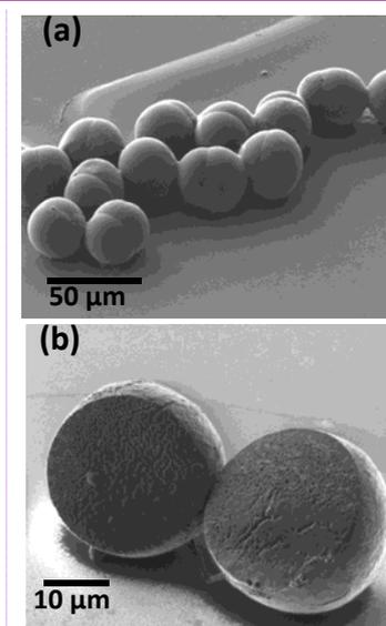
Figure 5. FIB images of (a) Janus particles with 1:2 (PLA:PCL) volume ratios. (b) PCL Hemispherical Microparticles.
