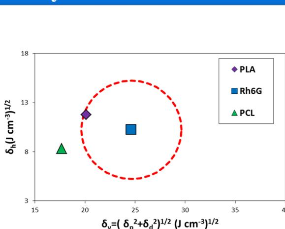
Figure 3. Bagley's two-dimensional graphs of partial solubility parameters. PLA in the solubility circle signifies Rh6G's higher preference for PLA than PCL.
