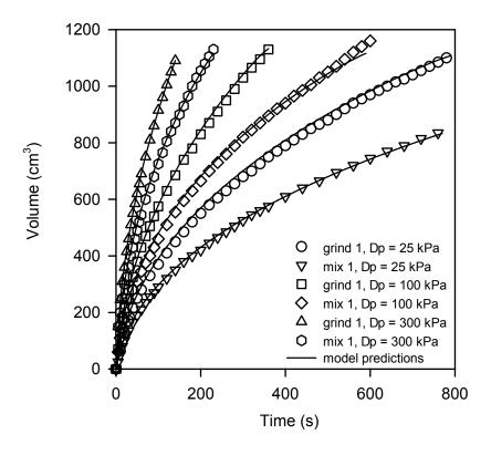
Figure 5: The effects of particle size distribution on filtration performance.
