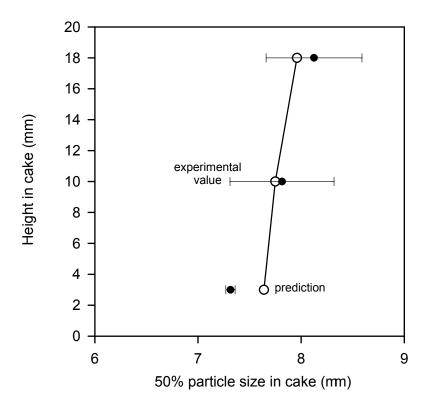
Figure 7: Experimental and theoretical particle sizes in a filter cake; grind 1,  $\Delta p$  = 100 kPa.
