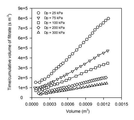
Figure 3: Sequential variation of experimental data with filtration pressure; grind 1.
