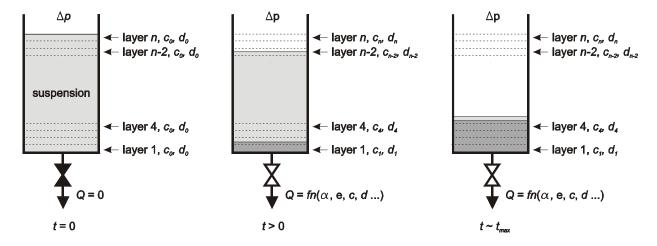
Figure 4: Schematic of the model for filtration with simultaneous sedimentation.
