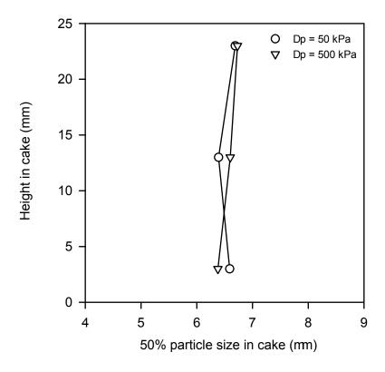
Figure 9: The effects of filtration pressure on the measured particle size in a filter cake; grind 3.
