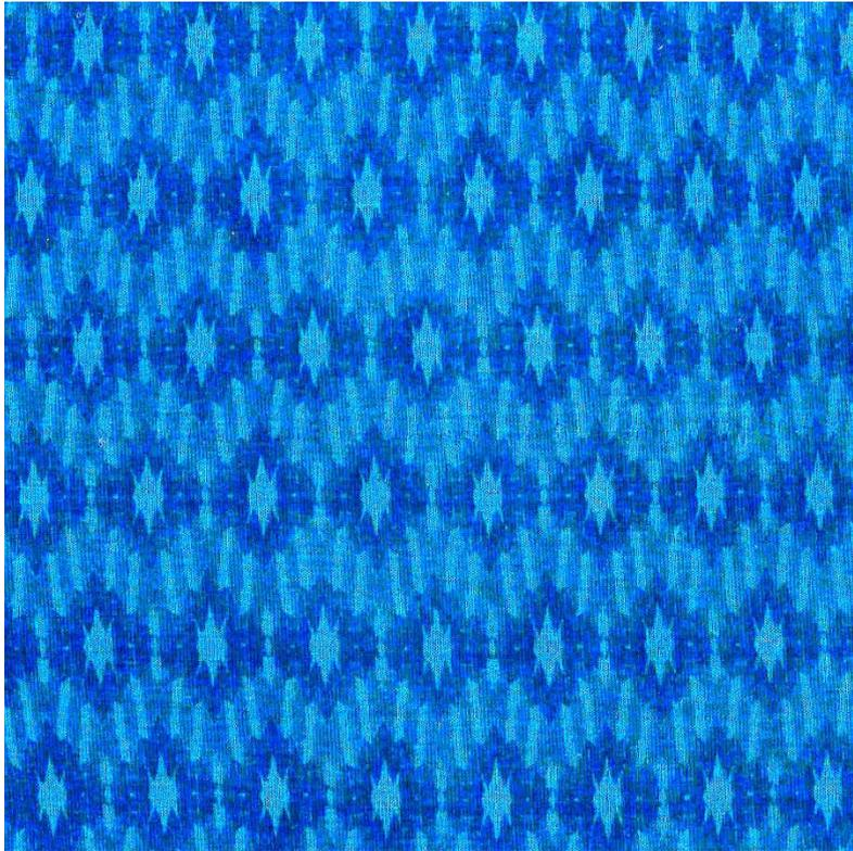
Figure 139: Laser-dyed knitted polyester textile sample: greyscale method
