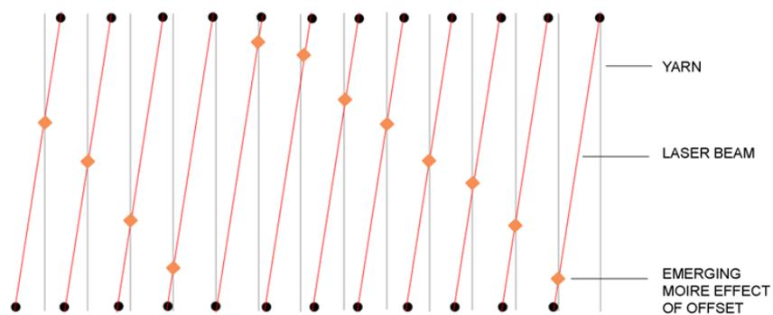
Figure 80: Diagram demonstrating emerging moiré effect
