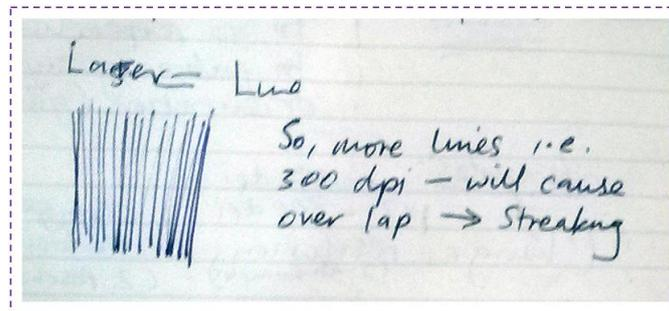
Figure 61: Log book note: Laser beam scanning causing beam overlap leading to a 'streaking' effect
