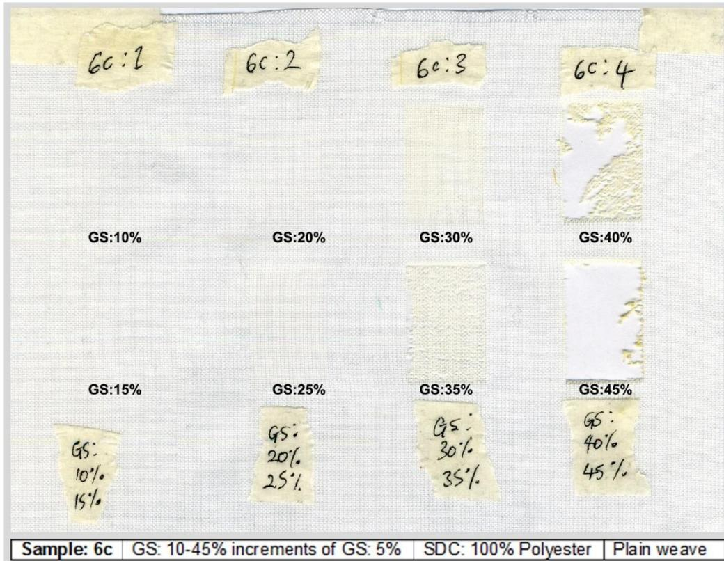
Figure 54: Laser treated ISO woven polyester with a reduced range of 8 greys
