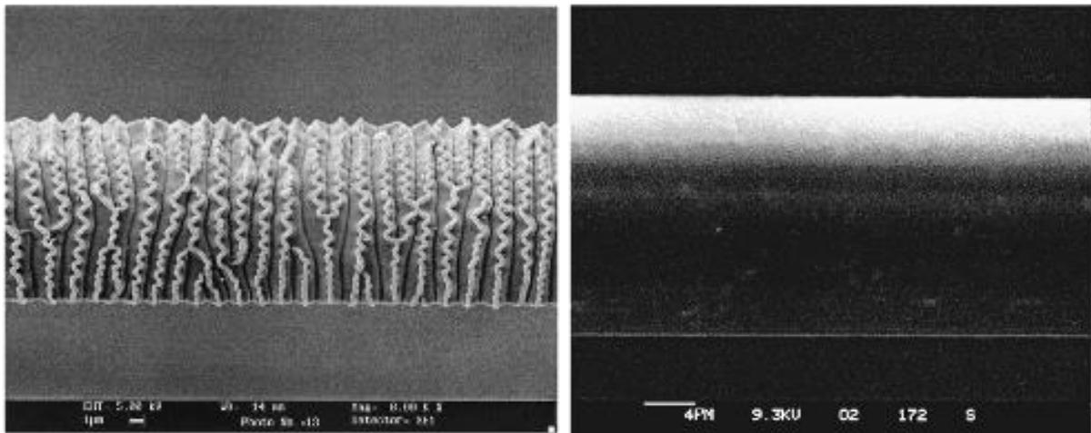
Figure 14: (Left) Surface structure of laser treated polyester under high fluence (Kan 2008b, p.115)
