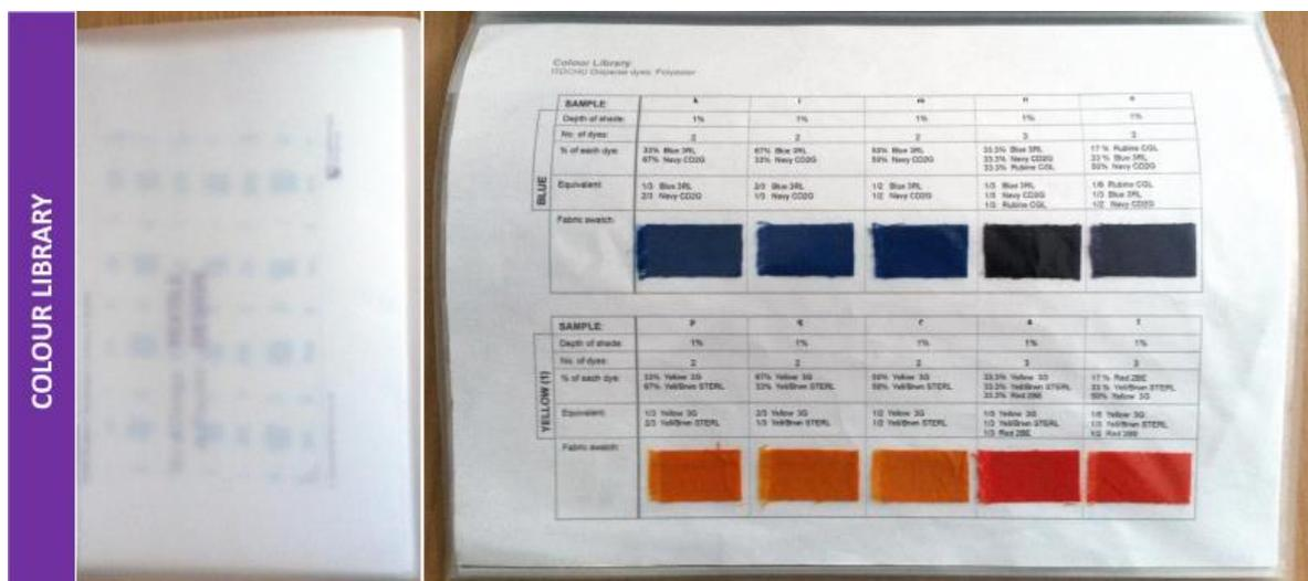
Figure 44: Colour Library with precision dyed PET fabric swatches
