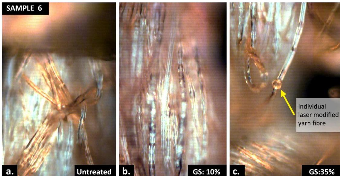
Figure 55: Laser treated SDC polyester treated sample 6 viewed at x20 magnification
