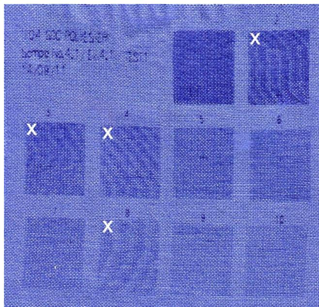
Figure 78: Examples of moiré surface effects generated in this research with woven PET
