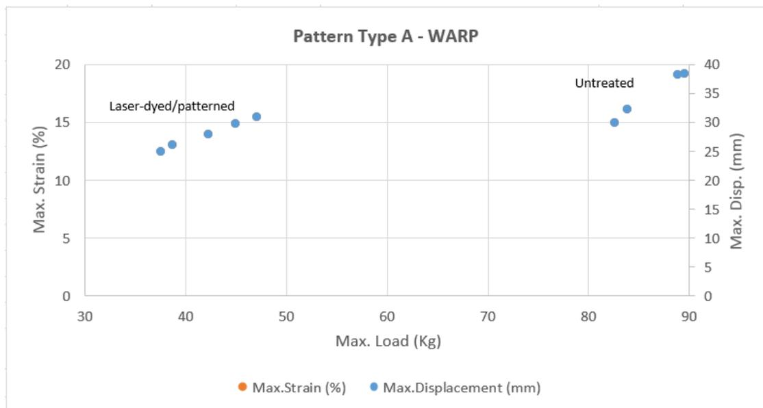
Figure 124: Tensile Strength results graph: WARP - Pattern Type A and Untreated fabric
