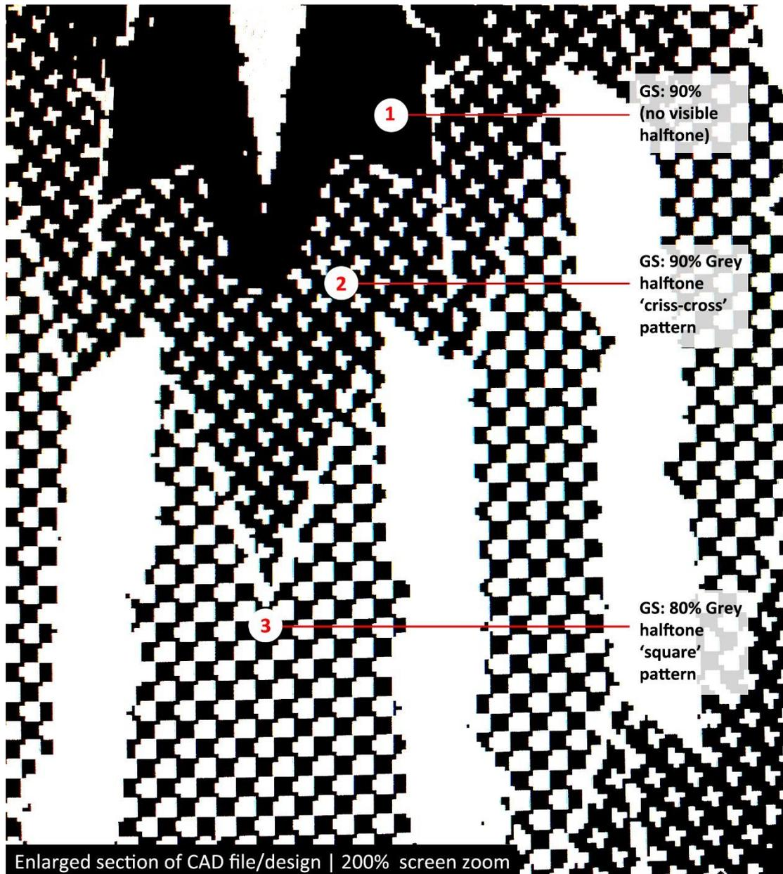
Figure 68: Halftone reduction CAD file - pixelated grids based on different GS% in a pattern/design
