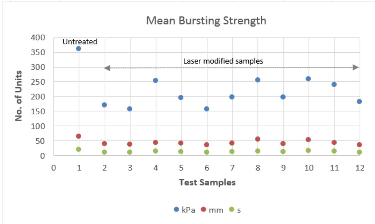
Figure 134: Bursting strength results graph
