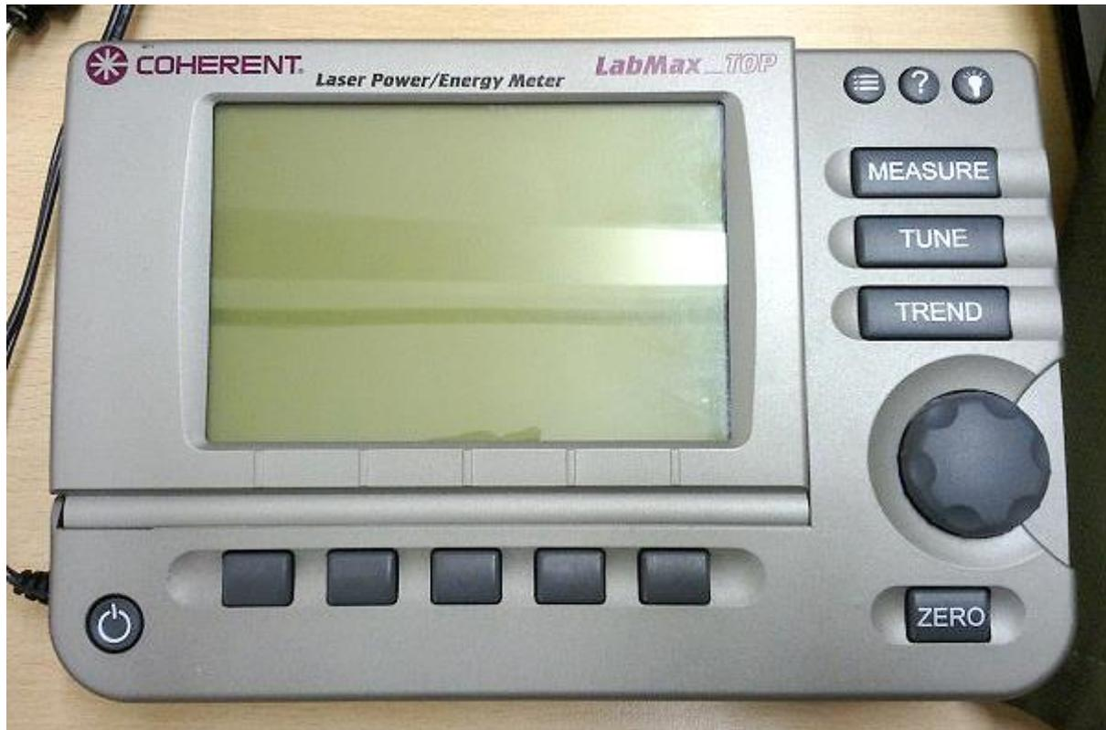
Figure 43: Digital laser power meter – 0-10W Coherent LM10 Probe
