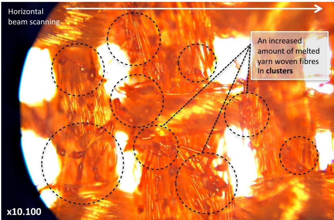
Figure 69: Horizontal beam scanning showing increased fibre damage with woven PET sample
