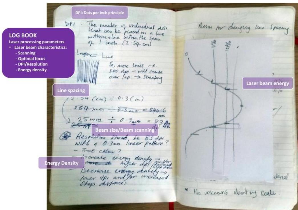
Figure 37: Log book: Problem solving in relation to beam behaviour and laser scanning
