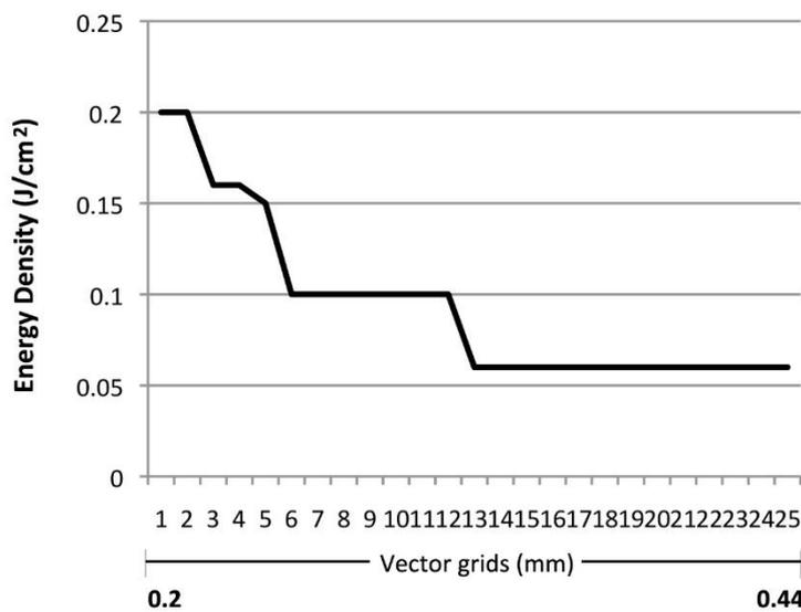
Figure 92: Diagram showing an energy density decline as line spacing increases per vector grid
