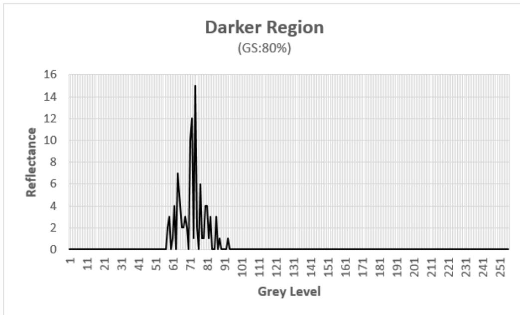
Figure 114: Grey Level Histogram of fabric sample: Darker Region (GS: 80%)
