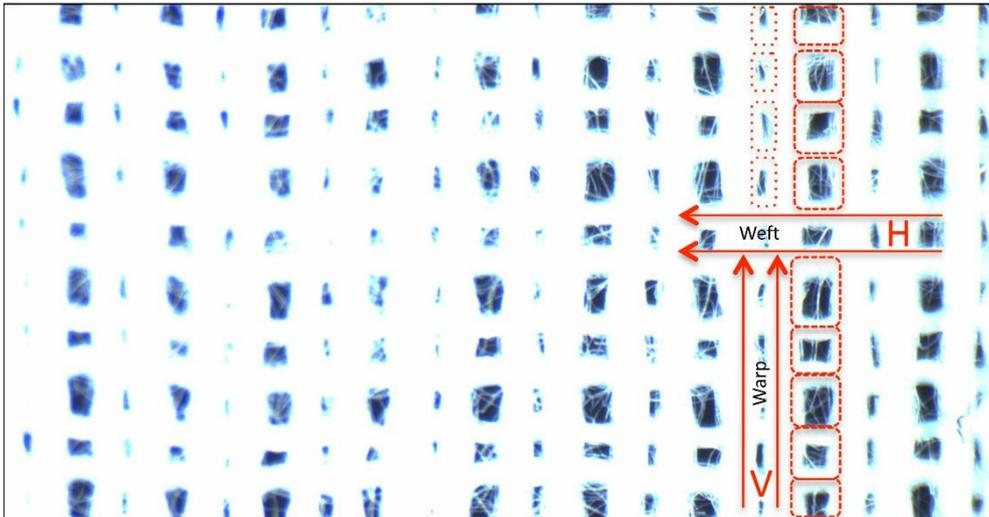
Figure 71: Woven PET fabric structure showing spacing of warp yarns and weft yarns (x5 mag.)
