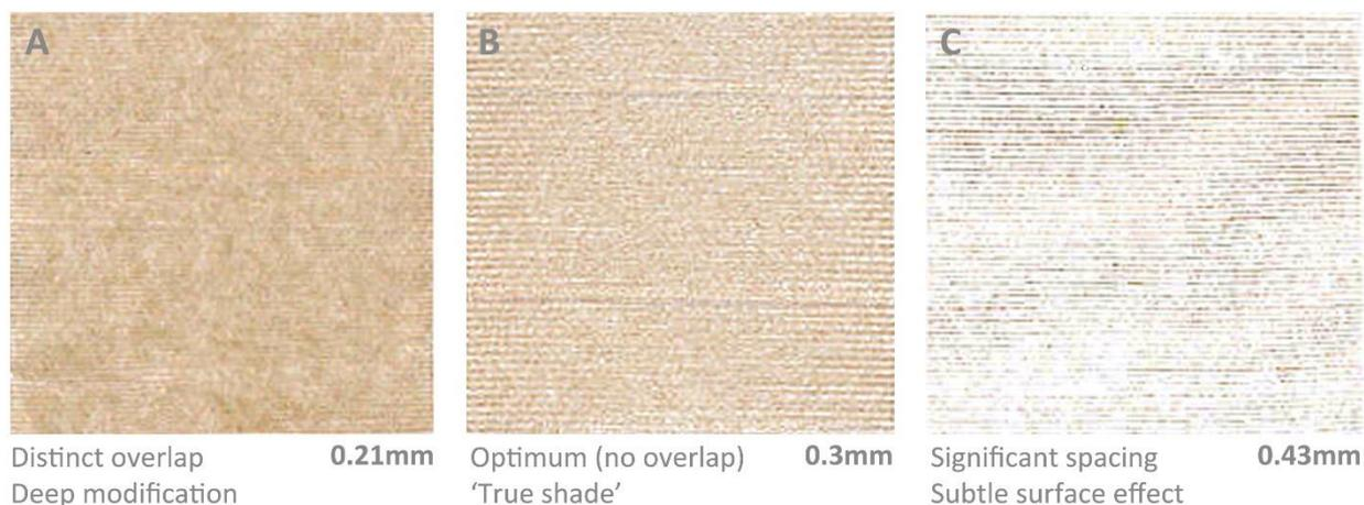
Figure 88: Laser marked vector grids on paper
