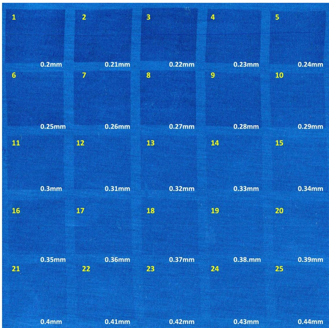
Figure 87: Laser-dyed tonal colour chart: knitted polyester fabric sample
