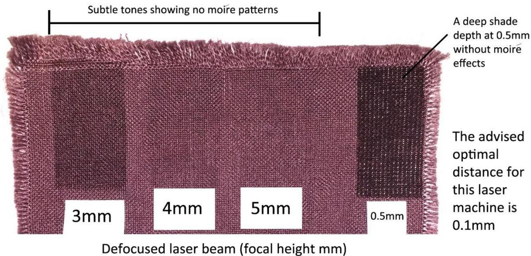
Figure 81: Defocusing the laser beam with woven PET to eliminate moiré effects (laser bed system)
