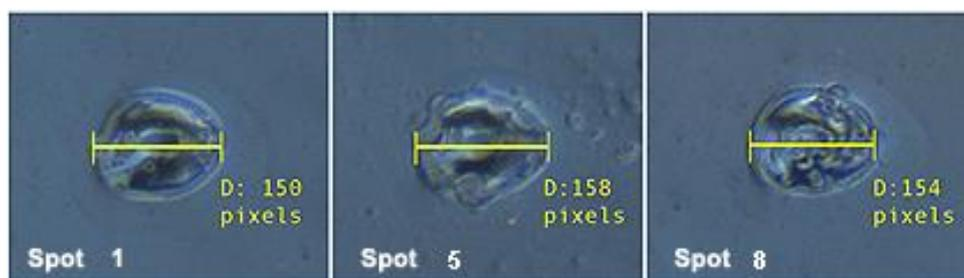
d. Micrographs of acrylic burn print (x10.100) showing the number of pixels/diameter per spot
