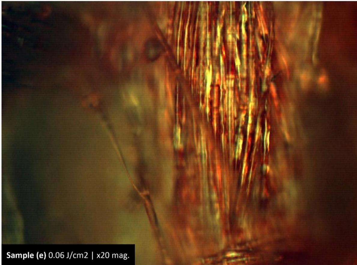
Figure 154: Sample (e): showing sufficient coloration without significant damage when processed with 0.06 J/cm<sup>2</sup> energy density.
