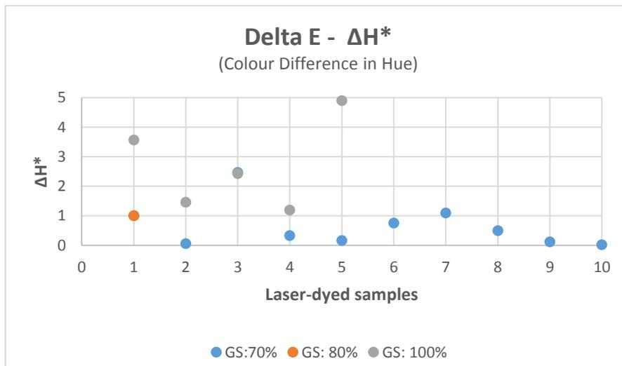
Figure 108: Delta E Colour difference: Hue results ( $\Delta H^*$ )
