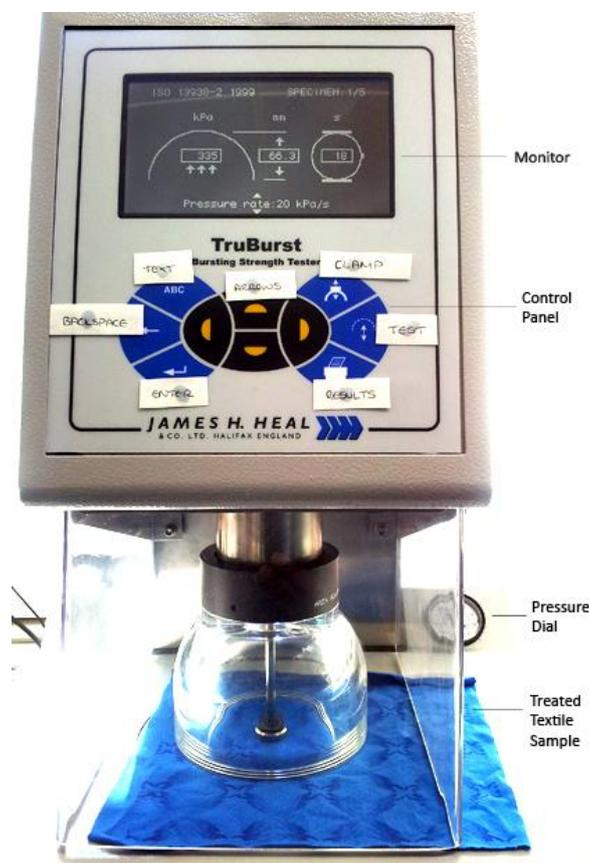
Figure 132: Bursting Strength Tester Machine
