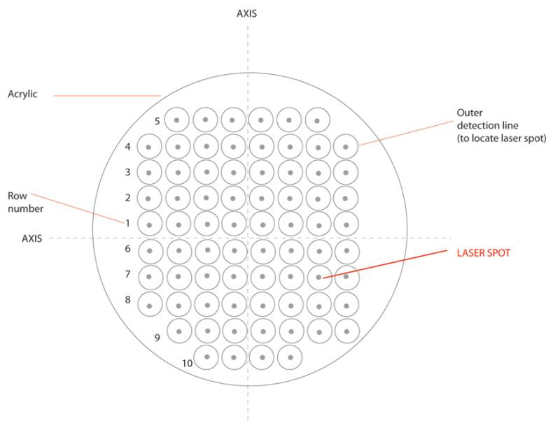
a. Burn print orientation: example showing layout of laser spots
