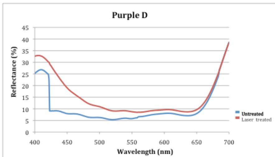
Figure 100: Reflectance/Batch 4: Purple - Laser treated and untreated fabrics: GS: 70% (*Purple D*)
