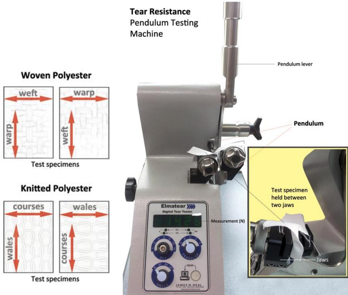
Figure 128: Tear Resistance specimens - woven and knitted polyester fabrics (Left)
