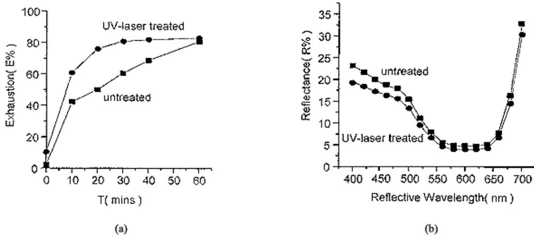
Figure 18 (Left): Exhaustion rate of laser treated and untreated dyed polyester samples (Lau et al. 1997, p. 526)
