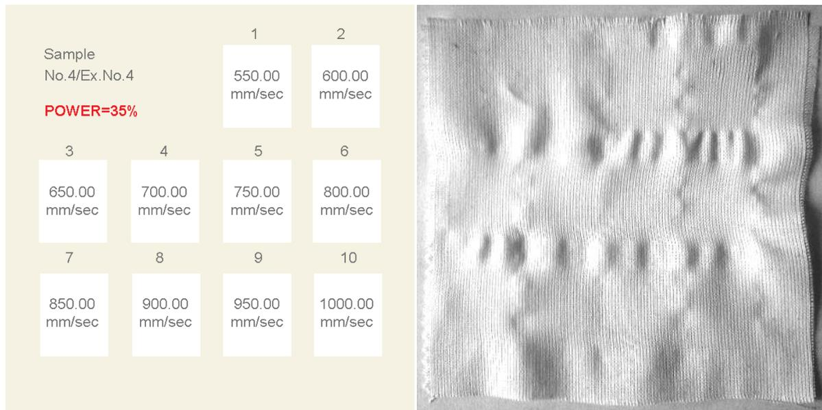
Figure 40: Configuration of laser parameters explored using the CO2 10W Synrad laser marker (left); and the resulting woven polyester woven fabric sample (right)
