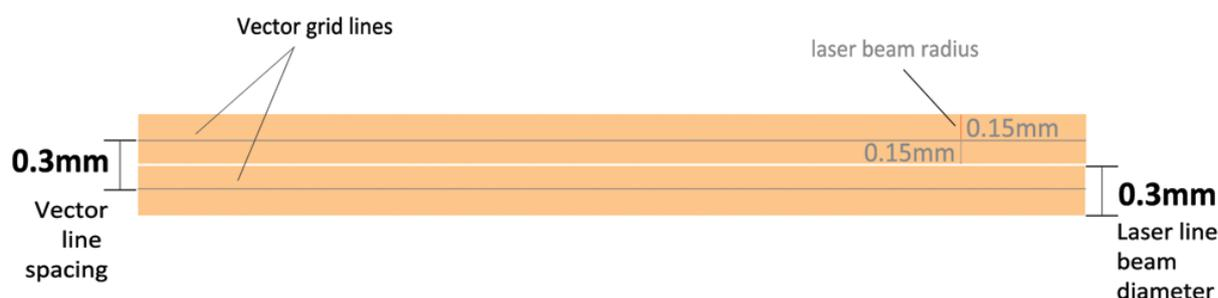
Figure 89: Diagram showing the position of a 0.3mm laser line vector grid
