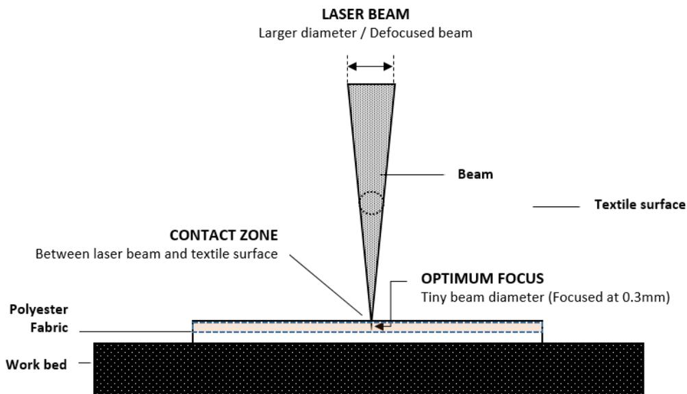
Figure 36: Fibre-laser interaction
