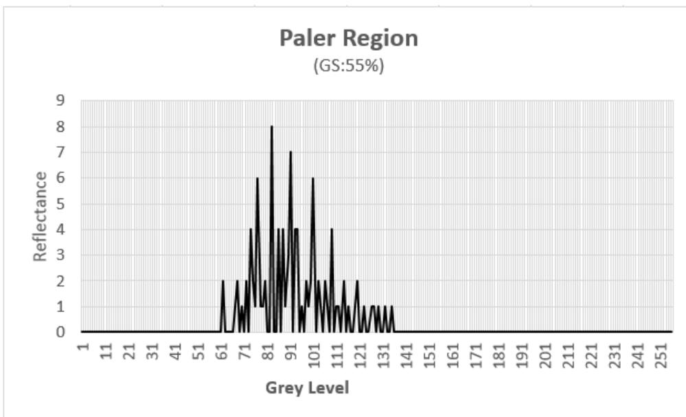
Figure 113: Grey Level Histogram of fabric sample: Paler Region (GS: 55%)
