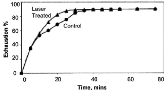
Figure 22: Exhaustion rate in acid bath – laser treated and control PA fabric samples (Shahidi et al. 2013, p.43)
