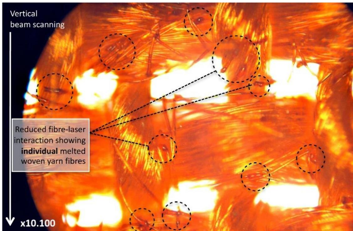
Figure 70: Vertical beam scanning showing reduced fibre damage with woven PET sample
