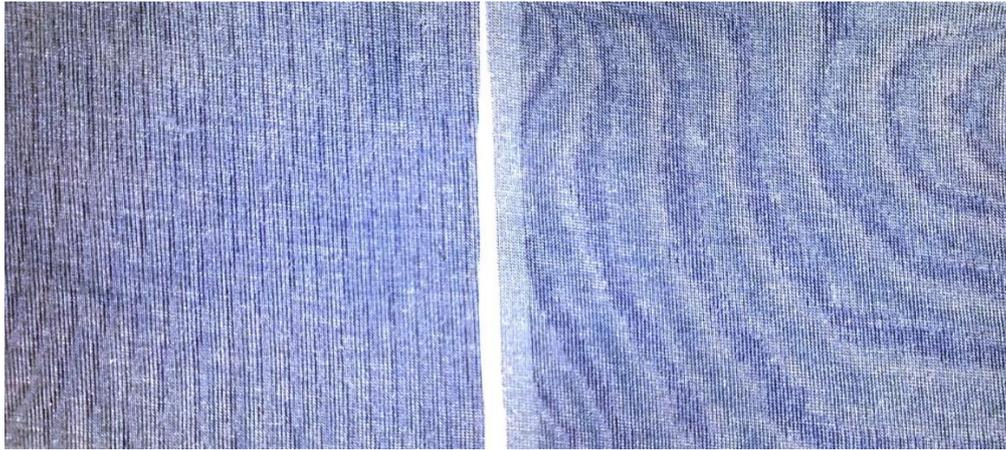
Figure 82: Moiré pattern on knitted PET textile surface
