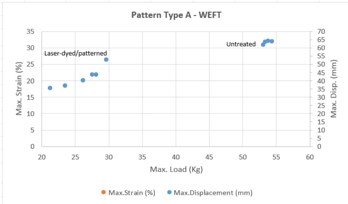
Figure 125: Tensile Strength results graph: WEFT - Pattern Type A and Untreated fabric
