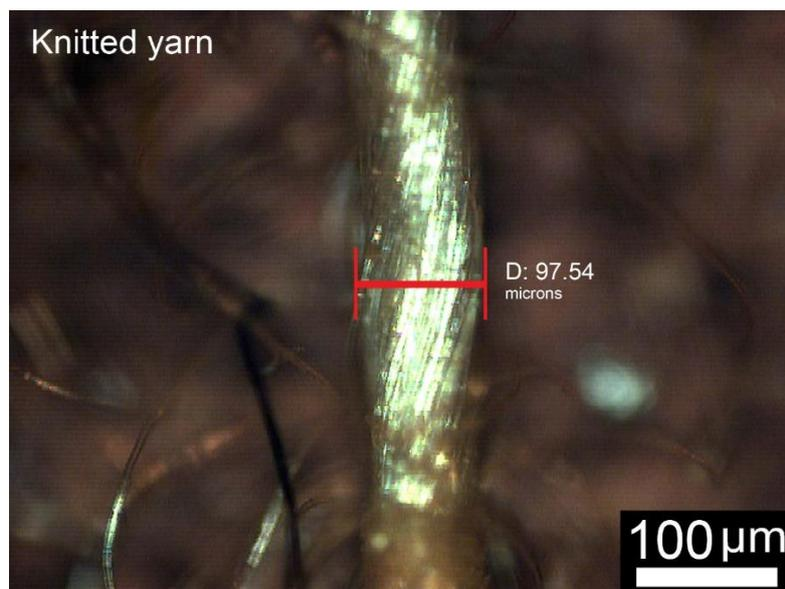
Figure 83: Micrograph of individual yarn taken from knitted PET fabric (x10.100 magnification)
