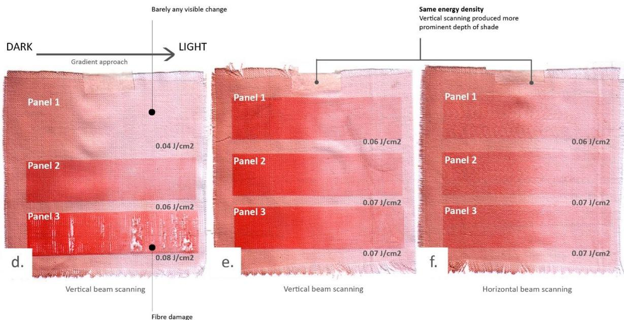
Figure 152: Gradient samples: laser modified panels with different energy densities
