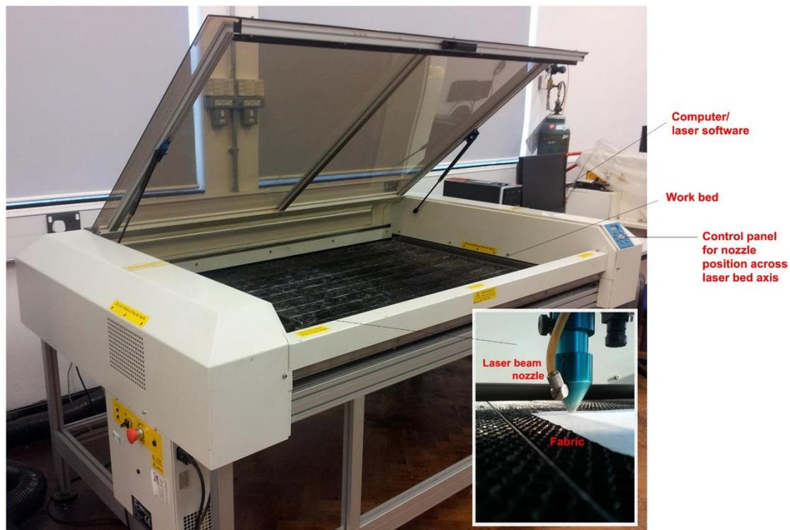
Figure 47: 58W CO<sub>2</sub> Laser bed system
