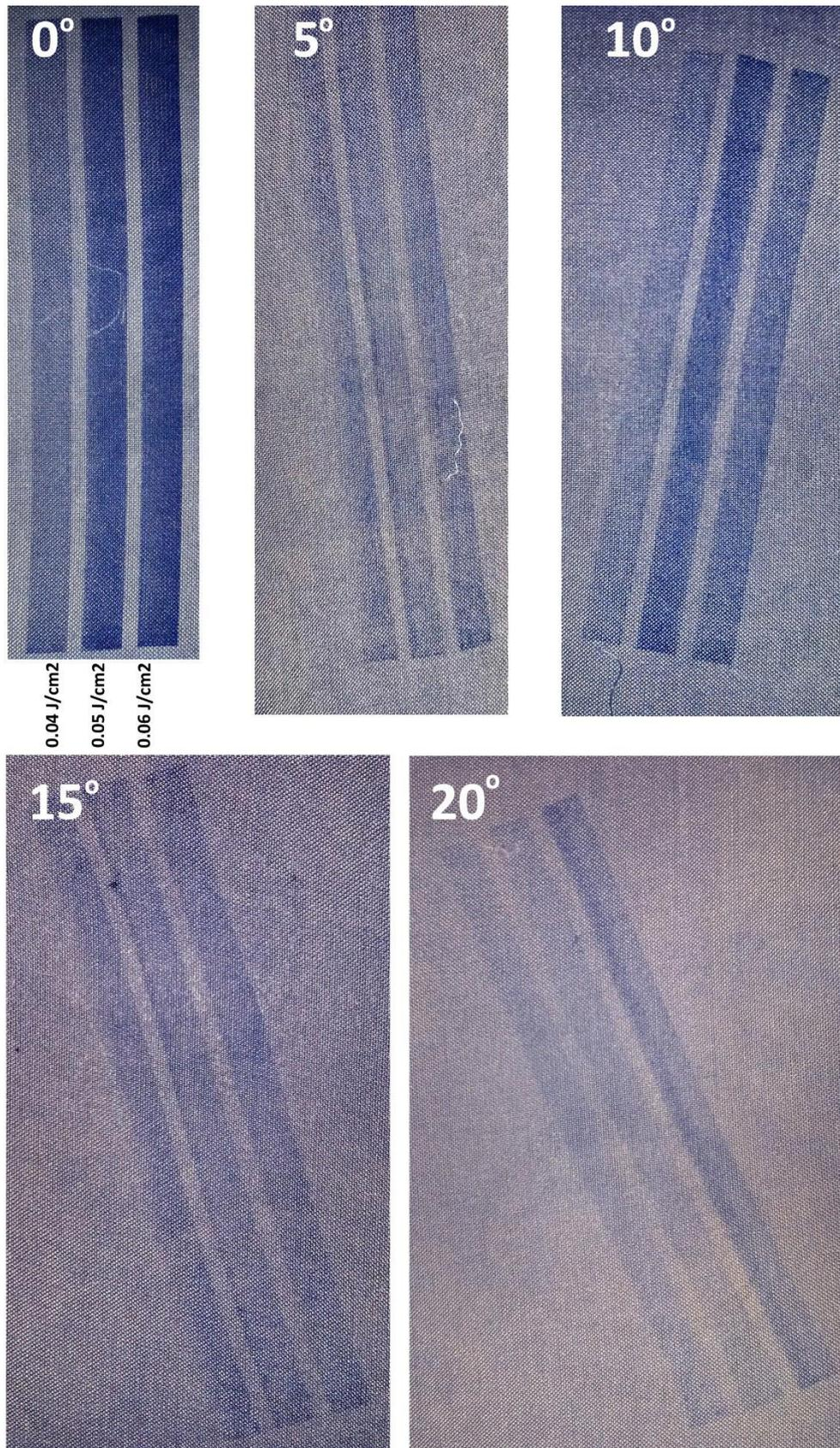
Figure 160: Axis experiments with woven PET samples laser modified at 0°, 5°, 10°, 15° and 20°
