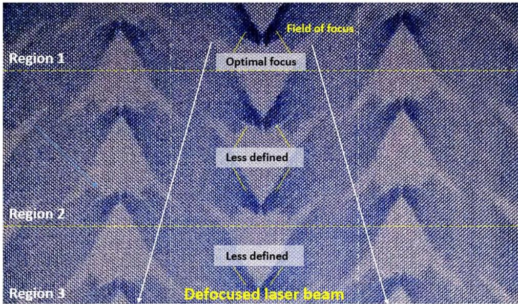
Figure 59: FLD processed woven PET sample showing reduced sharpness due to defocused beam
