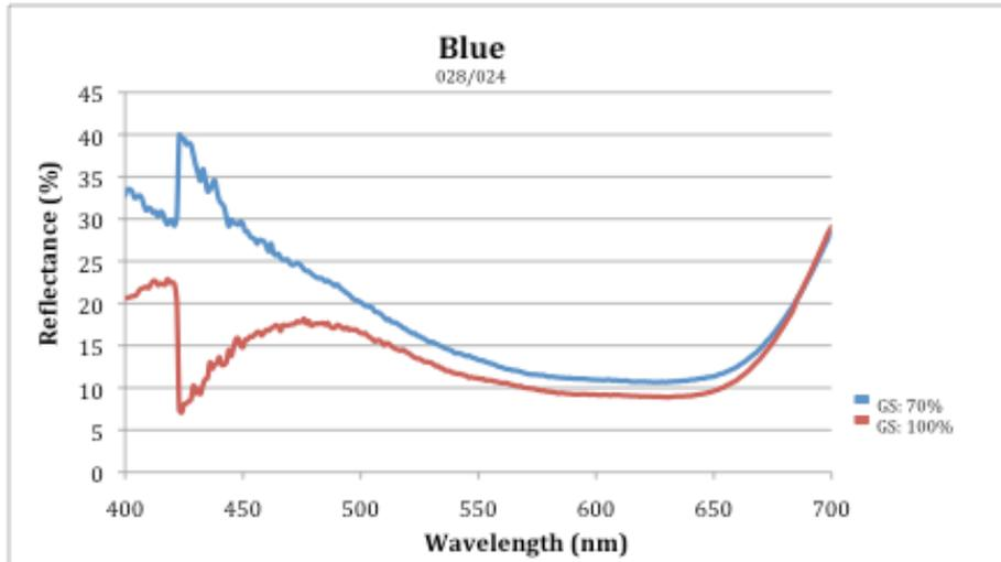
Figure 96: Reflectance/Batch 1: Blue - Laser-dyed fabrics: GS: 70% and GS: 100% (*Blue*)
