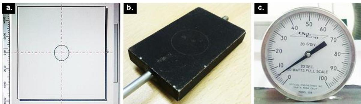
Figure 42: Computer screen/central spot (a); 10-100W Power meter probe (b); and gauge (c)
