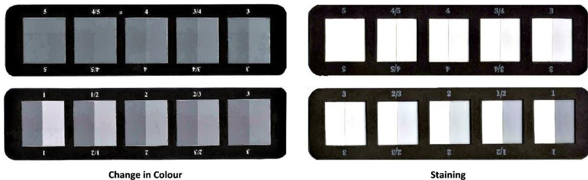
Figure 119: ISO Grey scales for assessing Change in Colour and Staining
