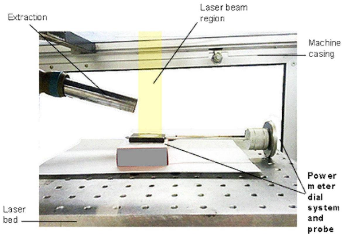
Figure 41: Measuring power output of CO<sub>2</sub> Synrad 10W laser marker
