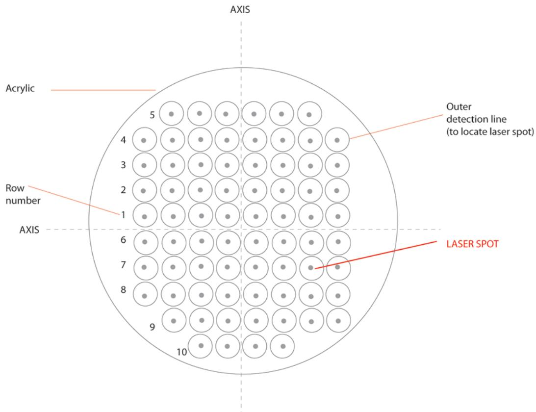
Figure 39: Burn print in a circular piece of acrylic showing the layout of multiple laser spots
