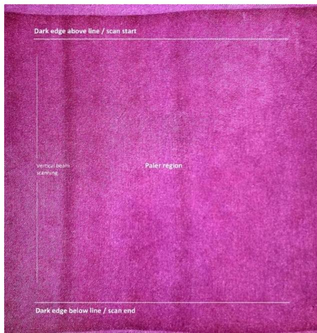
Figure 65: FLD fabric sample (no pattern) showing darker edges due to inertia (woven PET)
