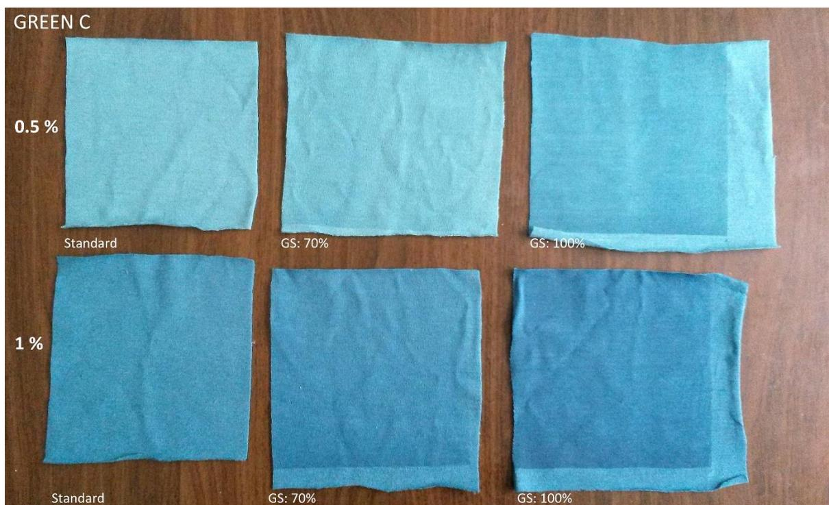
Figure 102: Fabric samples used in reflectance testing (Batch: *Green C*)
