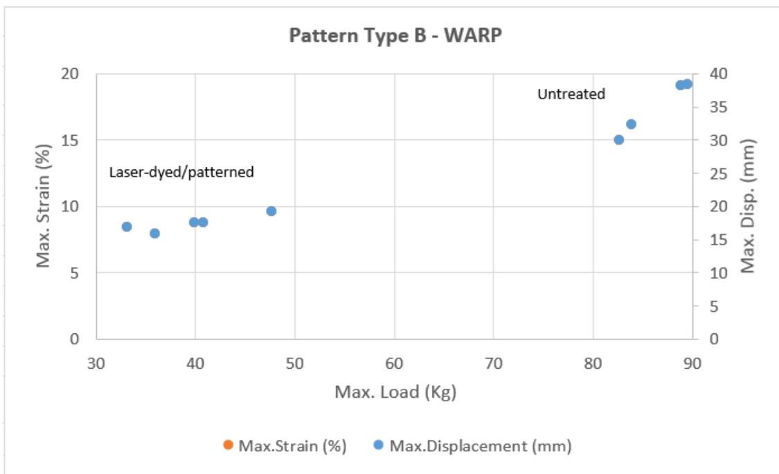
Figure 126: Tensile Strength results graph: WARP - Pattern Type B and Untreated fabric
