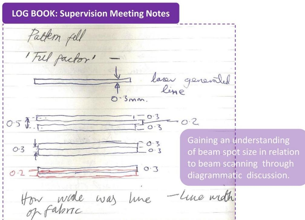
Figure 86: Log book notes - beam spot size versus vector line spacing
