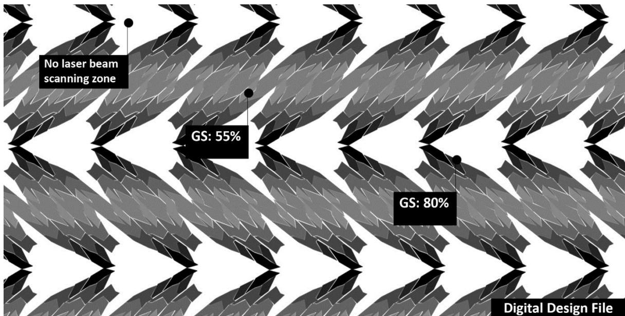
Figure 110: Digital design file with a range of grey tones (GS %) which form an all over repeat design
