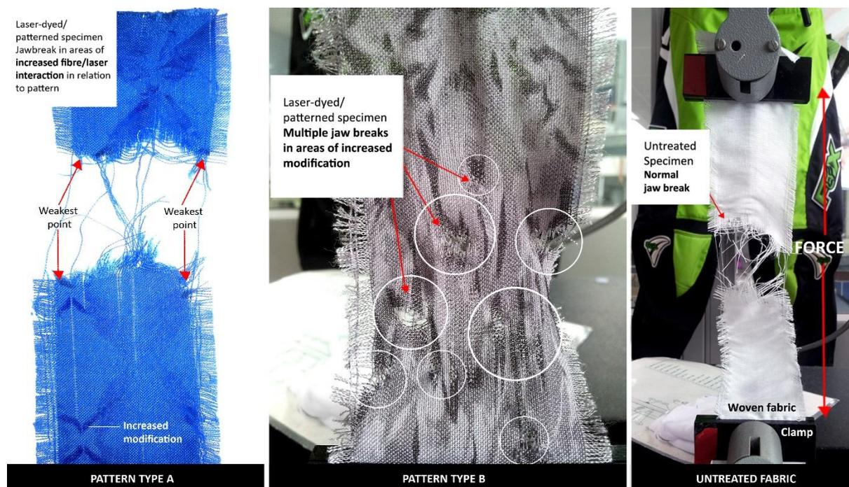
Figure 127: Tensile strength tests showing jaw break: Pattern Type A, B and Untreated specimen
