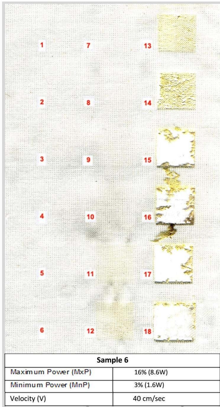
Figure 53: Laser treated ISO woven polyester with an 18 shade greyscale
