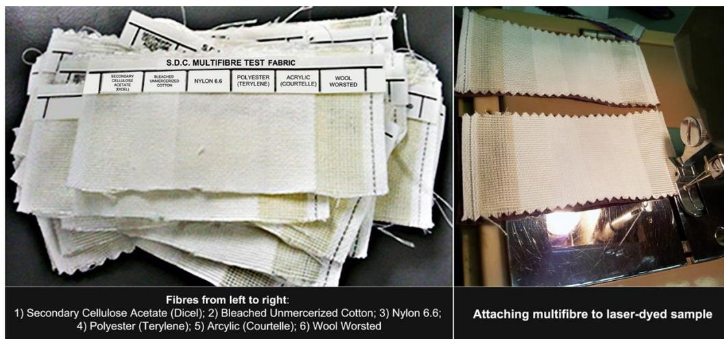
Figure 116: SDC Multifibre DW; Prepared for wash fastness tests
