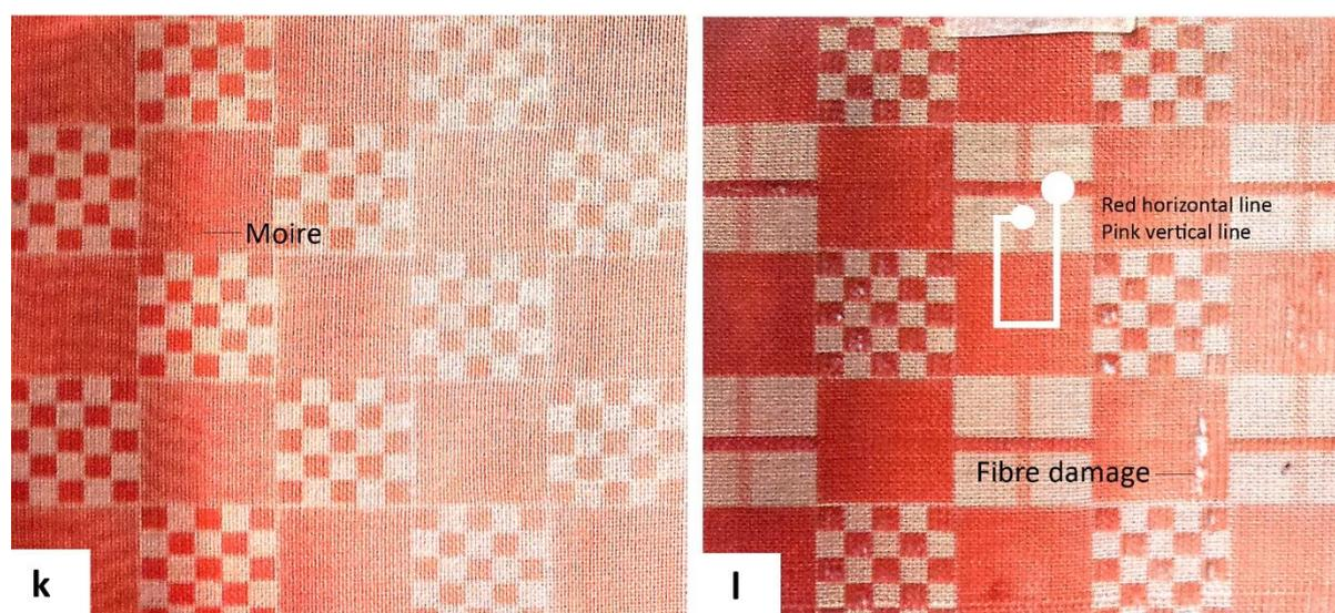
Figure 156: FDL samples: gradient pattern effects
