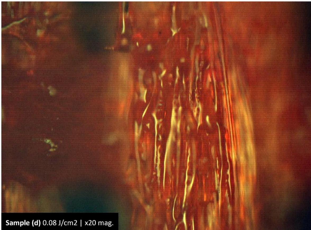
Figure 153: Sample (d): showing damaged fibres when processed with 0.08 J/cm<sup>2</sup> energy density.
