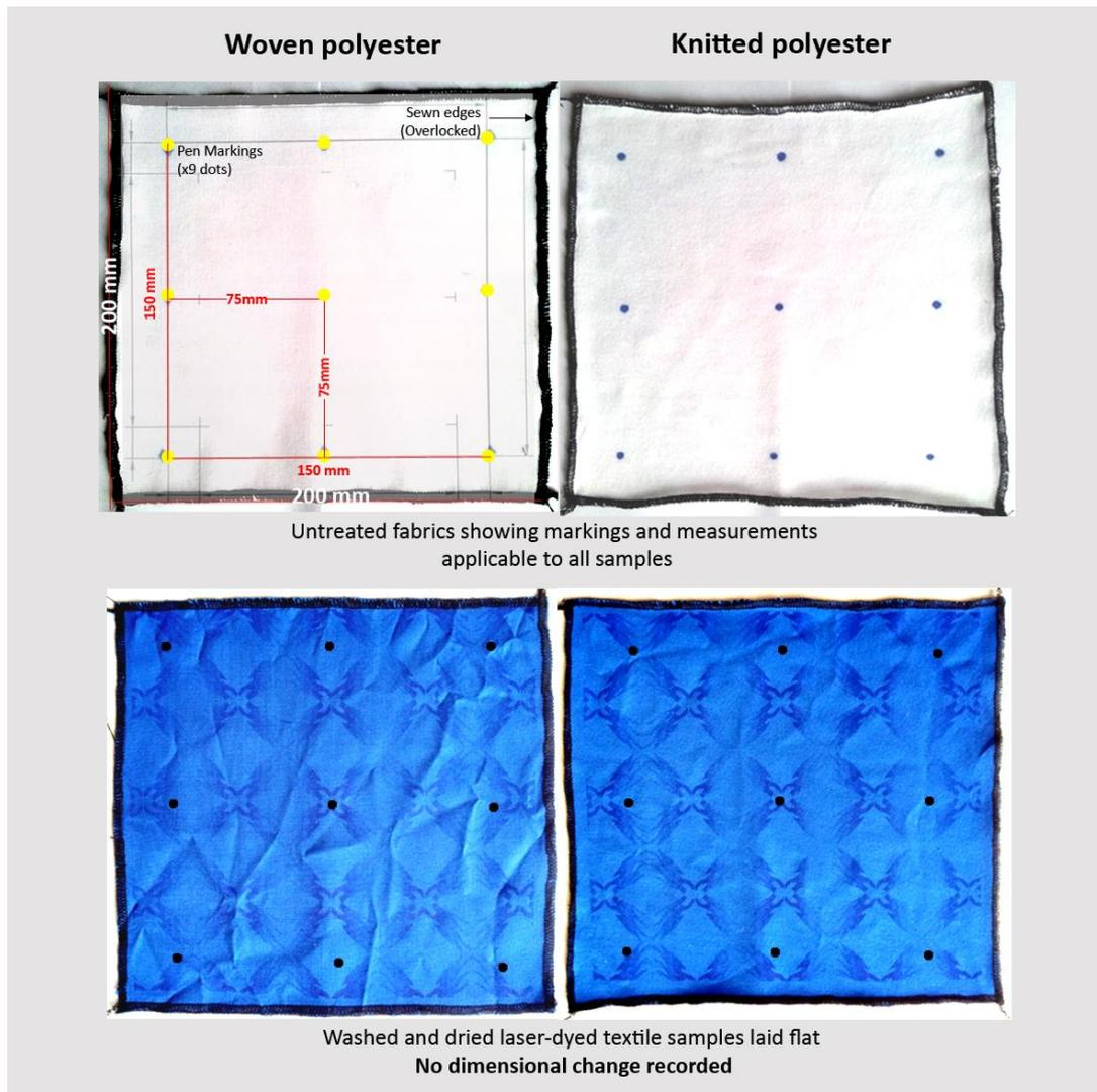
Figure 135: Samples tested for dimensional stability
