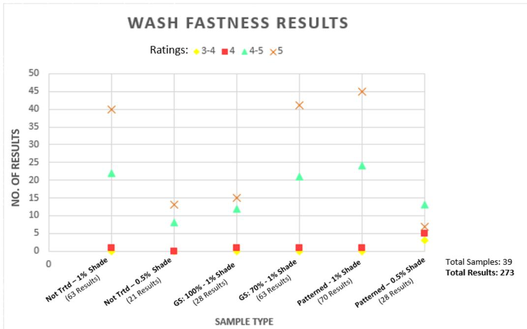
Figure 120: Wash fastness test results graph
