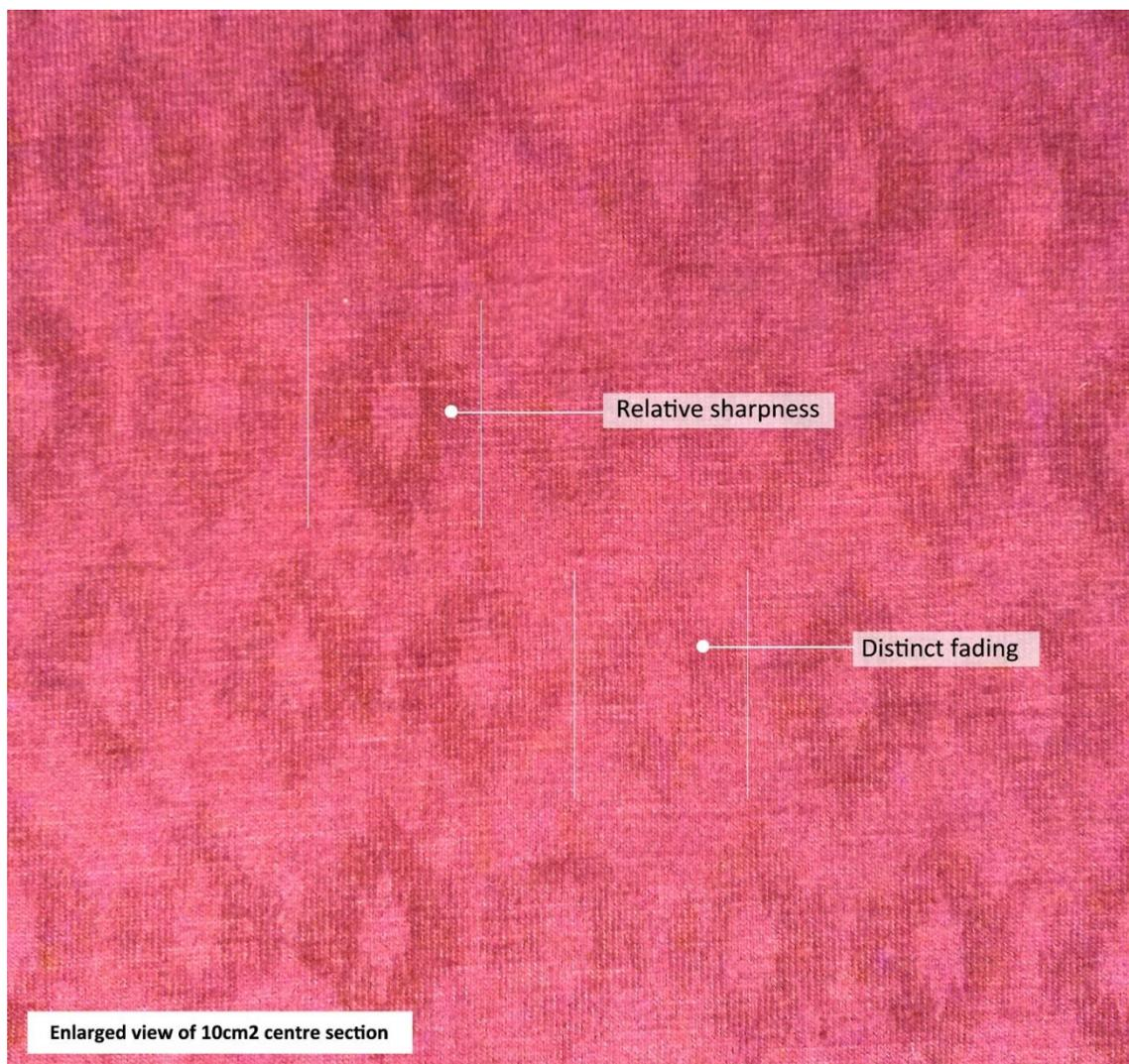
Figure 72: Vertically scanned pattern showing some interruption of image on the laser-dyed PET knit
