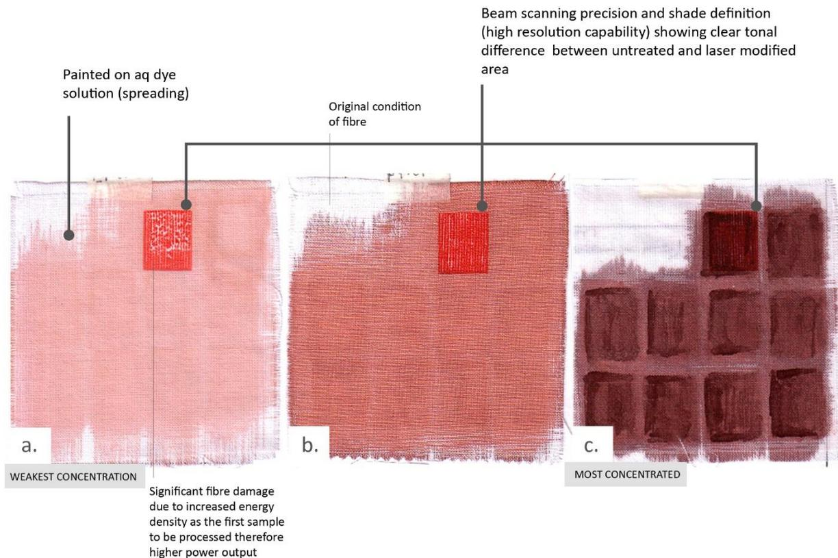
Figure 150: Laser modified blocks using a variable dye concentration water based approach
