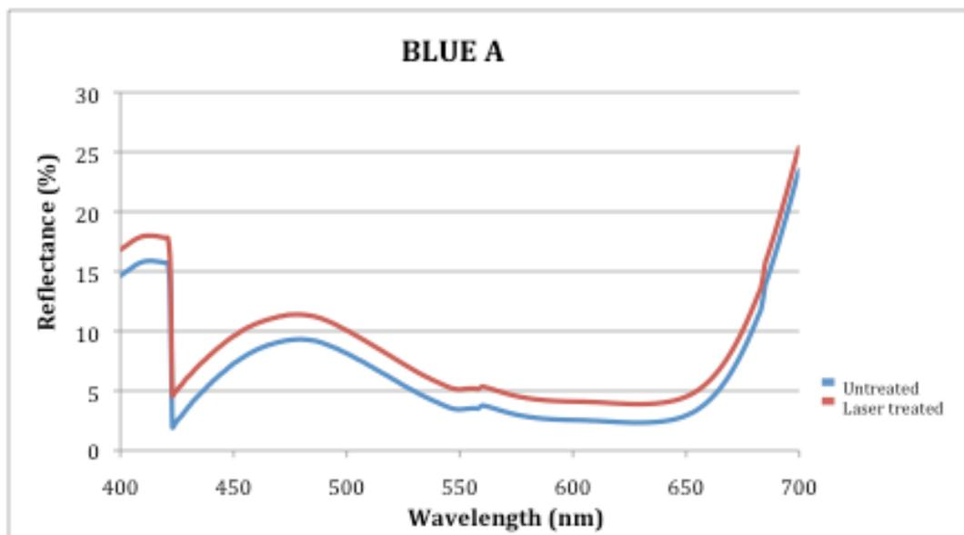
Figure 95: Reflectance/Batch 1: Blue - Laser treated: GS: 70% (*Blue A*) and untreated fabrics
