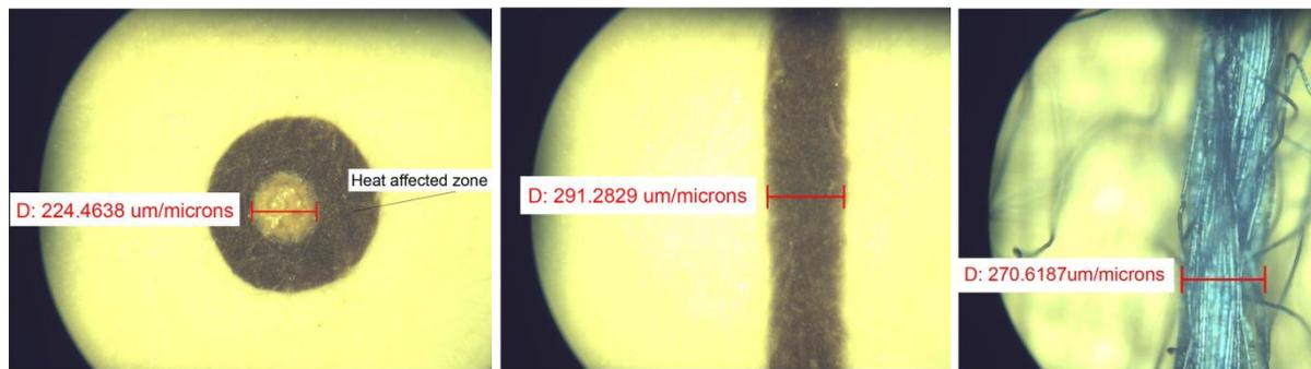
Spot mark fired onto Dioptron light sensitive paper      Line mark fired onto Dioptron light sensitive paper      Individual dyed polyester yarn fibre
