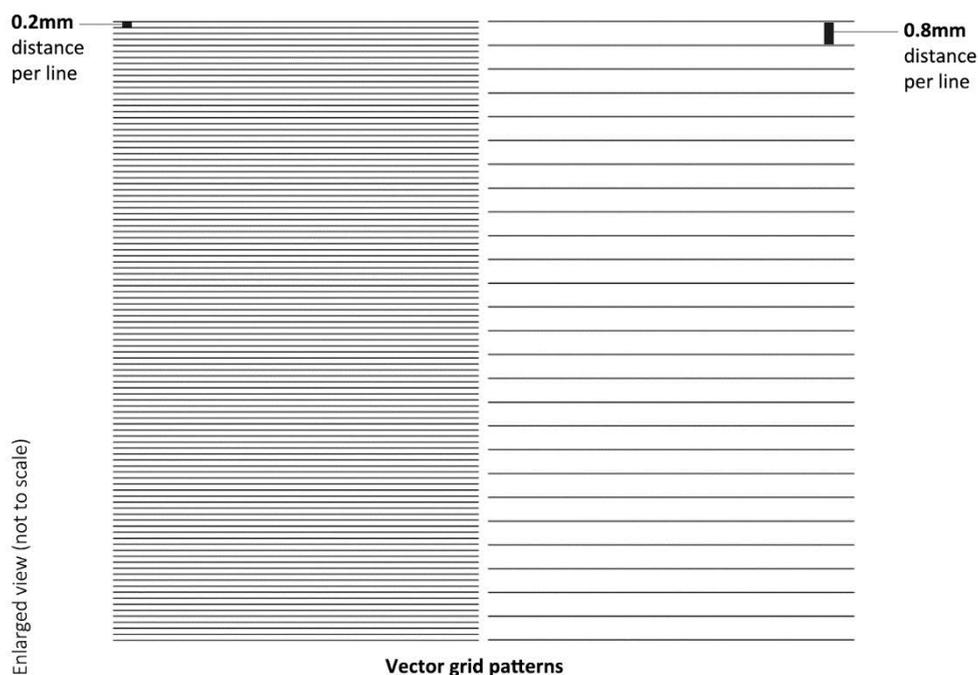
Figure 85: Vector generated linear grid patterns
