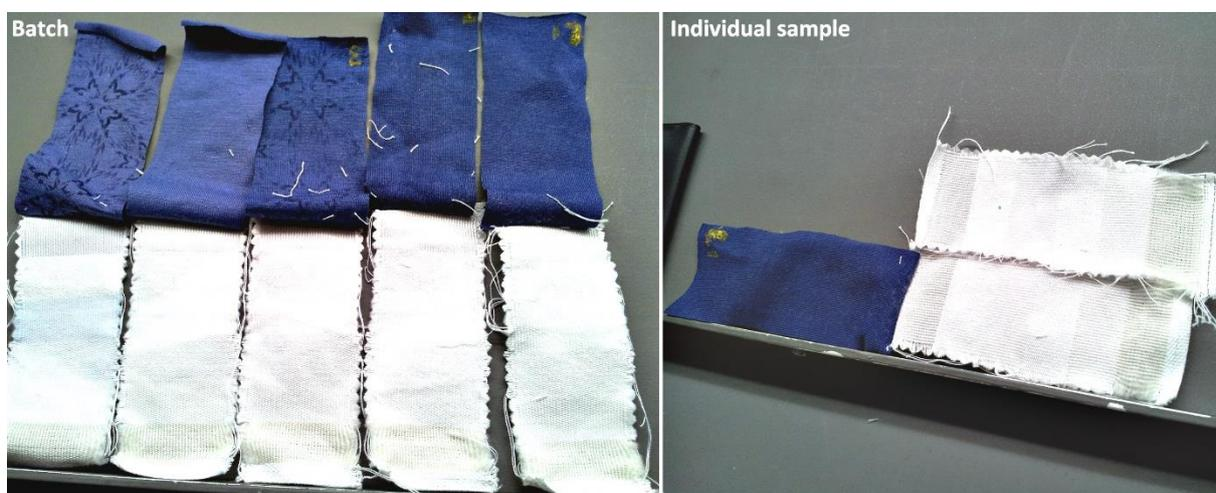
Figure 118: Fabrics assessed inside light cabinet for wash fastness by batch and per specimen
