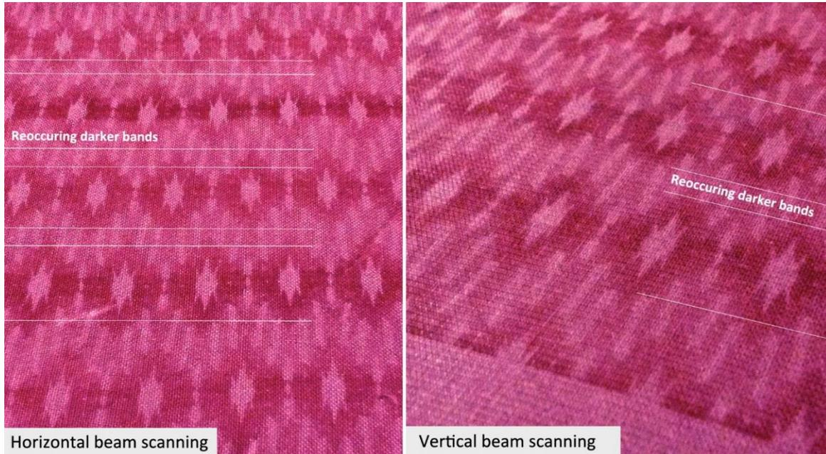
Figure 62: Visible overlapping 'streaking' effect as a result of beam overlap during scanning
