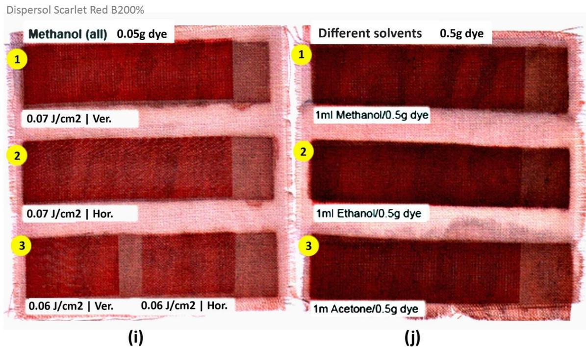
Figure 155: Solvent based samples
