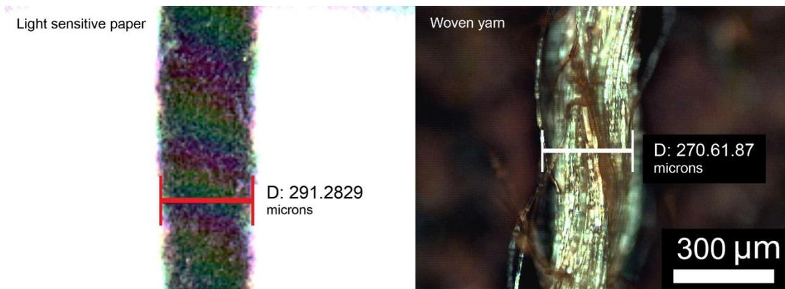
Figure 79: Laser beam scan with Synrad 60W Laser (left), Individual woven polyester yarn (right), x10.100 magnification
