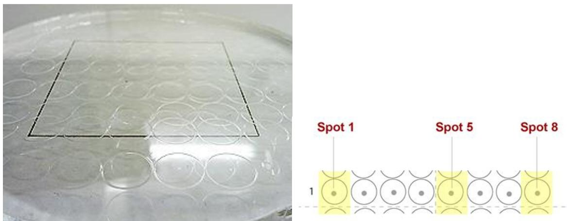
b. (Left) Orientation of burn print: laser spots fired on to acrylic specimen;
