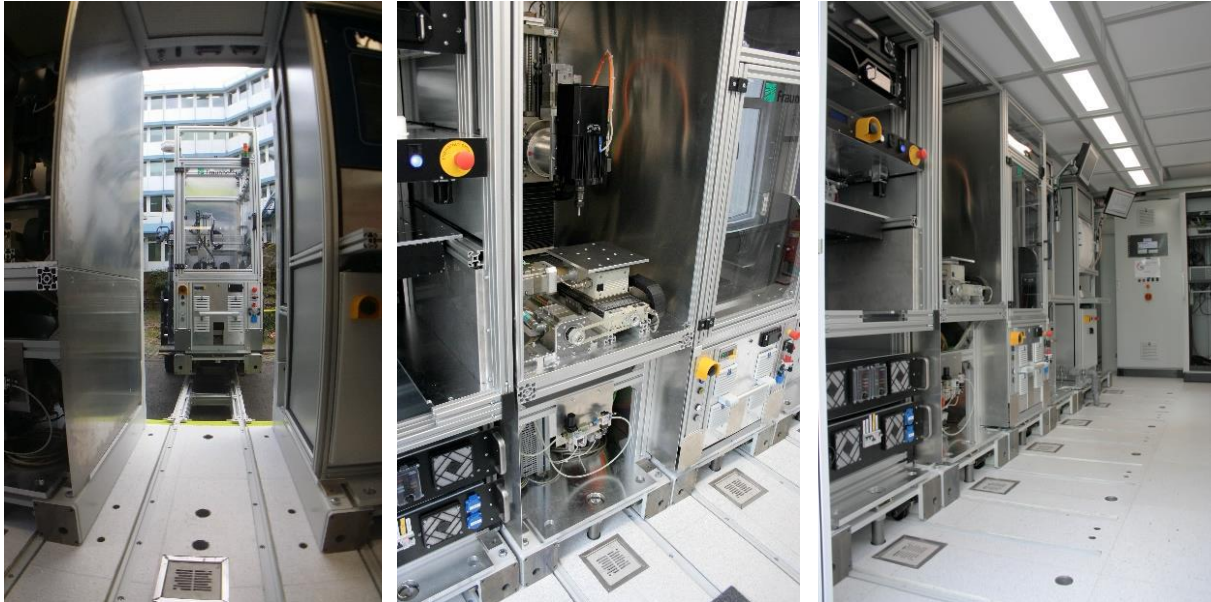
Figure 20: Process module integration (left), installed process modules (middle), view of equipment front and the operator`s corridor (right).
