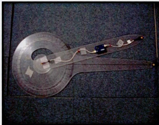
Figure 3.2: Markers placed on a simple goniometer to measure reliability of camera system
