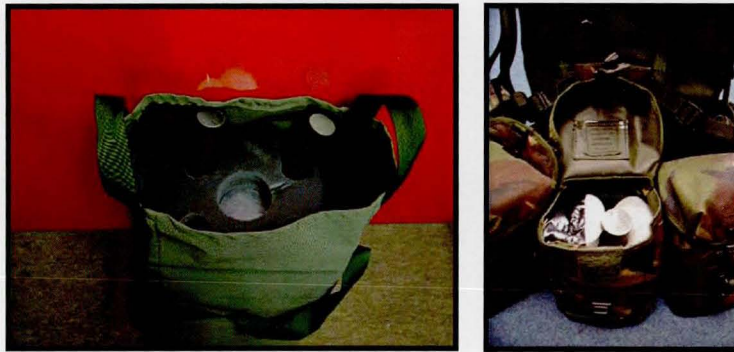
Figure 3.18: Weight block (left) and steel rods (right) used to load LCSs
