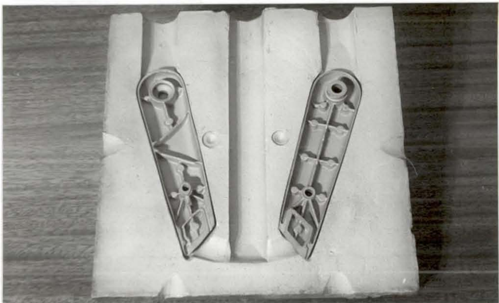
Permanent metal mould in LM6 - resultant castings, resting in mould cavity, made in KAYEM 12.
