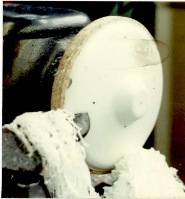
Completed shell mould in W.E.P., note thickness gauges - small brown dots.
