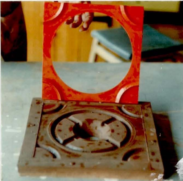
Plaster pattern for permanent metal mould. Wooden pattern removed.
