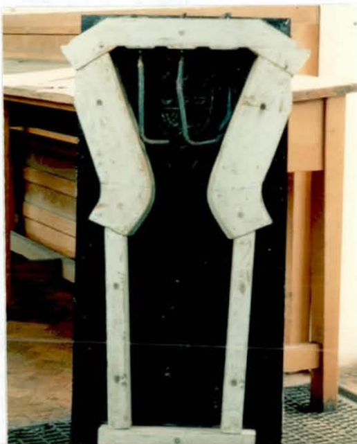
Mould for bench end made in G.R.P. and timber. Impression of school crest taken from plasticine original.
