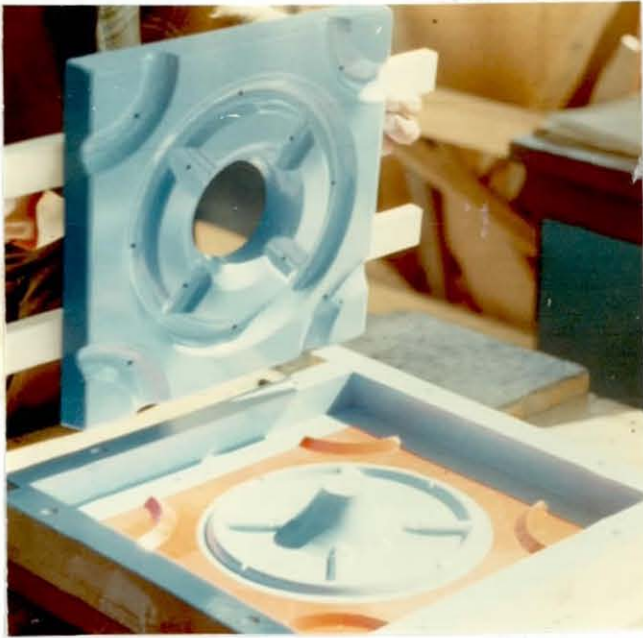
Open mould for patric cast. Note recesses to give uniform metal section.
