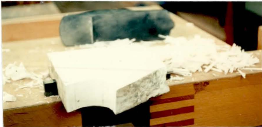
W.E.P. can be worked by all hand and machine tools: note the shavings made by this smoothing plane.
