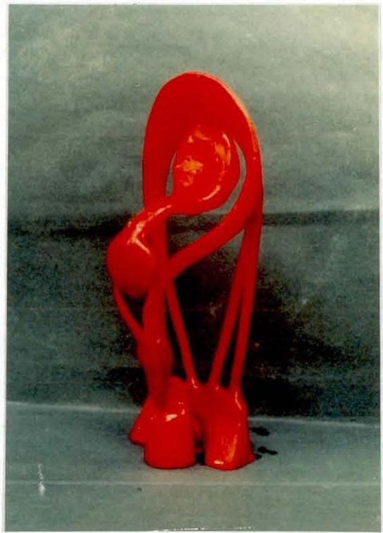
Wax for stylized Impala ready for investment; note built in feeder to horns and body.
