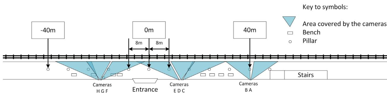
Figure 3 – Platform diagram and positioning of the video cameras
