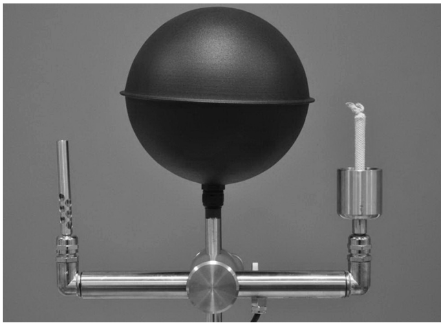
Figure 1 Official WBGT instrument according to ISO 7726 and ISO 7243, showing (left to right) shielded dry bulb, black globe (15 cm diameter), and natural wet bulb (wetted cotton wick over sensor with water reservoir below) sensors.
