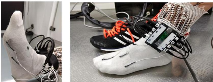
**Figure 2 Positioning of temperature and relative humidity sensors on the right foot.**
