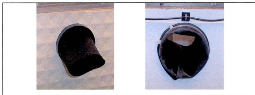
Figure 2.5 and Figure 2.6 show the armhole from the inside and outside of the freezer door.
