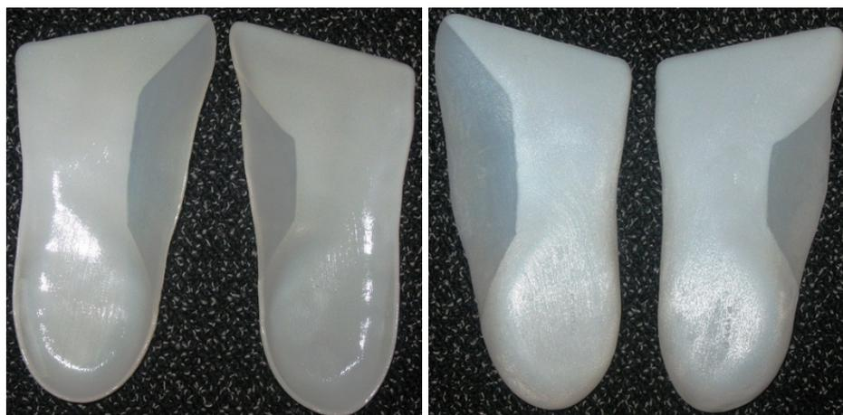
**Figure 7.2.** Top (left) and bottom (right) views of a pair of personalised insoles developed using multiple materials.
