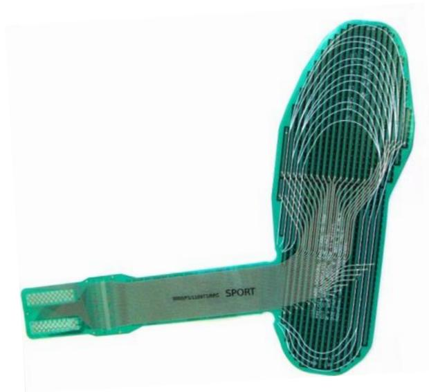
**Figure 4.7.** The Tekscan in-shoe plantar pressure sensor before trimming.
