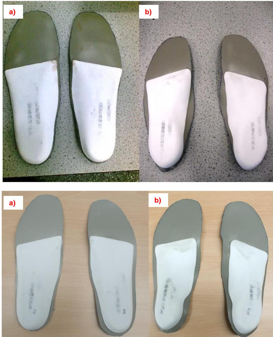
**Figure 5.24.** Bottom views of the (a) control and (b) personalised insoles after 1.5 (top images) and 3 months (bottom images) of usage.
