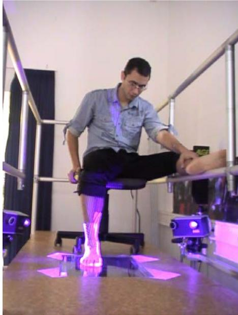
**Figure 6.2.** Participant having the foot scanned for the static design.
