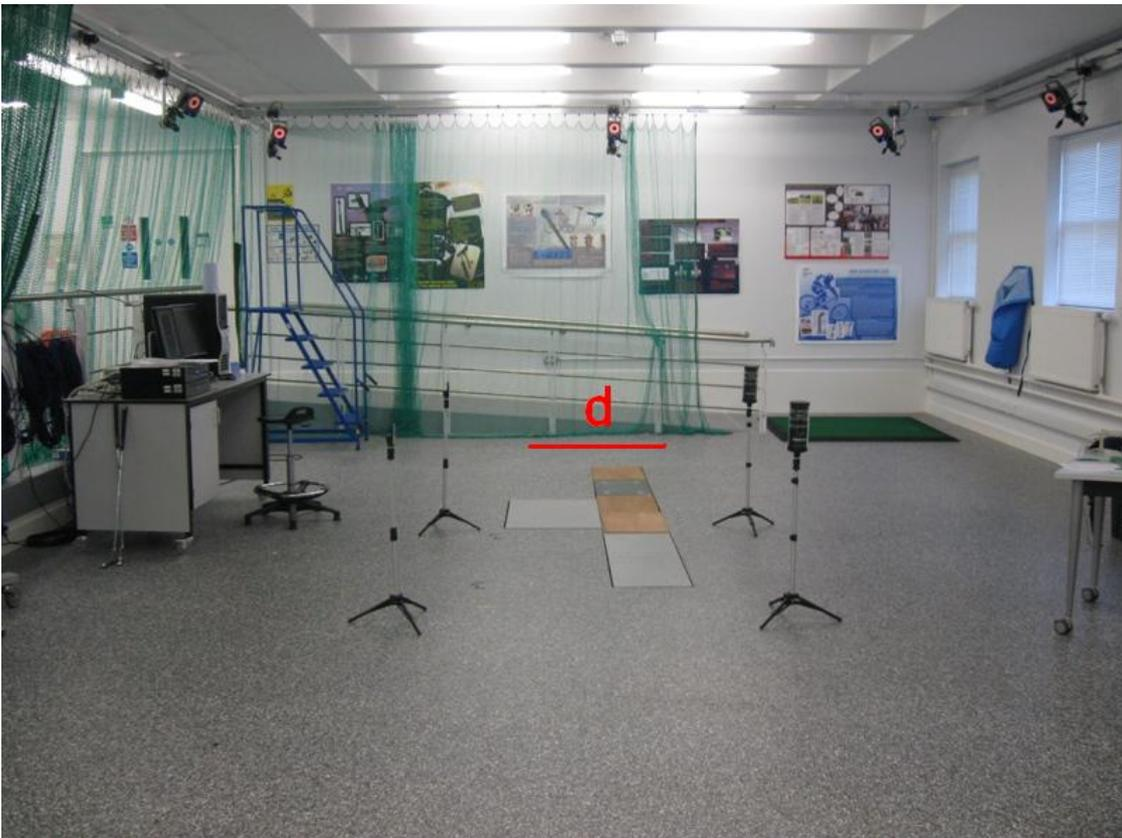
**Figure 5.7.** Views of the laboratory set up with the 10-m runway, electronic timing gates and Vicon system; (a: 2-metres distance between timing gates; b: start of the runway; c: the force platform used in the study; and d: end of runway).
