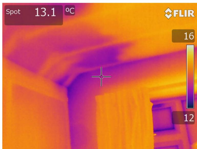
**Figure 8 IR image 2 of the air leakage path in Alison's bedroom**
