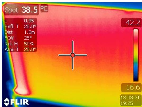
Figure 44 IR image of the kitchen radiator
