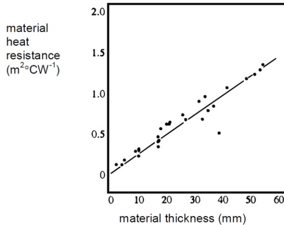
**Figure 13** Relation between clothing material insulation and the material thickness (Havenith and Wammes in Lotens 1993).
