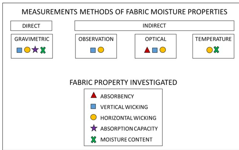
**Figure 22** Diagram representing the measurement methods to measure fabric moisture absorption and transport properties.
