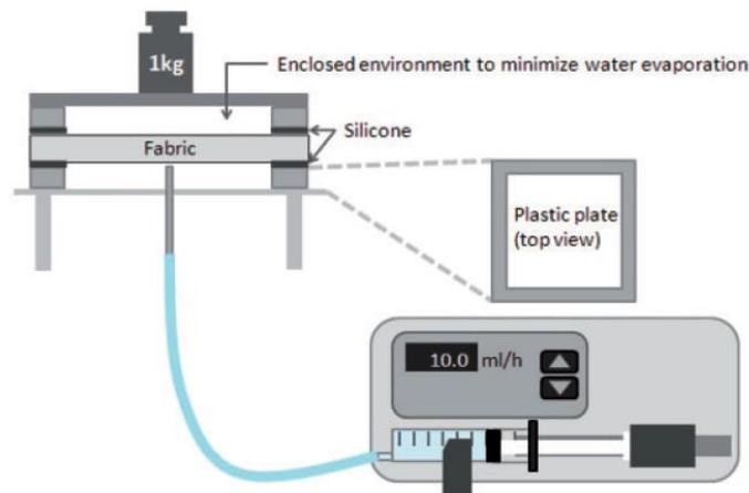
**Figure 23** Schematic drawing of horizontal wicking test. From Tang et al., 2014.
