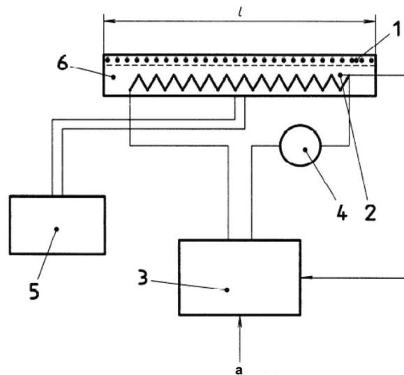
**Figure 17**-Measuring unit with temperature and water supply control. 1 metal plate; 2 temperature sensor; 3 temperature controller; 4 heating-power measuring device; 5 water-dosing service; 6 metal block with heating element. From BS EN ISO 11092:2014.
