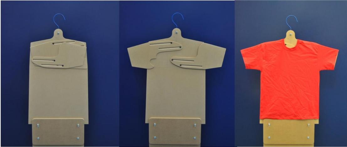
**Figure 4** Custom-made T-Shirt-like shape stand, used for the image acquisition of the experimental garment in Study 5.
