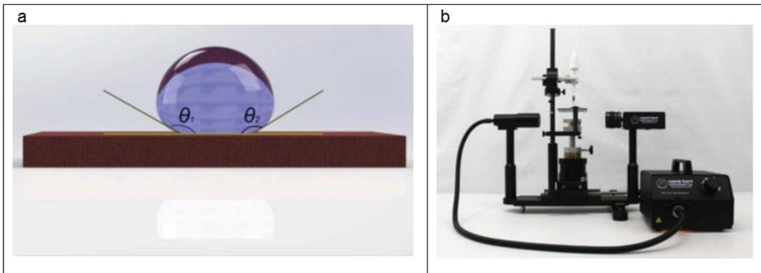
**Figure 24** (a) Tangential lines at the borders of the water drop. (b) Contact Angle Goniometer/Tensiometer (rame-hart Model 260). From Tang et al. 2014.
