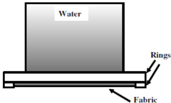
Figure 21-Inverted cup assembly. From ASTM E96 1999
