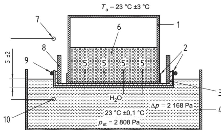
**Figure 19**-Schematic test arrangement for the desiccant cup method. 1 measuring cup; 2 membranes; 3 textile specimen; 4 water bath; 5 water vapour; 6 saturated potassium acetate solution; 7 temperature sensor for ambient temperature; 8 specimen holder; 9 rubber ring; 10 temperature sensor. From BS EN ISO 15496:2004.
