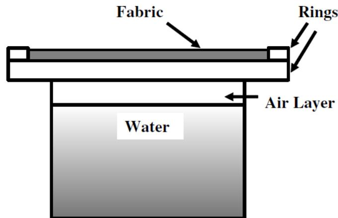
**Figure 20**-Upright cup assembly. From ASTM E96 1999
