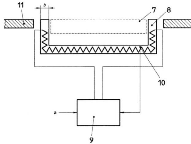
**Figure 18**-Thermal guard with temperature controller. 7 measuring unit (according to Fig 1); 8 thermal guard; 9 temperature controller (according to fig 1); 10 temperature sensor (according to fig 1); 11 measuring table. From ISO 11092.
