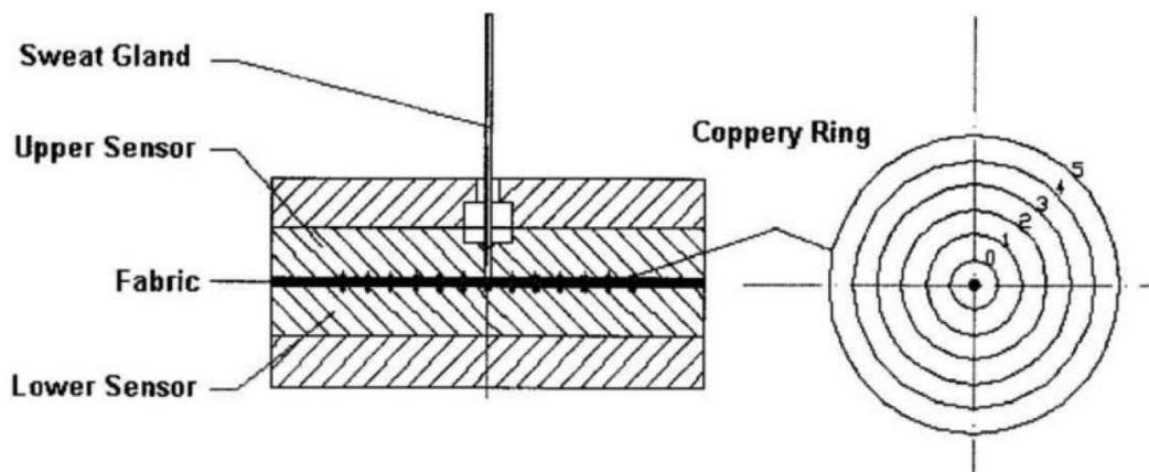
Figure 25-Sketch of the Moisture Management Sensors. From Hu et al., 2005.
