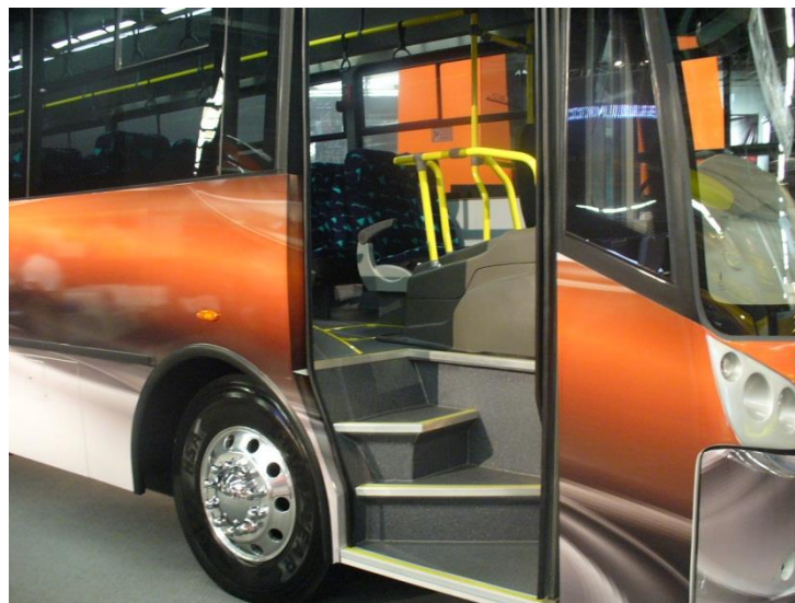
Figure 5.8 Example of a bus with steps in curve (main reason for this design is that the engine is placed in front of the bus-truck)
