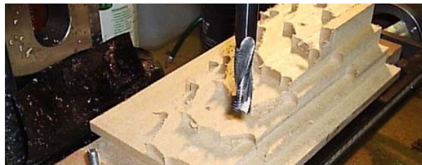
Figure 97: CNC milling on a medium-density fibreboard
