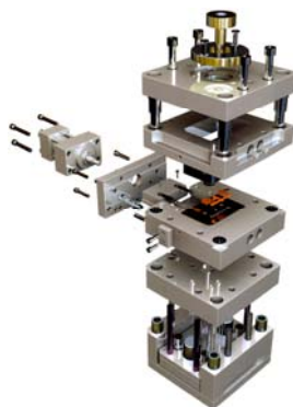
Figure 159: An exploded illustration of a two-cavity mould (Pipes 2007)
