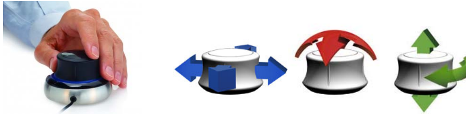
Figure 98: Panning left / right and zoom, panning up / down and rotate, and tilting functions with the SpaceNavigator controller cap
