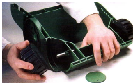
Figure 175: Assembly of an appearance prototype for a lawnmower (Garner 2006)
