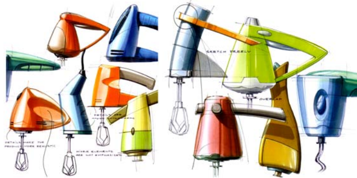
Figure 195: The use of colour, shading, outlining and details to show the visual character of a product concept (Eissen and Steur 2008)
