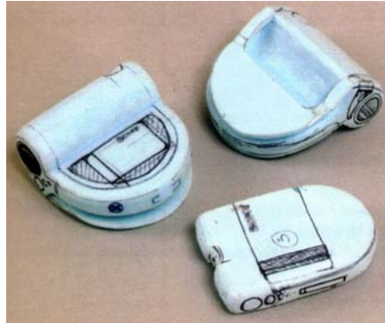
Figure 164: Rigid cellular foam models of products where markers have been used to show details (Garner 2006)
