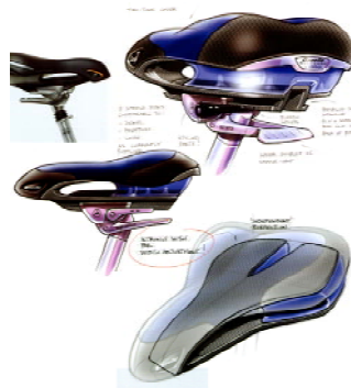
Figure 211: Rendering of a rubberised bicycle seat (Eissen and Steur 2008)
