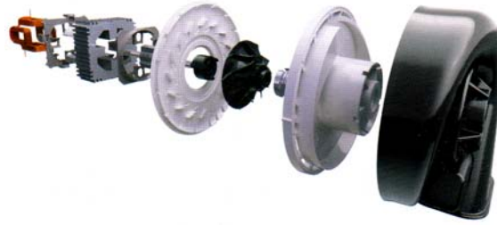
Figure 234: CAD representation of an exploded view for the Dyson vacuum cleaner motor (Pipes 2007)
