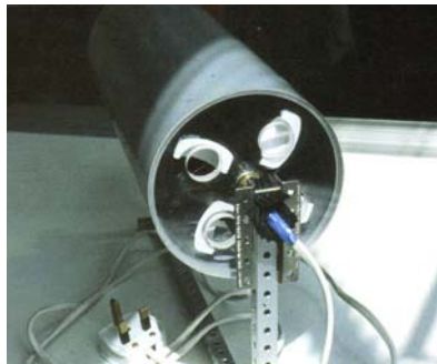
Figure 168: Principle-proving model of a drive system produced during the industrial design of a lawnmower (Garner 2006)
