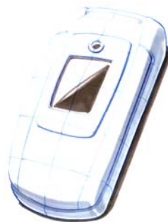
Figure 230: Profile lines of a mobile phone (Pavel 2005)
