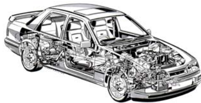
Figure 157: Manual ink drawing of a technical illustration with thick lines for important areas and the use of shading and break lines (Pipes 2007)
