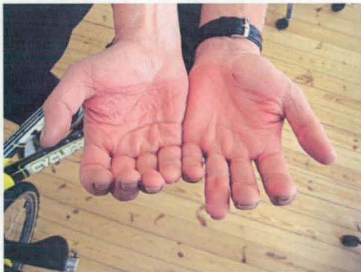
Figure 12.8 The effect of palm pressure from a traditional handle, left, and the new design, right.
