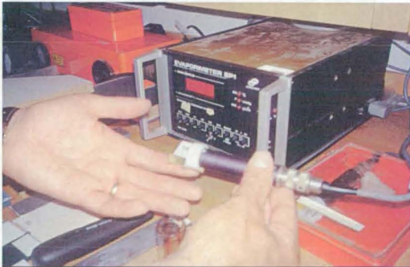
Figure 8.4 The probe for recording skin moisture applied on the researched skin location
