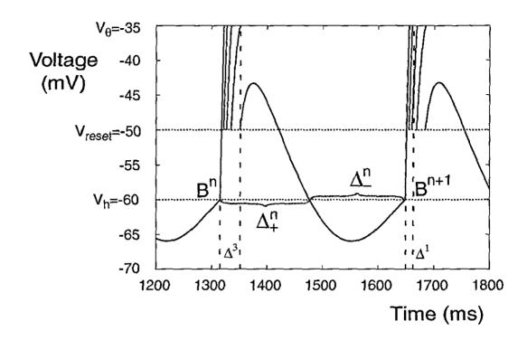
**Figure 5.3** The integrate-and-fire-or-burst model of a neuron periodically stimulated by a sinusoid:  $I_{app} = 0.1 + 0.25\cos(6\pi x/1000)$ . All other parameter values are given in table 5.1. See the text for an explanation of the various labels.
