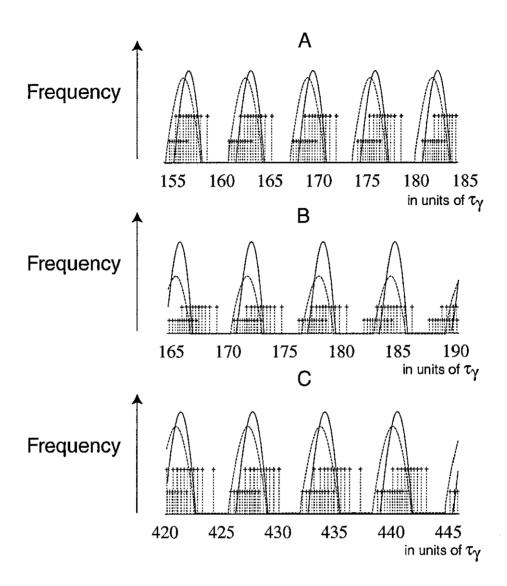
**Figure 3.8** Comparison of the integrate-and-fire dynamics and the analog model in the bursting regime. Output is created by cimparing direct numerical simulation of equation (3.3) and (3.4) (with balance equation (3.7)) with that of equations (3.15). Parameter values  $\alpha=0.5,~I=2,~A:~\gamma=0.99,~\tau=5.0,~\epsilon=3.5,~B:~\gamma=0.9,~\tau_{\gamma}=5.0,~\epsilon=8.0,~C:~\gamma=0.9,~\tau=0.2,~\epsilon=3.5.$  See the text for a description of the dynamics.
