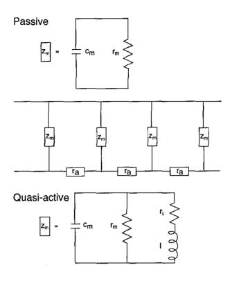
**Figure 2.7** A schematic description of passive and quasi-active membranes in terms of electrical circuit diagrams. The passive dendrite can be viewed as a capacitor  $c_m$  in parallel with a resistance  $r_m$ . A quasi-active dendrite has an additional inductive branch with a resistance  $r_l$  in series with an inductance l.
