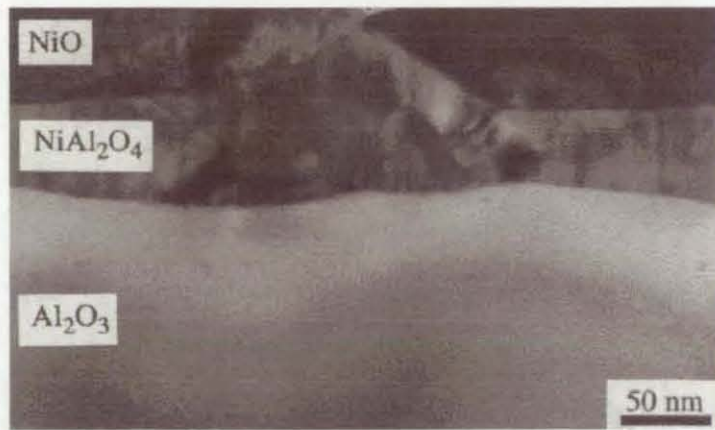
Figure 7.1: Cross section TEM image of spinel formation at a NiO/Al 2 O 3 interface at 1375 K. NiO was first deposited on Al 2 O 3 by pulsed laser deposition, then the system was heat treated to initiate the spinel reaction. Courtesy of M. T. Johnson et al. [96].
