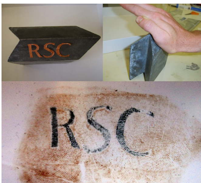
Fig.2 The effect of rubeanic acid treatment of a gel-lift from a hand that has briefly touched (top right) the copper logo on a lead brick (top left).
