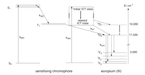
Scheme 2 Jablonski diagram illustrating sensitised emission of Eu(III), either via an intermediate chromophore triplet or a solvent-relaxed internal charge transfer excited state.
