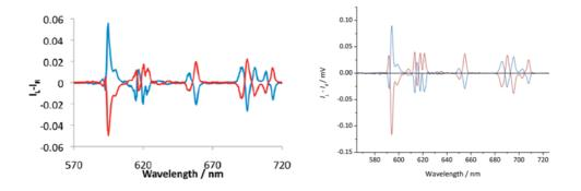
Figure 6 Circularly polarized luminescence spectra for: *left*,  $\Delta$ -[Eu.L<sup>2</sup>] (blue) and the  $\Lambda$  isomer (red) (50µM, H<sub>2</sub>O, 295K,  $\lambda_{exc}$  280 nm); *right*,  $\Delta$  (blue) and  $\Lambda$  (red) [Eu.L<sup>7</sup>] (3 µM; 295K, MeOH,  $\lambda_{exc}$  360 nm), showing the enhanced spectral resolution, e.g. for the  $\Delta J = 4$  transitions around 700 nm (*viz*. Fig. 4 [C and D] above). <sup>25,26,31</sup>
