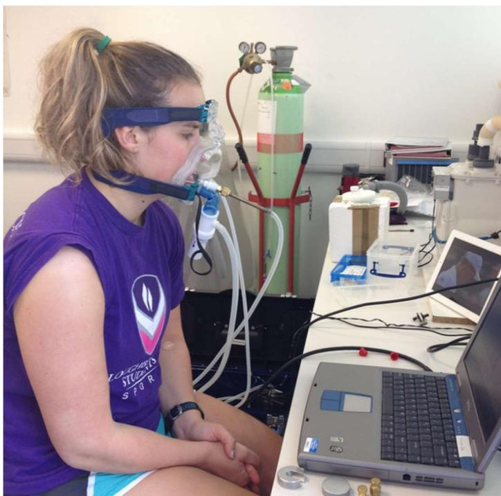
**Figure 5.3.5.1. Photo of exhaled breath VOCs sample collection using portable breath sampler**
