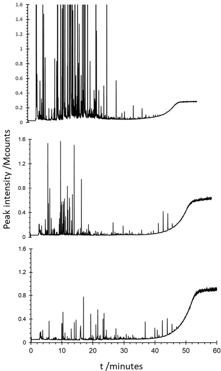
**Figure 4.5.4.1. TIC chromatogram illustrating participant breath sample using the portable breath sampler (top), room air (middle) and purified air supply (bottom)**
