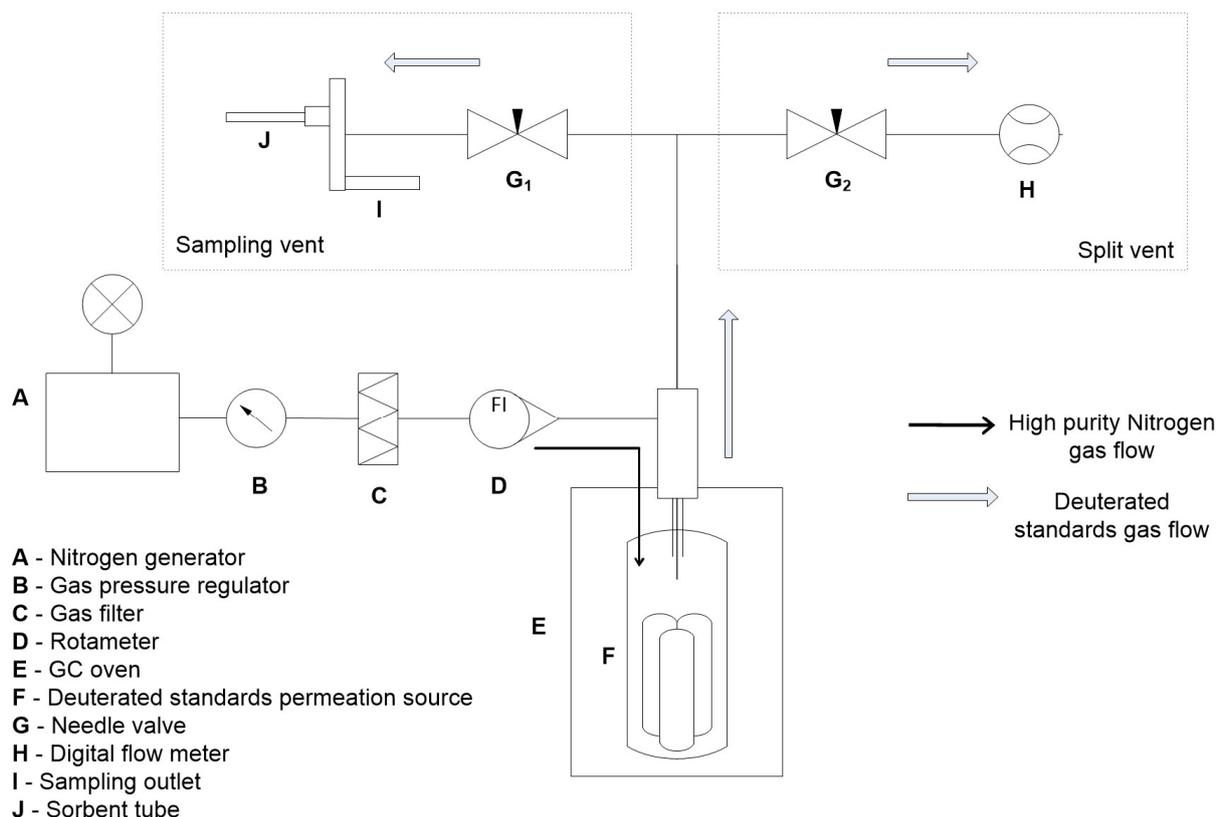
**Figure 3.2.2. Schematic diagram of internal standards permeation system**
