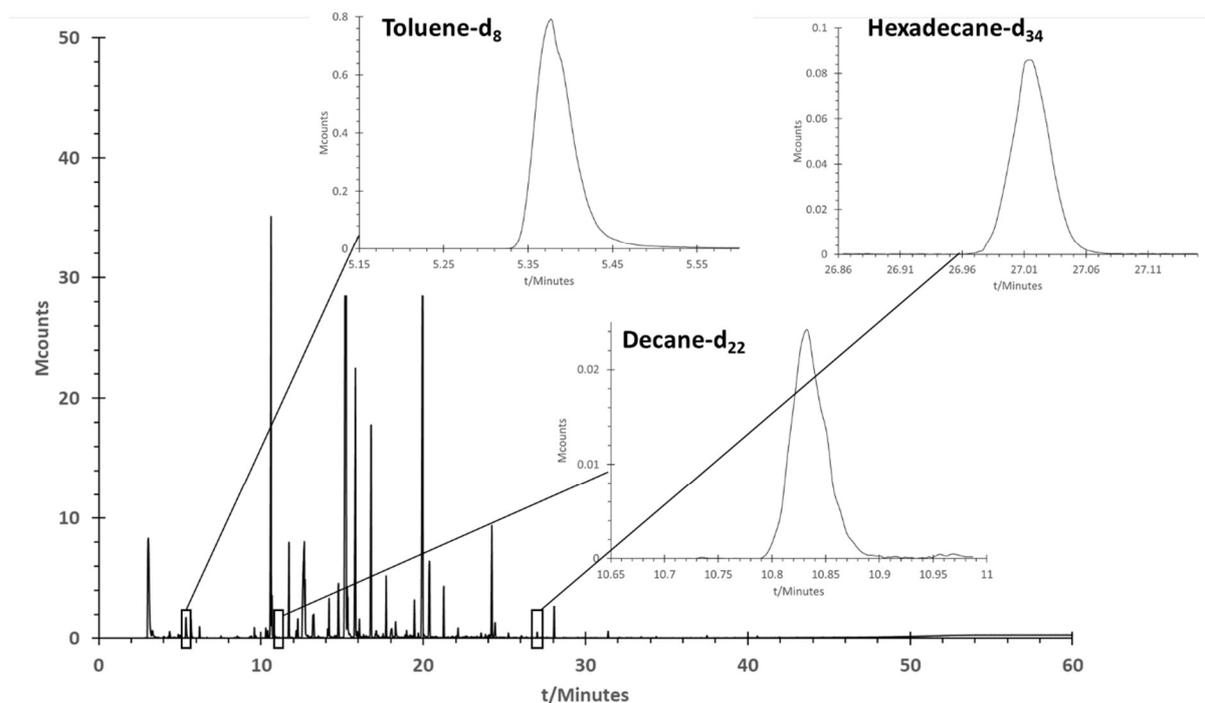
**Figure 3.2.3.1. TIC chromatogram of 2.5 L breath sample doped with internal standards toluene-d<sub>8</sub>, decane-d<sub>22</sub> and hexadecane-d<sub>34</sub>. The EIC chromatogram of the three internal standards are shown on the right hand.**
