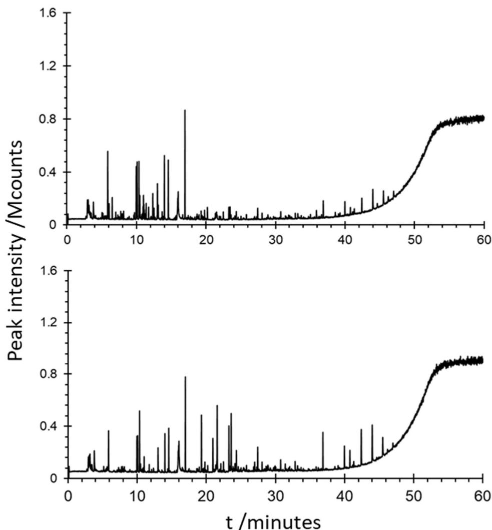
**Figure 4.5.2.2. TIC chromatogram of purified air supply from two sources on the same day: purification elements from original adaptive breath sampler (top) and custom built purification unit from portable breath sampler (bottom)**
