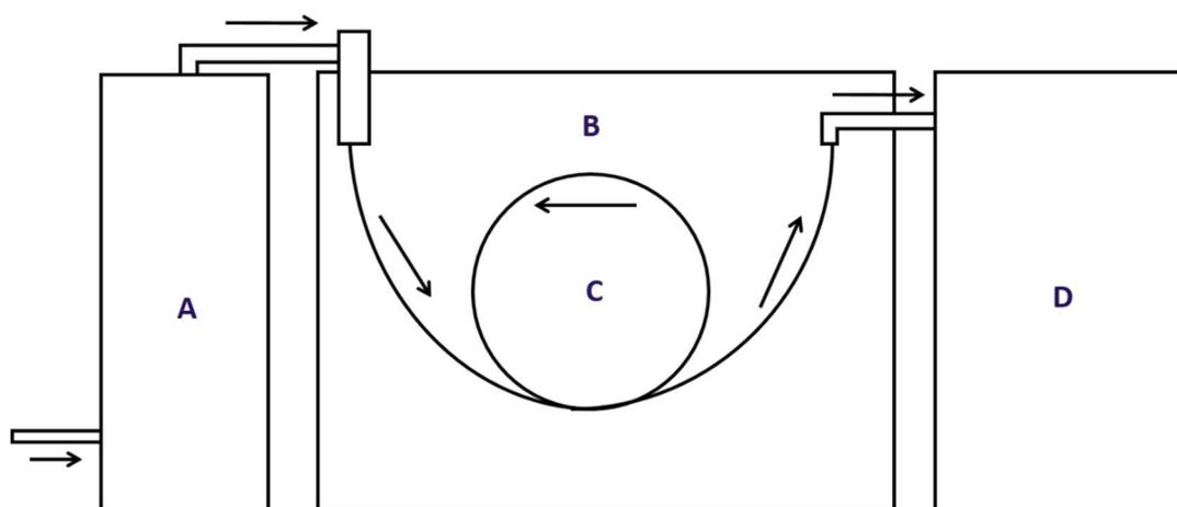
**Figure 2.3. Schematic diagram of TD-GC-MS setup used in breath analysis. High purity helium is pumped into Unity Series 1 thermal desorption unit coupled to an Ultra thermal desorption auto sampler unit (A) where breath sample collected on adsorbent tubes is injected into Varian 3800 gas chromatograph (B) and separated using a DB-5 capillary column (C), the separated breath sample is then analysed using a Varian Saturn 4000 ion trap mass spectrometer (D)**
