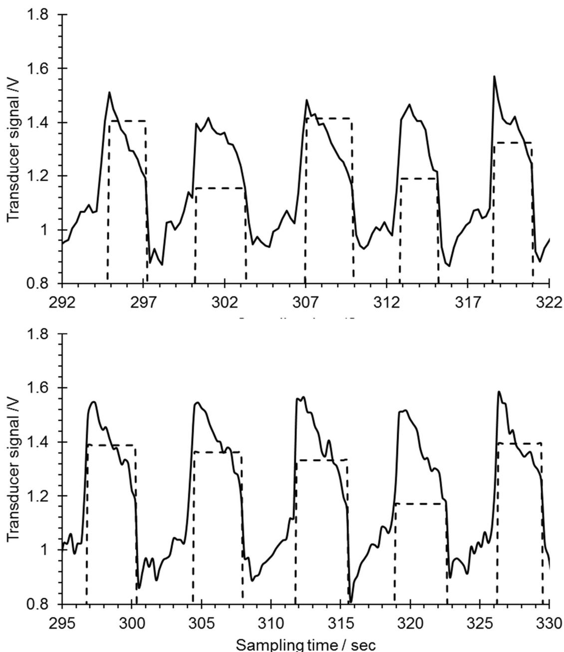
**Figure 4.5.4.2. An example of breath profile from a healthy participants collected from portable breath sampler (Top) and original adaptive breath sampler (Bottom)**
