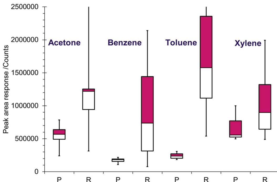
**Figure 4.5.2.1. Comparison of common air contaminants levels found in room air and purified air from the portable breath sampler. P denotes purified air supply and R denotes background room air.**
