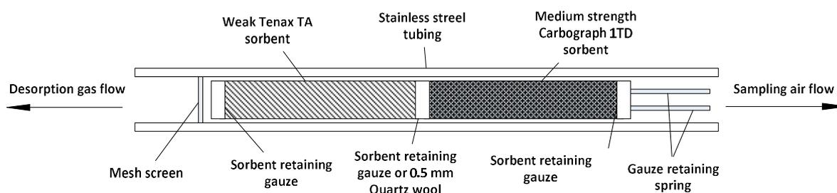
**Figure 1.6.4.2. Schematic diagram of multi-sorbent tube with weaker Tenax TA sorbent and medium strength Carbograph 1TD sorbent.**
