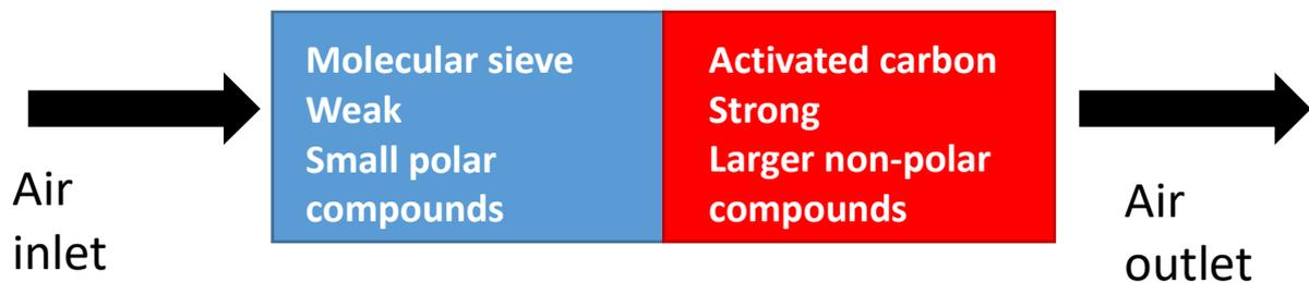
Figure 4.2.5.1. Combining molecular sieve and activated carbon
