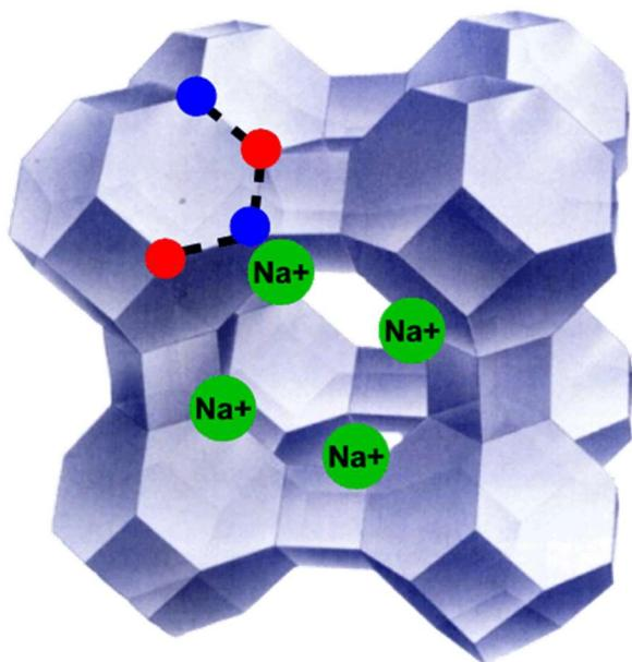
**Figure 4.2.2. Zeolite structure of molecular sieve 4A (76)**
