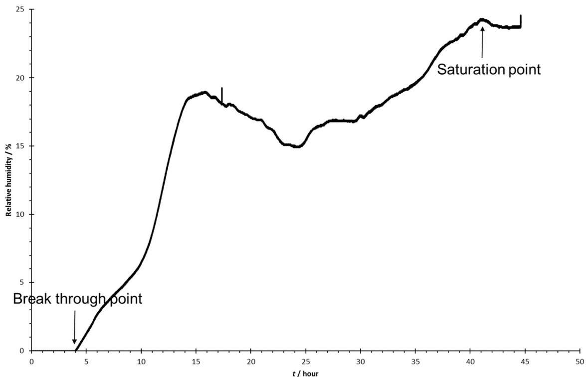
**Figure 4.5.1. Line plot of RH% against dehydration duration using molecular sieve 13X desiccant filter. Both break through point and saturation point are labelled on the graph**
