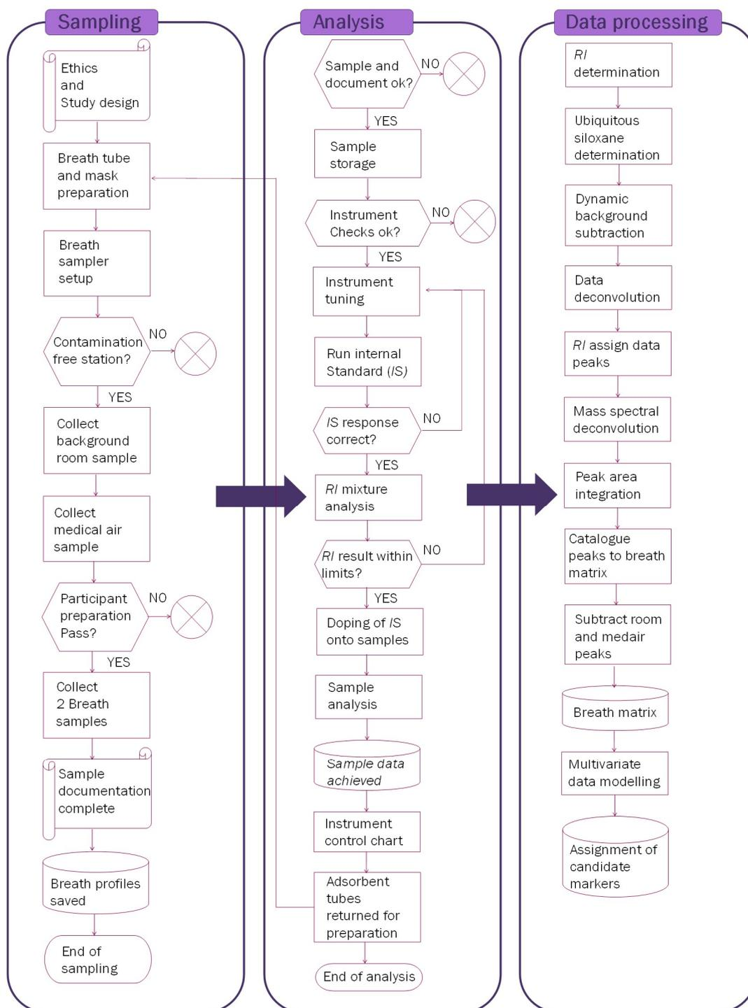
**Figure 2.1. The current exhaled breath VOCs analysis work-flow chart with 3 main stages: Exhaled breath sampling, breath sample analysis and data processing.**
