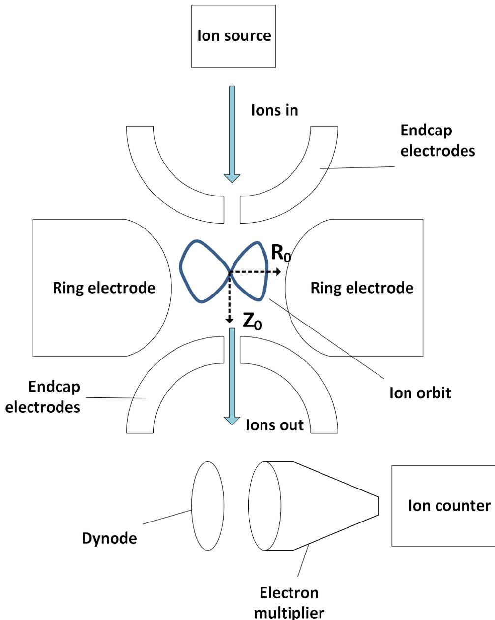
**Figure 1.6.4.3.1. Schematic diagram of quadrupole ion trap consisting of the central ring electrodes and two adjacent endcap electrodes. The ion trap is radially**
