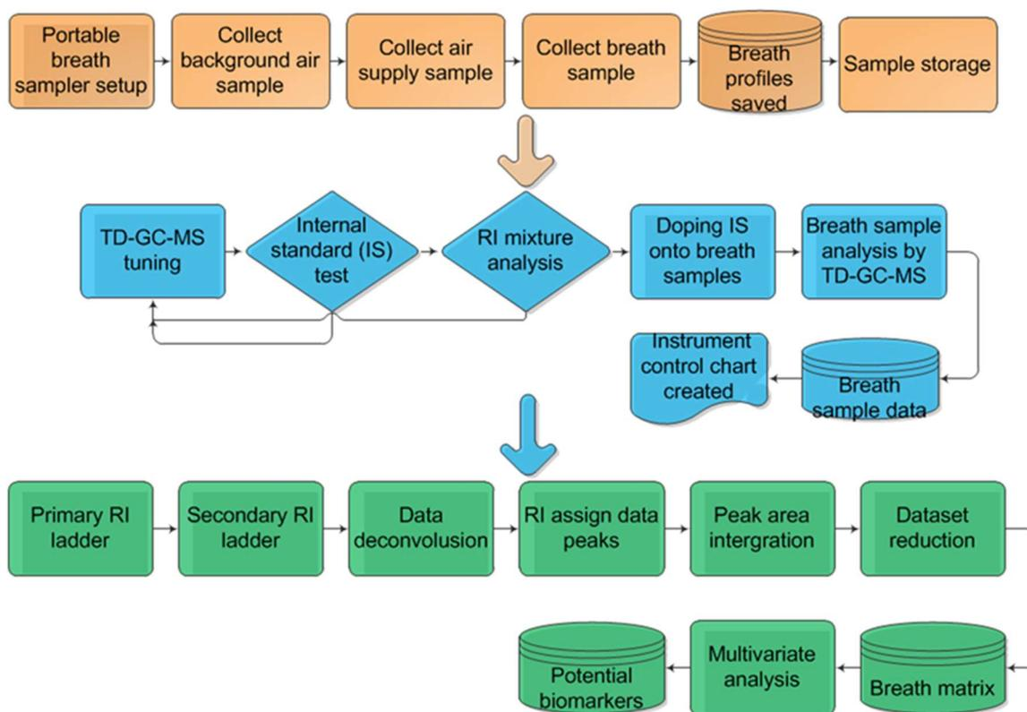
**Figure 5.4.2.1.1. Exhaled breath VOCs sampling work-flow using the portable breath sampler for EIB study**
