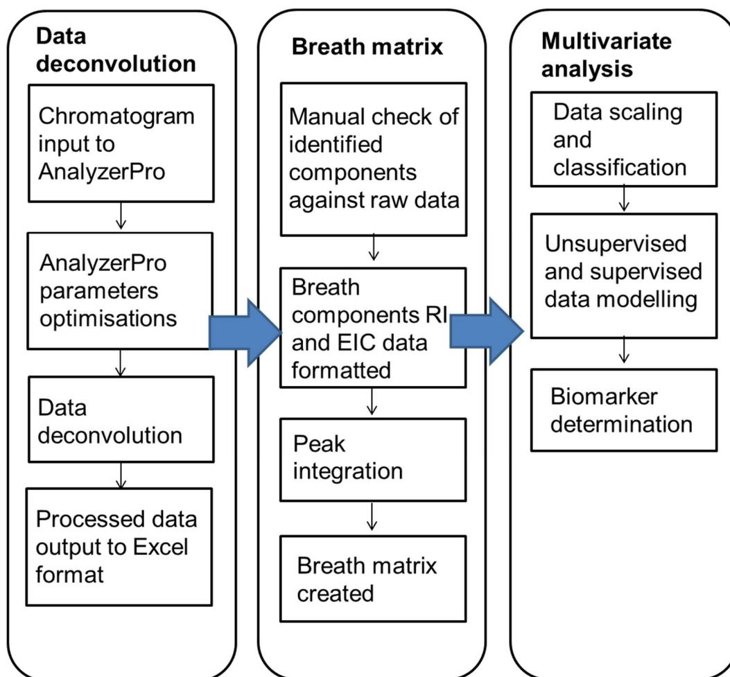
**Figure 2.4.1. The work-flow diagram of exhaled breath data processing method consisting of data deconvolution, creation of breath matrix and multivariate analysis.**
