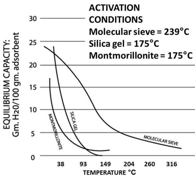
Figure 4.2.3.2.2. (top) Desiccant water capacity versus relative humidity based on air at atmospheric pressure and 25°C. (bottom) Desiccant water capacity versus temperature (77).
