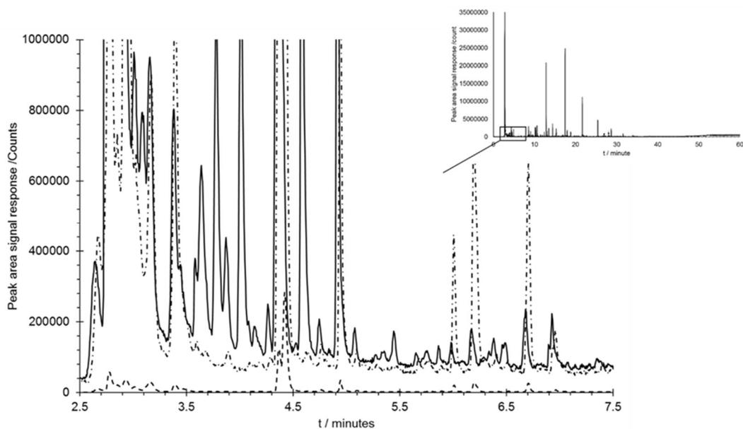
**Figure 5.4.2.1.2. TIC chromatogram of participant breath sample (bold line), purified air supply (dash line) and background room air (dash dot line) illustrating the comparison between endogenous and exogenous VOCs**
