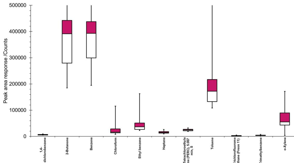
**Figure 4.5.5. The variability of 11 common room air contaminants found in breath sample using the portable breath sampler.**
