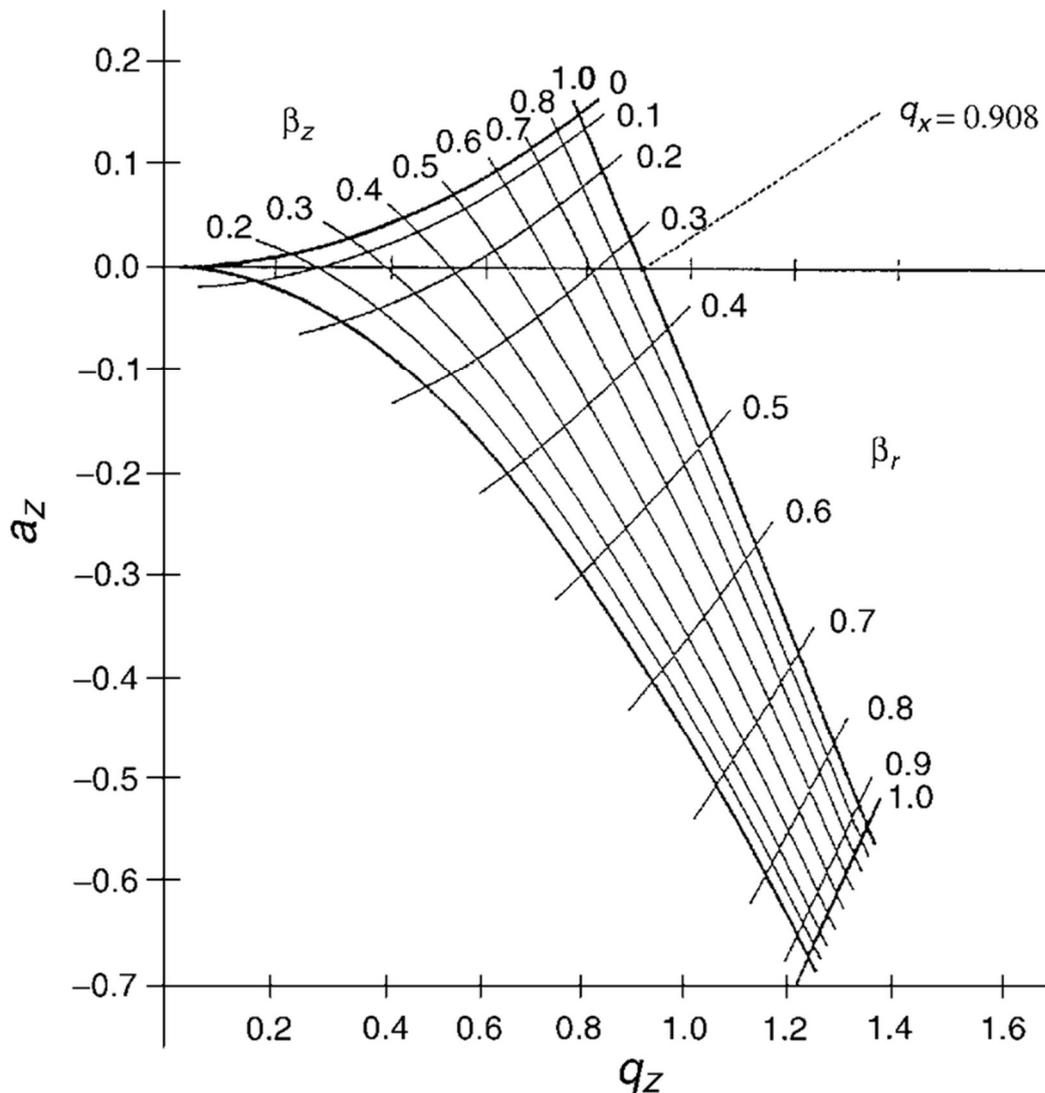
**Figure 1.6.4.3.2. The Mathieu stability diagram for quadrupole ion trap (58). Ion are simultaneous stable in both the R- and Z- planes if their  $a_z$  and  $q_z$  are within the**
