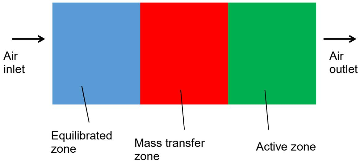
**Figure 4.2.3.1. Principle of desiccant water adsorption**
