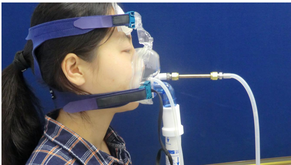
Figure 2-9 Photograph of the adaptive breath sampler in use.
