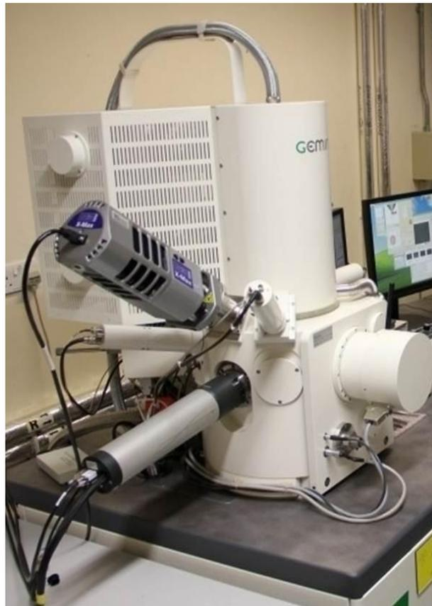
Figure 3-13. Leo 1530 VP FEG-SEM set-up.
