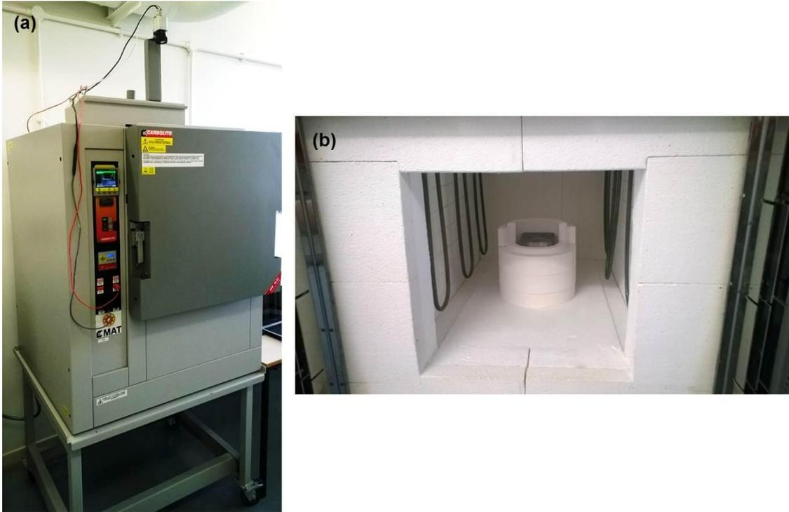
Figure 3-4. The images of (a) industrial MRF 16/22 microwave furnace with Micro-Epsilon/TIM 400 thermal imaging camera. (b) Microwave furnace chamber and the insulator blocks.
