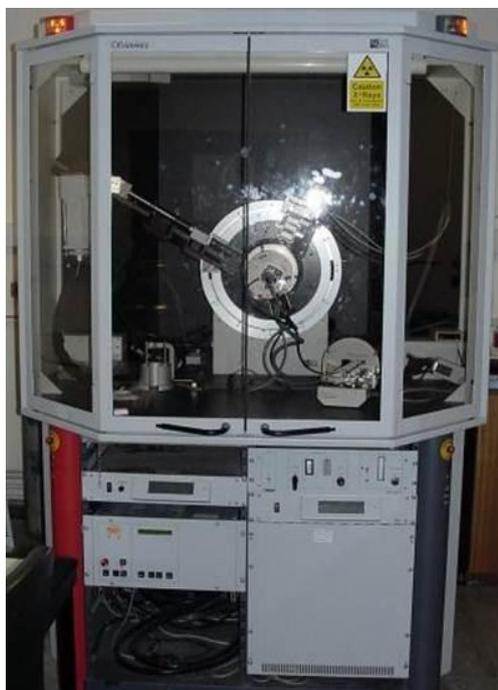
Figure 3-9. Photograph of the Bruker D8 X-ray diffractometer used in this study, the X-ray source is on the left, the sample is in the middle and the detector is on the right.
