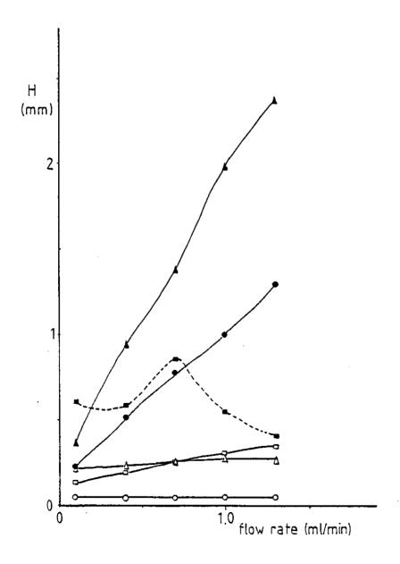
Dependence of plate height on eluent flow rate for PEG/PED standards on a polyether column packing. ethanol ( $\bigcirc$ ); PEG200 ( $\triangle$ ); PEG998 ( $\bigcirc$ ); PEG4820 ( $\bullet$ ); PEG9230 ( $\triangle$ ); PEG660000 ( $\bullet$ )
