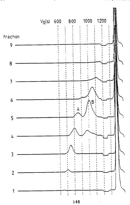
Chromatograms of the fractions of a mixture of PBMA (A) and PSS (B), concentrated from 8 injections, fraction collection times specified in table 2.3, eluent THF-HEP (36.2/63.8), at room temperature, PS-DVB packing, serial number 17-23, flow rate 0.5 cm<sup>3</sup> /min, instrument 2.
