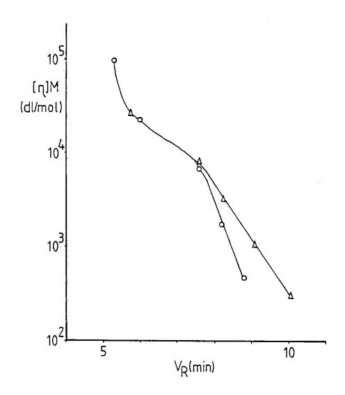
that the universal calibration is valid for [ $\Omega$ ]M above 9 \* 10 $^{\circ}$  dl mol<sup>-1</sup>.
