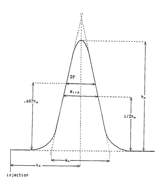
chromatographic peak (  $\P^2$ ) which is the fundamental parameter for evaluating column axial dispersion effects[86]. Assuming that the chromatogram has a Gaussian shape, as in figure 1.2, N and H are defined by:
