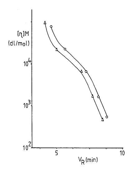
Hydrodynamic volume versus  $V_R$  calibration curves for PSA standards at room temperature, polyacrylamide column packing, serial number J56-3, flow rate 1 cm $^3$ /min, instrument 1. water ( O ); water-MeOH ( 80/20 ) (  $\Delta$  )
