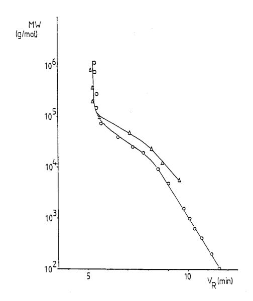
Log molecular weight versus  $V_m$  calibration curves for water-MeOH (80/20) mixture at room temperature, polyacrylamide column packing, serial number J56-3, flow rate 1 cm<sup>2</sup>/min, instrument 1. PEG, PEO (O); PSA ( $\Delta$ )
