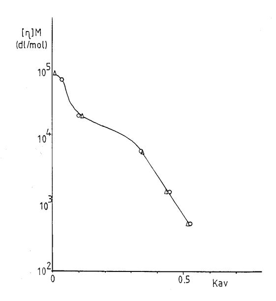
Hydrodynamic volume versus  $K_{av}$  calibration curves for PSA standards at room temperature, polyacrylamide column packing, serial number J56-3, flow rate 1 cm $^3$ /min, instrument 1. water ( O ); water-MeOH ( 80/20 ) (  $\Delta$  )
