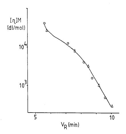
Hydrodynamic volume versus K.v calibration curves for PEG/PEO standards at room temperature, polyacrylamide column packing, serial number J56-3, flow rate 1 cm $^{3}$ /min, instrument 1. water ( O ); water-MeOH ( 80/20 ) (  $\Delta$  )
