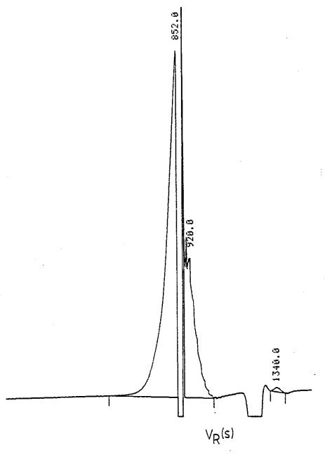
Chromatogram of PBMA ( 0.4% ) in THF with a PS-DVB column packing, serial number 17-21, instrument 3, showing the disturbance in flow rate caused by turning the switching valve to inject position.
