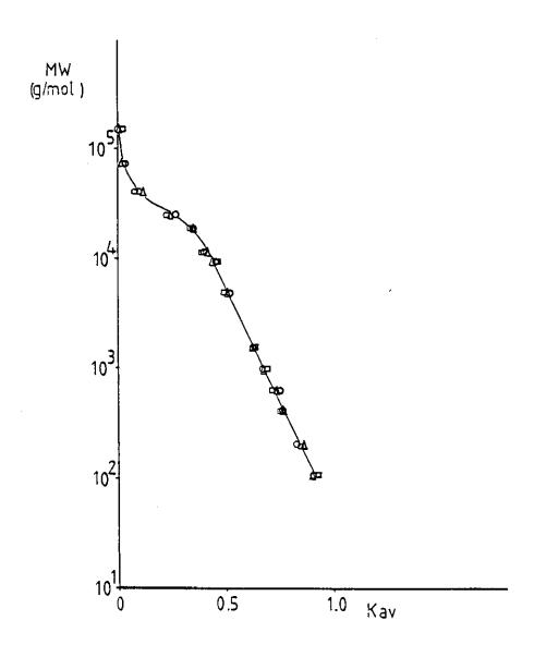
Log MW versus  $K_{av}$  calibration curve for PSA standards at room temperature, polyacrylamide column packing, serial number J56-3, flow rate 1 cm $^{\circ}$ /min, instrument 1. water (O); water-MeOH (80/20) ( $\Delta$ )
