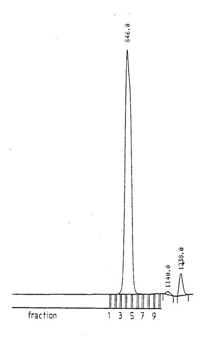
Chromatograms of the fractions of the standard PS32500 (specified in figure 3.30 ) in THF, at room temperature, column packing PS-DVB, serial number 17-21, flow rate 0.5 cm $^{\circ}$ /min, instrument 2
