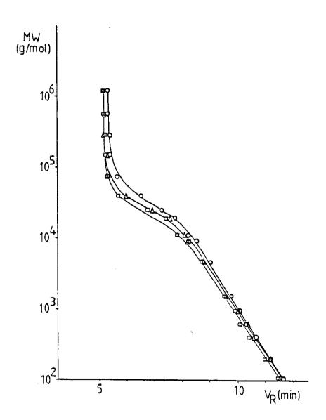
Log molecular weight versus  $V_R$  calibration curves for PSA standards at room temperature, polyacrylamide column packing, serial number J56-3, flow rate 1 cm $^{\circ}/min$ , instrument 1. water ( $\circ$ ); water-MeOH ( $\circ$ 80/20) ( $\circ$ 4).
