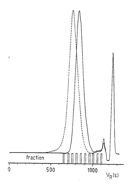
Chromatogram of a mixture of PSS and PBMA ( 0.3% each ) in THF, at room temperature, column packing PS-DVB, serial number 17-21, flow rate 0.5 cm<sup>3</sup>/min, instrument 2, showing the  $V_{\pi}$  for fraction collection.
