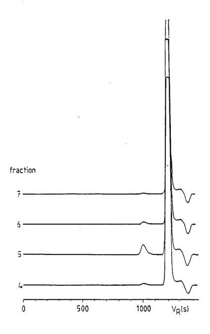
Chromatogram of PSS (---) and PBMA (----) in THF, at room temperature, column packing PS-DVB, serial number 17-21, flow rate 0.5 cm $^{\circ}$ /min, instrument 2, showing the  $V_{\pi}$  used for fraction collection in figure 3.33.
