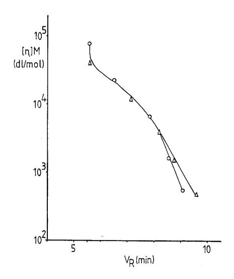
Hydrodynamic volume calibration curves with water-MeOH ( 80/20 ) mixture as eluent at room temperature, polyacrylamide column packing, serial number J56-3, flow rate 1 cm<sup>-3</sup>/min, instrument 1. PEG/PEO ( O ); PSA (  $\Delta$  ).
