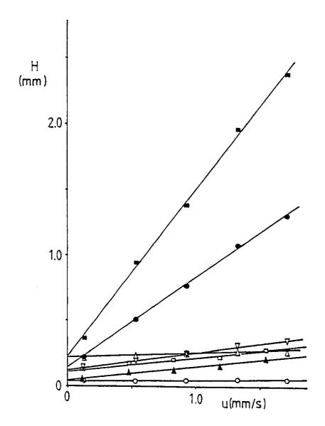
Dependence of experimental plate height on eluent flow velocity for polyether column packing, in water, instrument 1, Ethanol ( $\bigcirc$ ); PEG200 ( $\triangle$ ); PEG998 ( $\bigcirc$ ); PEG 4820 ( $\bigcirc$ ); PEG9230 ( $\bigcirc$ )
