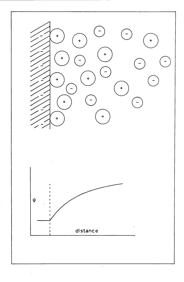
Fig. 3 The STERN Model for the Double Layer
