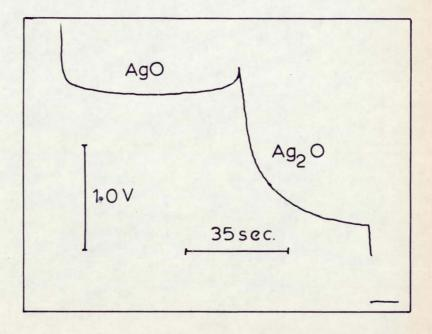
Fig. 19 P.S.V. Current-Potential Trace for Silver in 1.OM NaOH, 23°C, 6 x 10<sup>-4</sup> V sec<sup>-1</sup> (Trace runs from R - L) Start at + 0.338V. A- Preliminary Reaction Peak; B-Massive Ag<sub>2</sub>O Formation; C- Massive AgO Formation.
