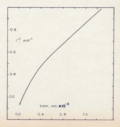
Fig. 26 Typical Tafel Plot for the Formation of Ag<sub>2</sub>0 in 1.0M NaOH at 23°C. Comparison of Potentiostatic and Galvanostatic Technique.
