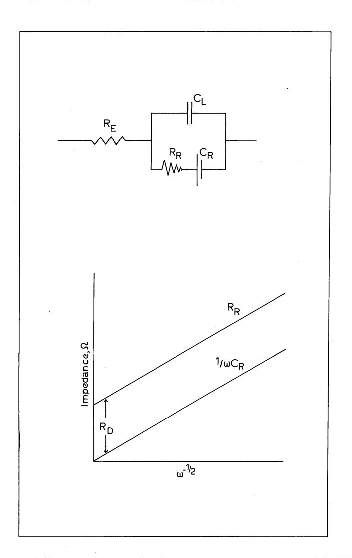
bridge measurements correspond to C<sub>L</sub>, the electrode capacitance (Ch. 2), and R<sub>E</sub>, the electrolyte resistance (130). Very accurate electrode capacitance measurements are possible using this technique (75), and the potential is continuously variable enabling accurate differential capacitance curves to be derived and, as a consequence, valid data concerning the structure of the double layer may be deduced.
