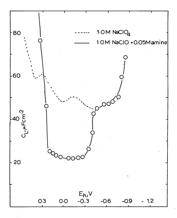
Fig. 17 The Effect of n-Butylamine on the Differential Capacitance of Silver in 1.0M NaOH, 23°C, 1000c/sec.
