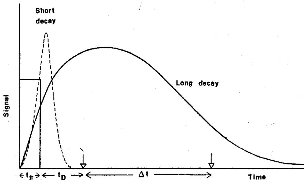
Fig 1.2 Diagram of time resolved fluorescence measurements
