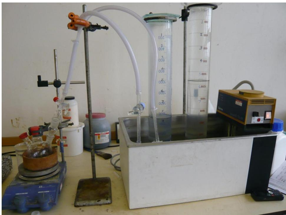
**Figure 3-24** – *Equipment used for measuring catalase activity*
