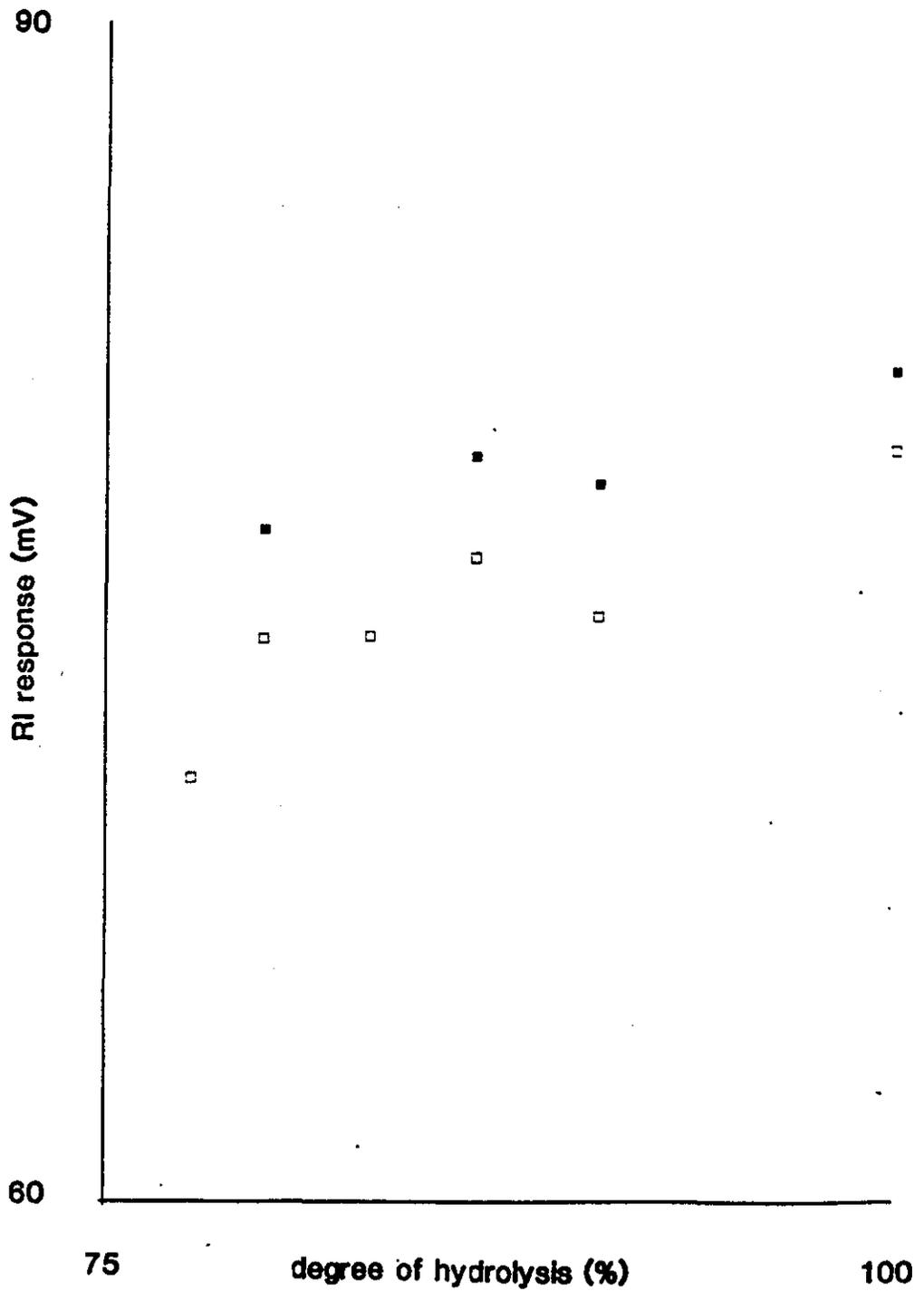
FIGURE 12 RI response as a function of degree of hydrolysis for PVOH samples dissolved in (□) 0.05M NaNO<sub>3</sub> and (■) 0.1% (w/v) Aerosol IB45.
