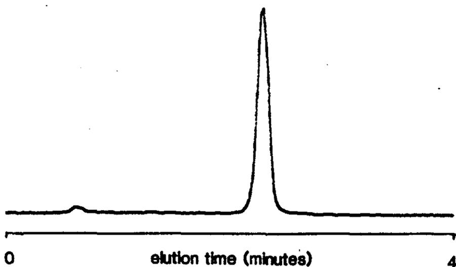
1 x PLRP-S  $8\mu\text{m}$   $4000\text{\AA}$  column and mass detector
