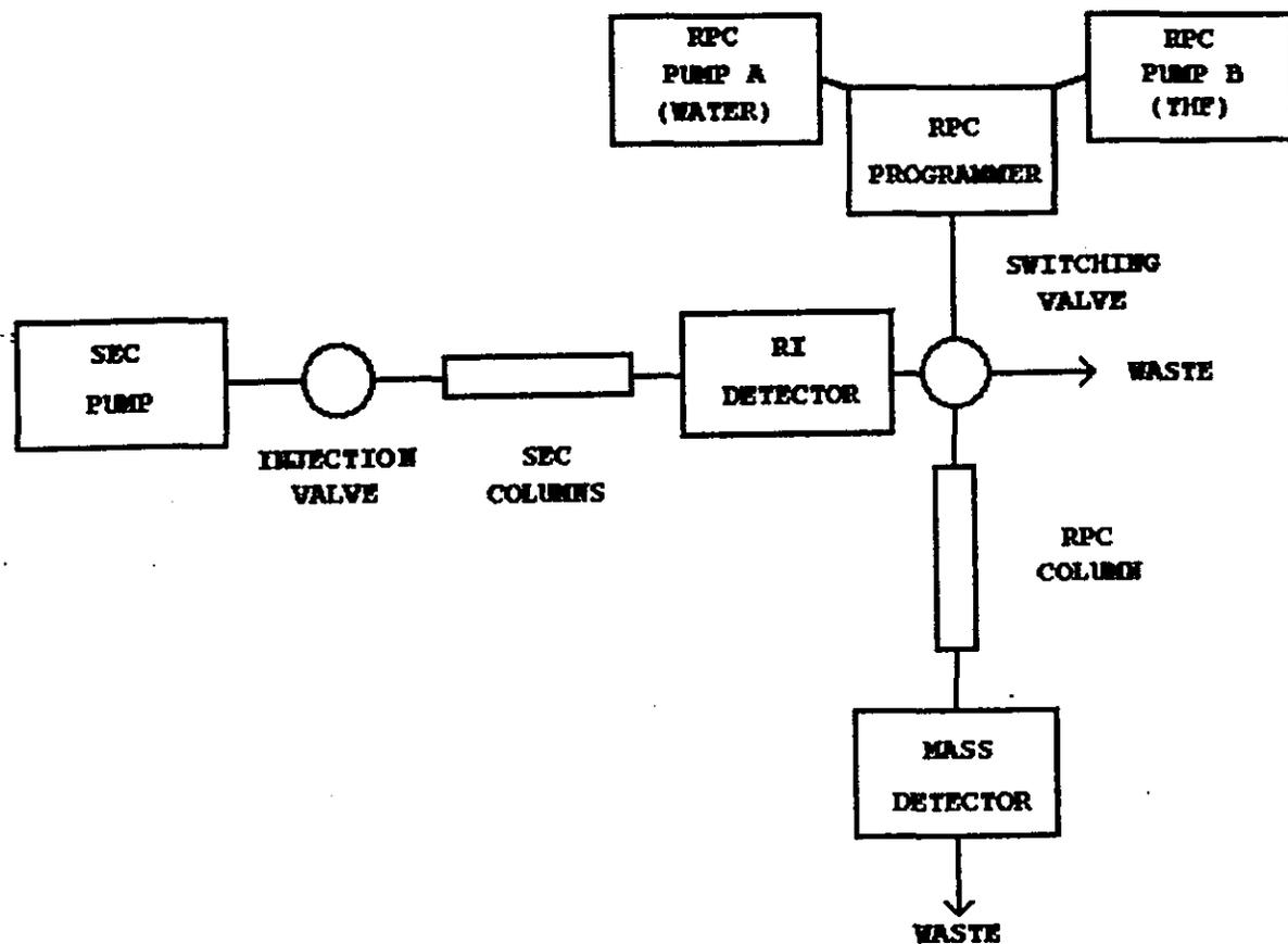
**FIGURE 2** Proposed CCC system with SEC preceding RPC
