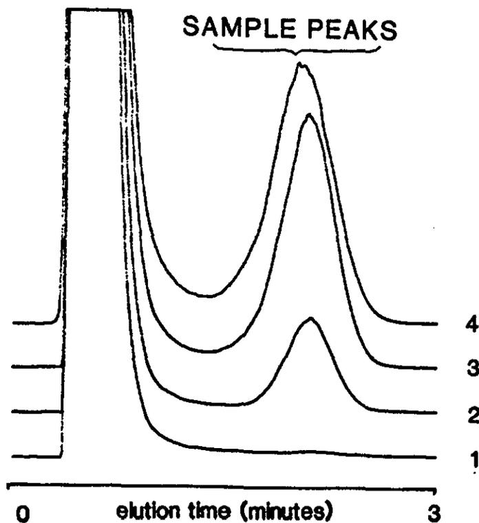
FIGURE 29 CCC chromatograms for a 73.7% hydrolysed PVOH sample (continuous mode): (a) SEC chromatogram from which fractions 1-4 were collected, with 0.25% (w/v) as eluent; (b) RPC chromatograms of fractions 1-4 with gradient elution from 65/35 (held for 0.5 minutes) to 30/70 water/THF (v/v) in 1.5 minutes.
