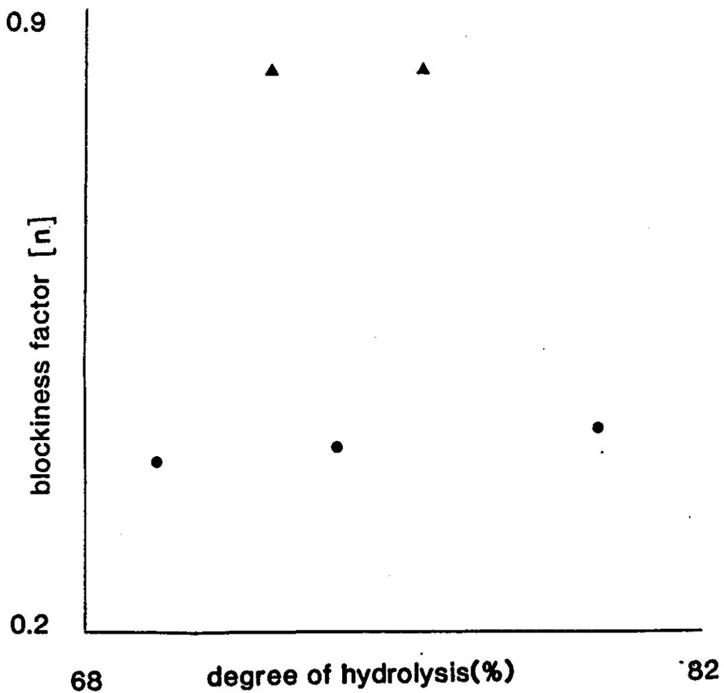
FIGURE 19 Blockiness factor as a function of degree of hydrolysis for (●) alkaline and (▲) acid hydrolysed PVOH samples calculated from NMR spectra.
