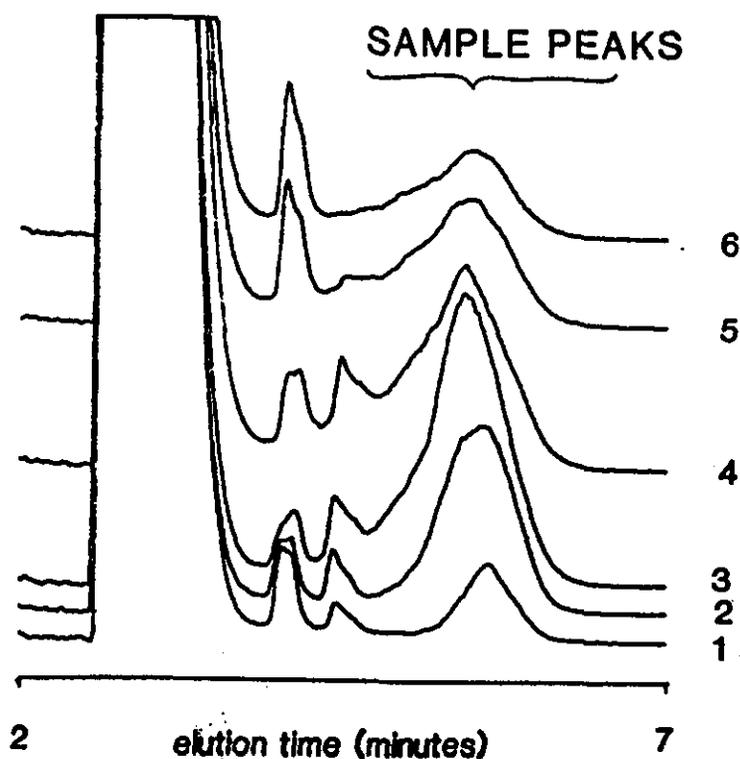
FIGURE 28 CCC chromatograms for a 73.7% hydrolysed PVOH sample (discontinuous mode): (a) typical SEC chromatogram from which fractions 1-6 were collected, with 0.25%(w/v) SLS as eluent; (b) RPC chromatograms of fractions 1-6 with gradient elution from 99/1 to 1/99 water/THF (v/v) in 10 minutes.
