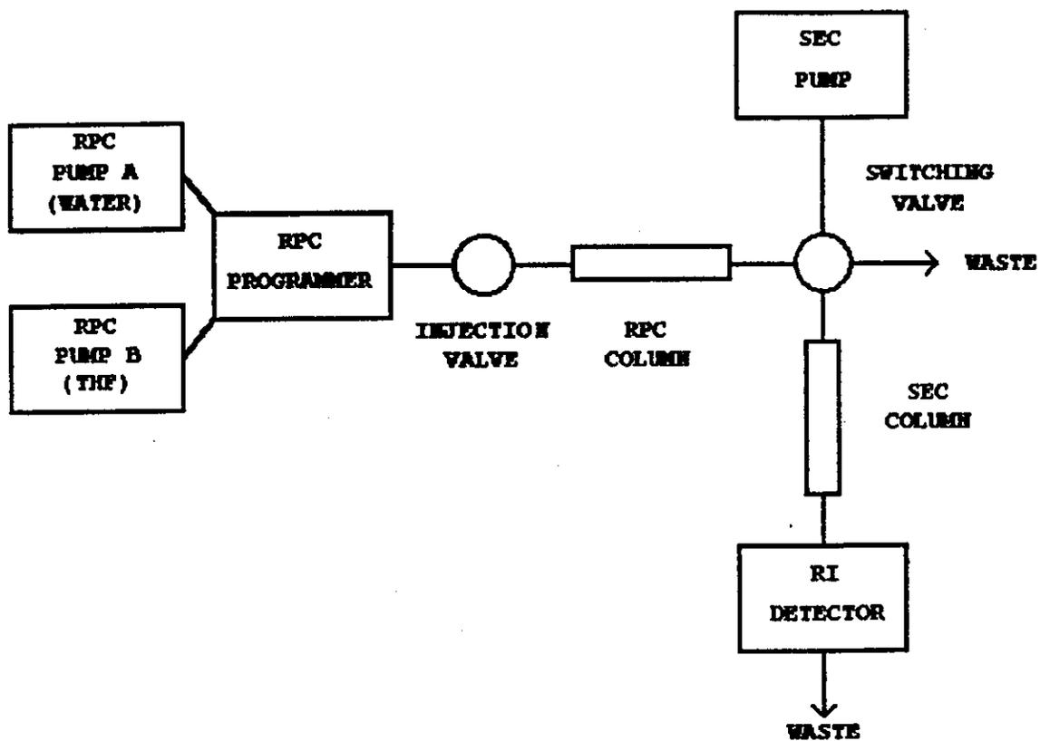
**FIGURE 1** Proposed CCC system with RPC preceding SEC
