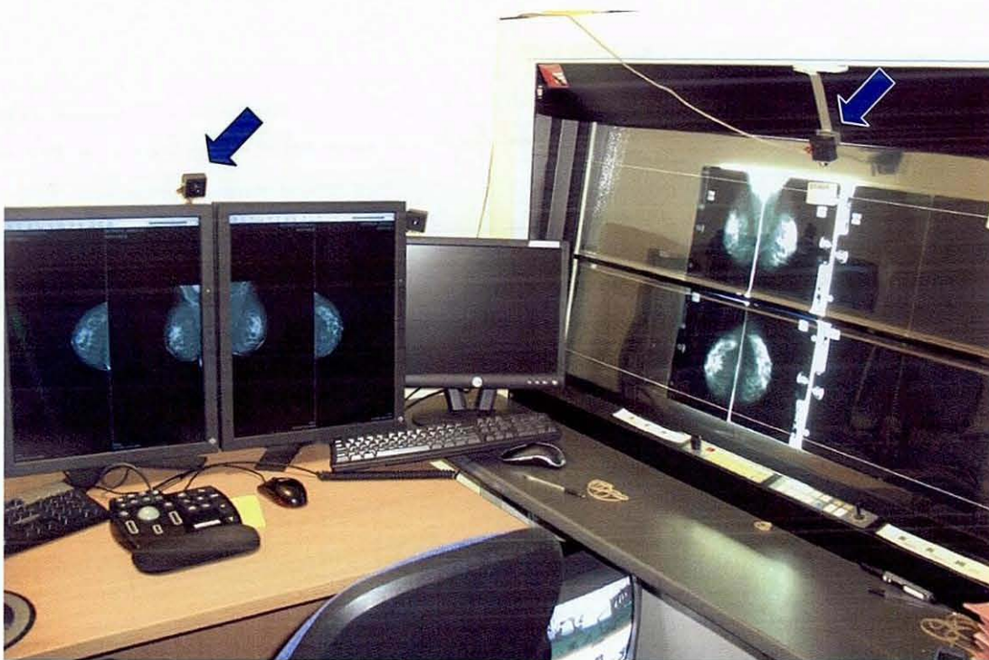
Figure 4.2 – The hybrid workstation with miniature video cameras highlighted by the blue arrows, and video recording display below the workstation.
