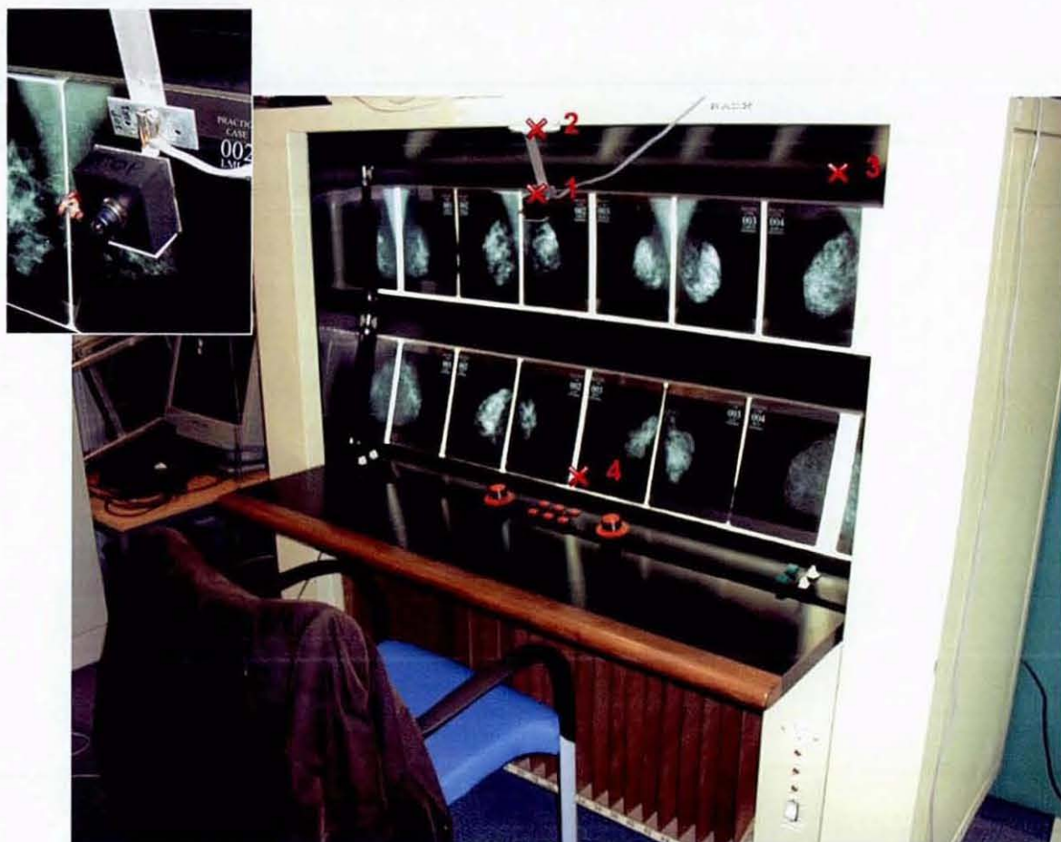
Figure 4.1 – Experimental set up for camera placement trials. Numbers 1 to 4 indicate the four camera placements trialled. The inset shows the camera used.
