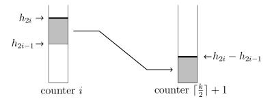
Counters i and  $\lceil \frac{k}{2} \rceil + 1$  are then set back to 0 by incrementing them once more. Then they are incremented simultaneously until counter  $\lceil \frac{k}{2} \rceil + 1$  reaches its counter bound. After this step, counter i stores value  $h_{2i} - h_{2i-1}$  as pointed out by the following illustration.
