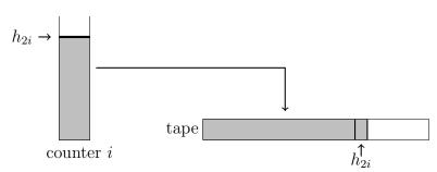
As counter  $\lceil \frac{k}{2} \rceil + 1$  has a counter bound of  $h_{2i-1}$ , we can easily set the value of counter *i* back to  $h_{2i-1}$ . Finally, the input head is moved back to position 0 and the value of counter  $\lceil \frac{k}{2} \rceil + 1$  is set back to 0.
