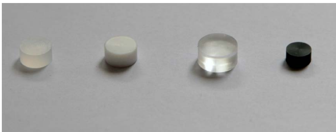
Figure 3.2 Untested cylindrical polymer specimens that have been prepared for high strain rate experiments using the SHPB technique. From left to right the specimen materials are PCTFE, PTFE, PMMA, and PVC.
