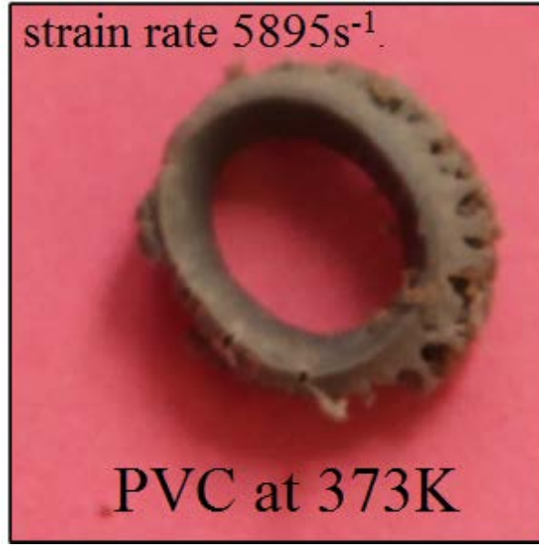
Figure 6.7 The deformed PVC sample after testing in the split Hopkinson bar at a strain rate of 5895 \text{ s}^{-1} and with the sample preheated to 373 K. The image is also repeated from that of Figure 5.24(i).
