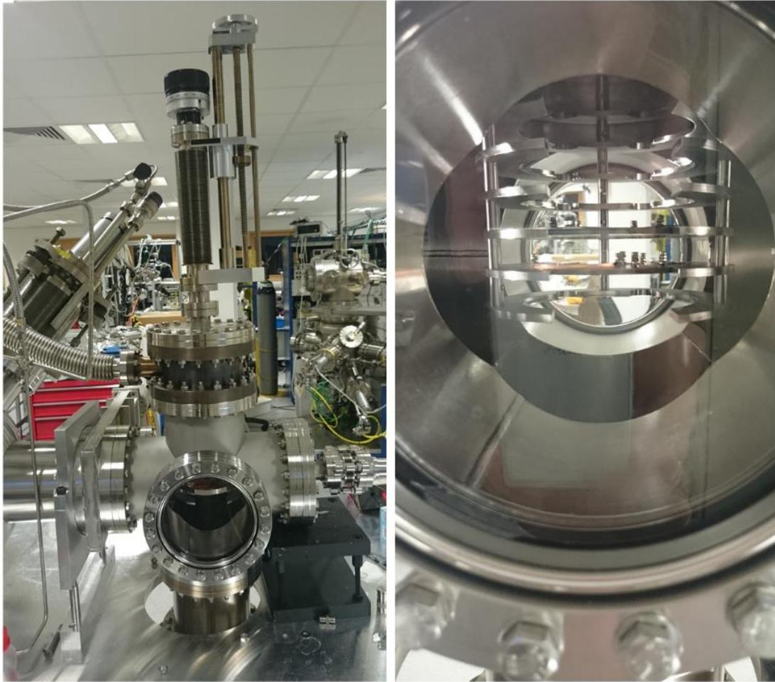
Figure 6.4. The entire load lock chamber is shown in the left hand image and the 7 sample cartridge system is shown in the right image.
