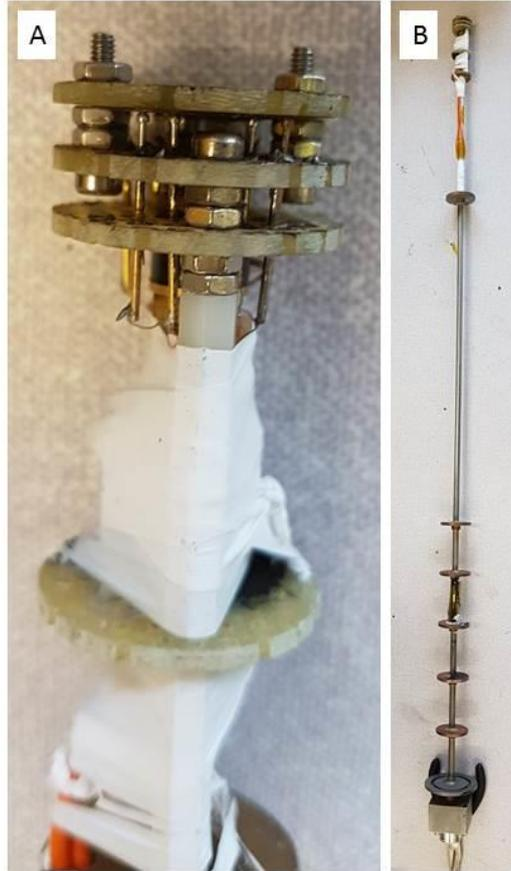
Figure 6.9. Photographs of a) the four-point probe and b) the sample stick (insert).
