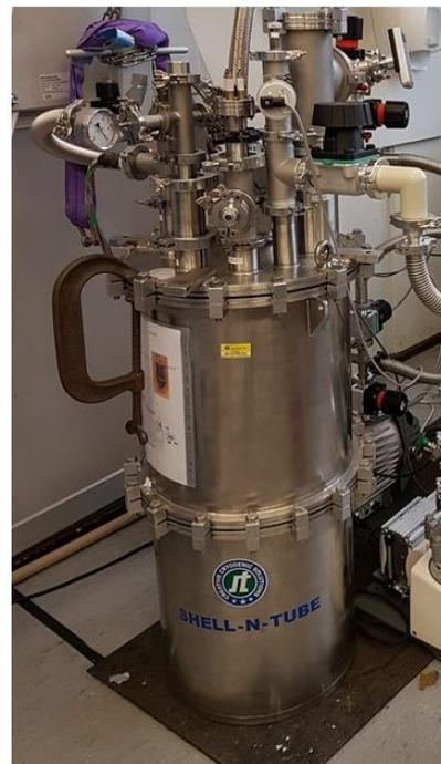
**Figure 6.7.** The left hand image shows a schematic drawing of the cryostat which houses the four-point probe and the right hand image shows a photograph of the cryostat.
