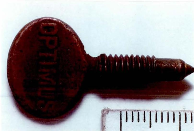
**Photo 3.2.3d:** The needle valve after laser treatment at a fluence of  $2\text{J}/\text{cm}^2$ . Note how the laser has penetrated into the thread and clarified the embossed writing.
