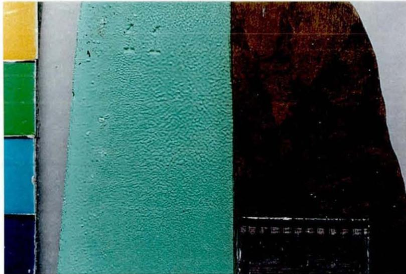
**Photo 3.1.7a:** *Case 6a.* The right-hand side of the coupon was subject to 7-8 laser pulses at  $2\text{J}/\text{cm}^2$ . The grain structure of the metal is visible under a thin, brown oxide layer.
