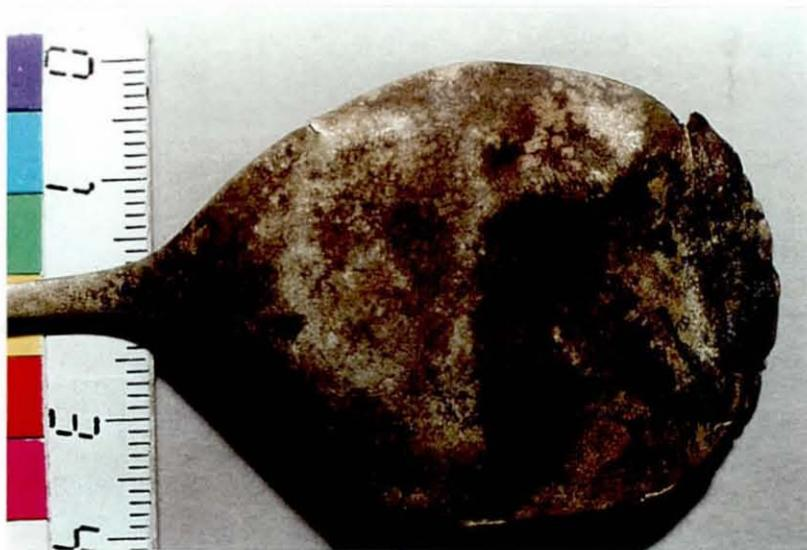
Photo 3.2.7b: The corrosion was removed from the spoon after just a couple of pulses at  $2\text{J}/\text{cm}^2$ . The source of the discoloration was not identified.
