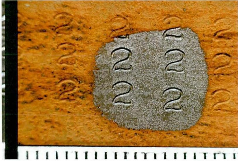
**Photo 3.1.10a:** *Case 9a.* The mild steel surface has been exposed after 2-3 laser pulses at  $2\text{J}/\text{cm}^2$ .
