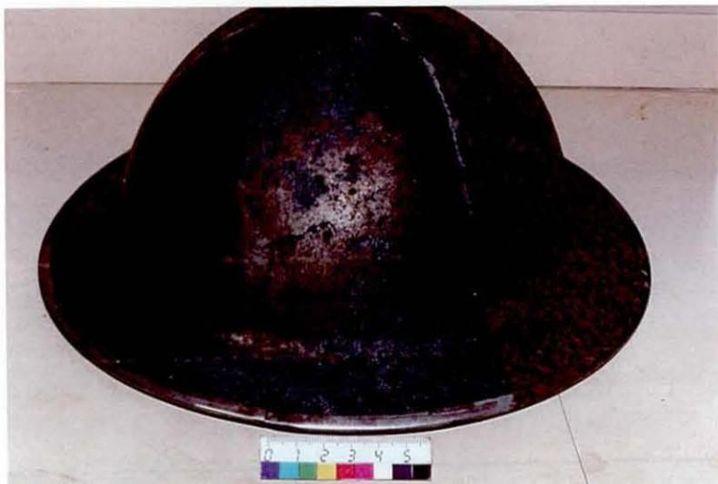
**Photo 3.2.5a:** *Case 5n*. The untreated, rusted surface is shown on the right, the laser treated surface in the middle, and the laser treated surface after a beeswax coating has been applied, on the left.
