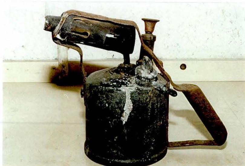
**Photo 3.2.3a:** Naturally corroded blowtorch of *Case 3n*, as received.
