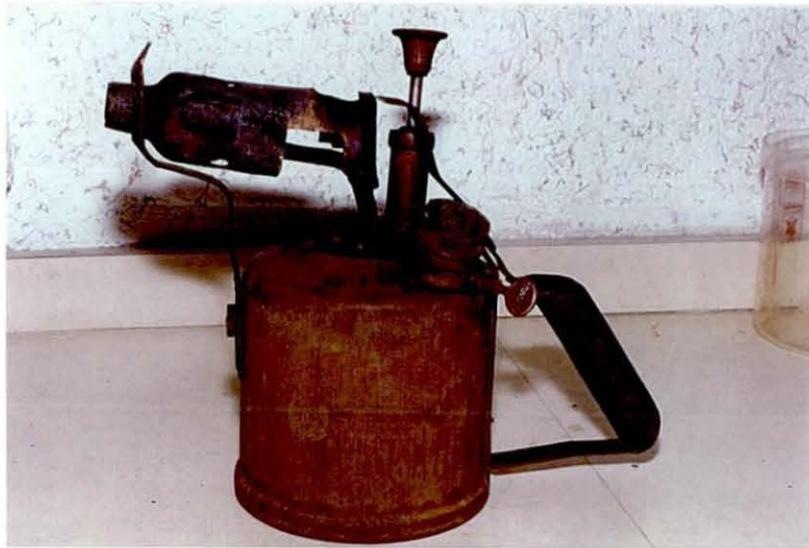
**Photo 3.2.3b:** The blowtorch after laser treatment at a fluence of  $2\text{J}/\text{cm}^2$ . Part of the steel bracket and head-piece have been removed for surface analysis.
