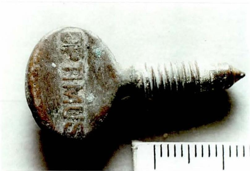
**Photo 3.2.3c:** The untreated needle valve from the blowtorch in *Case 3n*.
