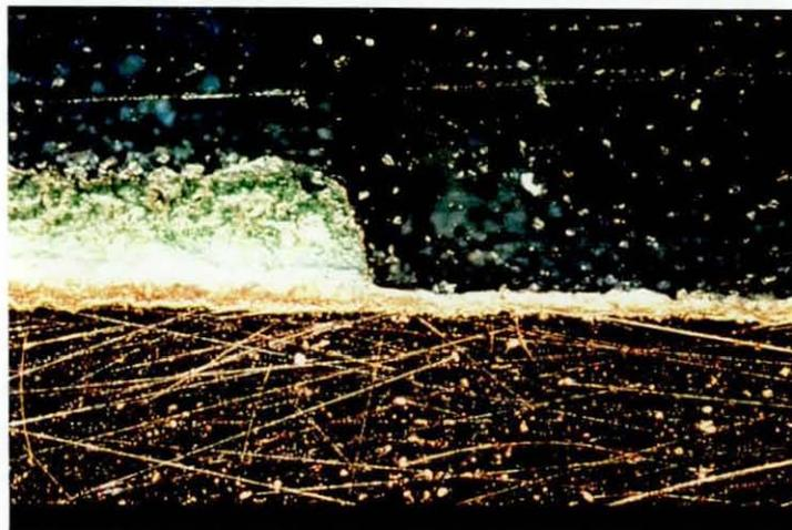
**Photo 3.1.4c:** Cross-section through the copper coupon from *Case 3a*. The left-hand side shows the untreated corrosion layers, the right-hand side the laser treated area. The red interfacial layer is clearly visible on both sides and represents the limit of the cleaning process.
