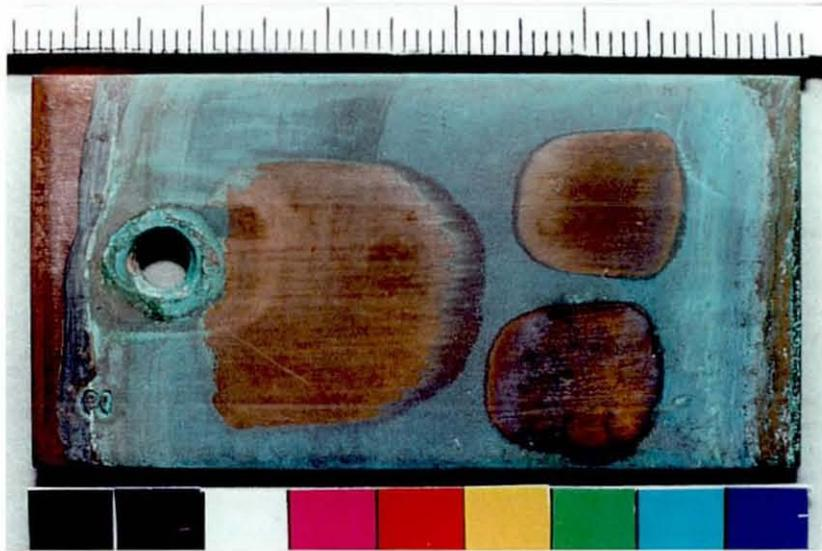
**Photo 3.1.2a:** *Case 1a*. The surface shows the results of three laser treatment tests; on the left, 2 pulses at  $0.5\text{J}/\text{cm}^2$ ; at the top right, 2 pulses at  $2\text{J}/\text{cm}^2$ ; at the bottom right, 10 pulses at  $2\text{J}/\text{cm}^2$ .
