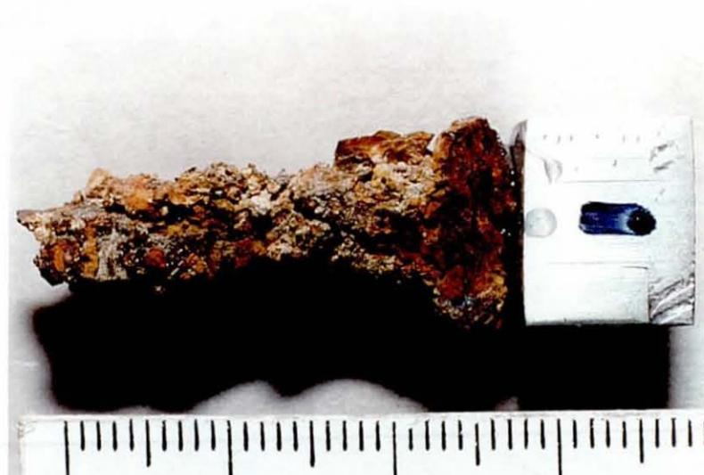
**Photo 3.2.6a:** The rusted nail from *Case 6n*. The shape of the original surface is completely obscured by corrosion products.
