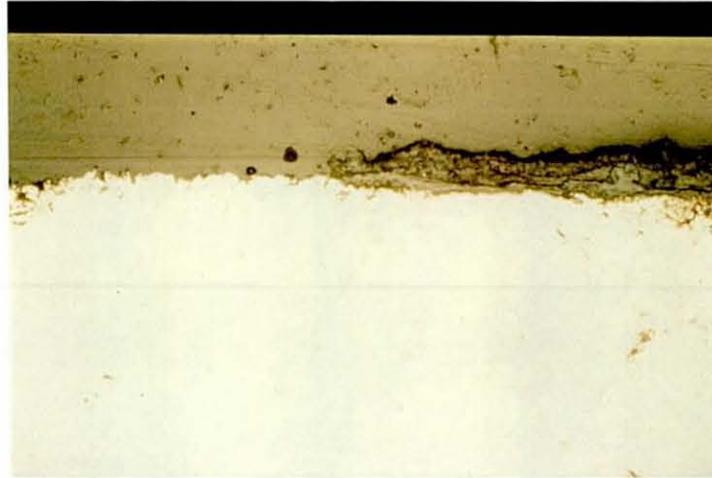
**Photo 3.2.3i:** A cross-section through the blowtorch body in *Case 3n*. The right-hand side is untreated and the left-hand side has been laser treated. There is no evidence of a remaining corrosion layer on the laser-treated side, and the metal surface has retained its roughness with no evidence of melting.
