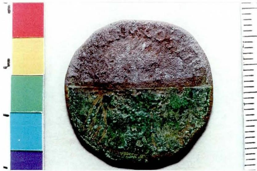
**Photo 3.2.2a:** *Case 2n*. The top half of the coin has been subjected to 20-30 laser pulses at  $2\text{J}/\text{cm}^2$ . There has been some loss of detail due to the laser.
