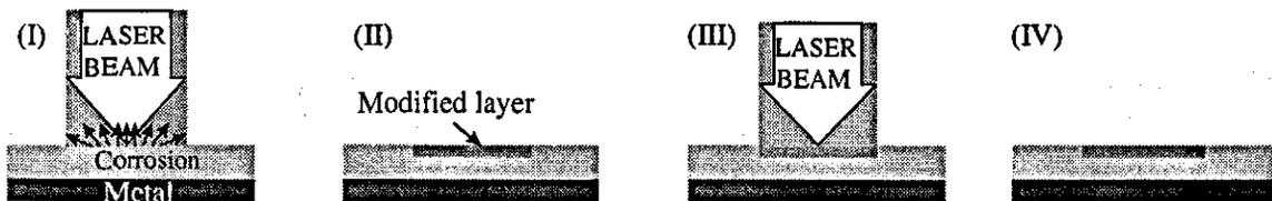
**Fig 3.2.9c:** Laser modification of surface corrosion products without causing significant ablation.
