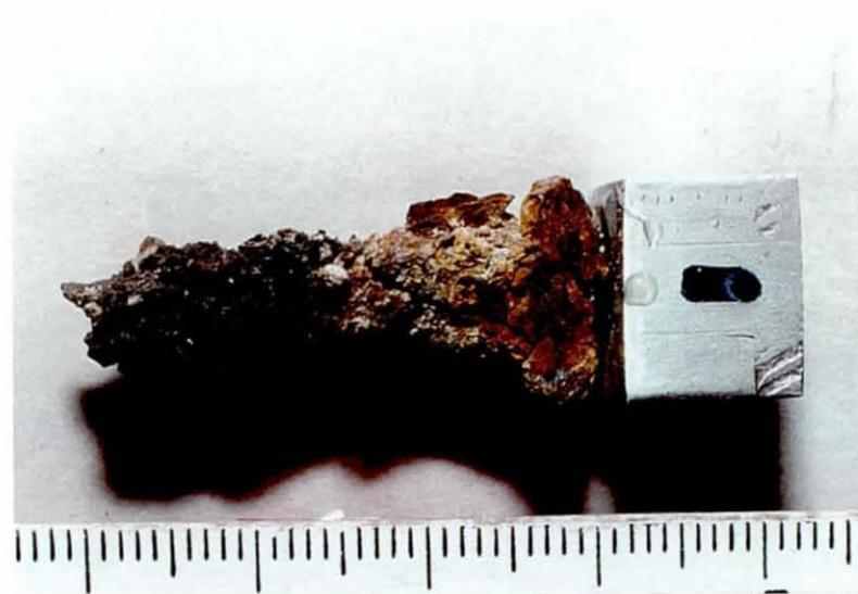
**Photo 3.2.6b:** Laser treatment of the nail at a fluence of  $2\text{J}/\text{cm}^2$  caused blackening of the corrosion products.
