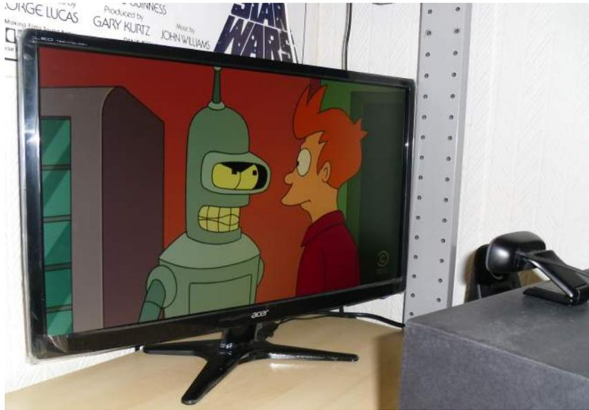
Figure 3.1: The web-camera is positioned in front of a LCD monitor. This allows us to select stimuli such as television shows that have a wide colour contrast. This static set-up allows us to optimize the position of the camera to obtain the strongest possible relation between a known colour and the colour identified by the camera (see subsection 3.2.1). This is achieved by manipulating lighting conditions and adjusting the distance between the camera and the screen.
