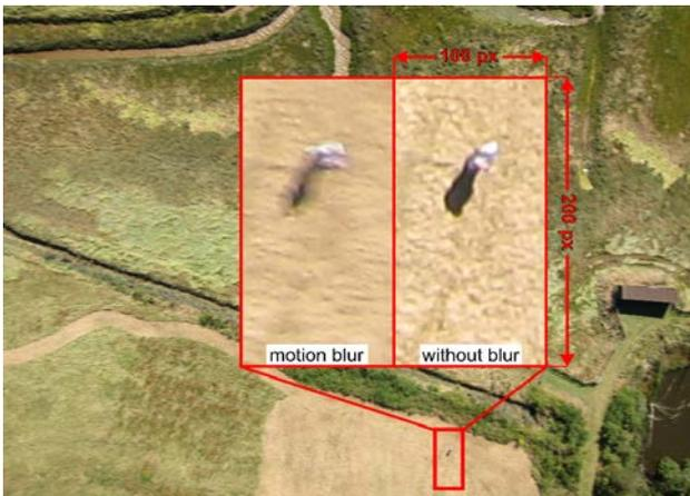
Figure 2. Motion blur example in high resolution UAV image.
