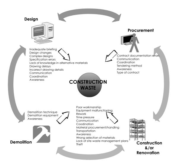
Figure 1: Lifecycle construction waste mapping (compiled from literature)
