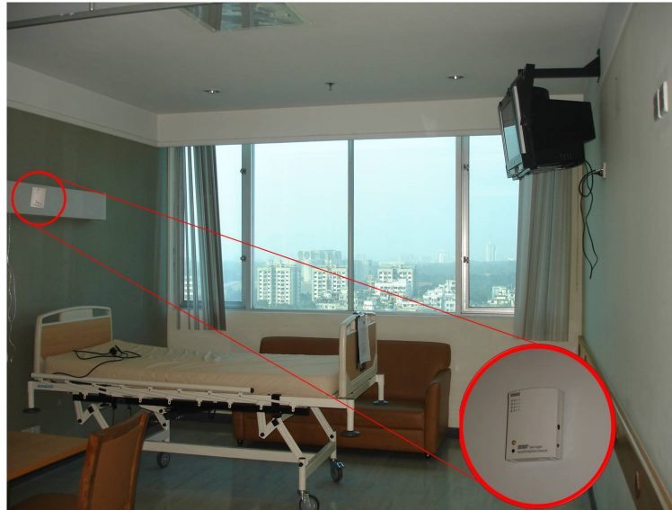
Figure 3: Location of indoor data logger(source: Joarder et al., 2010).
