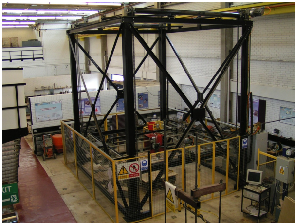
Figure 1: The printing frame of Concrete Printing.
